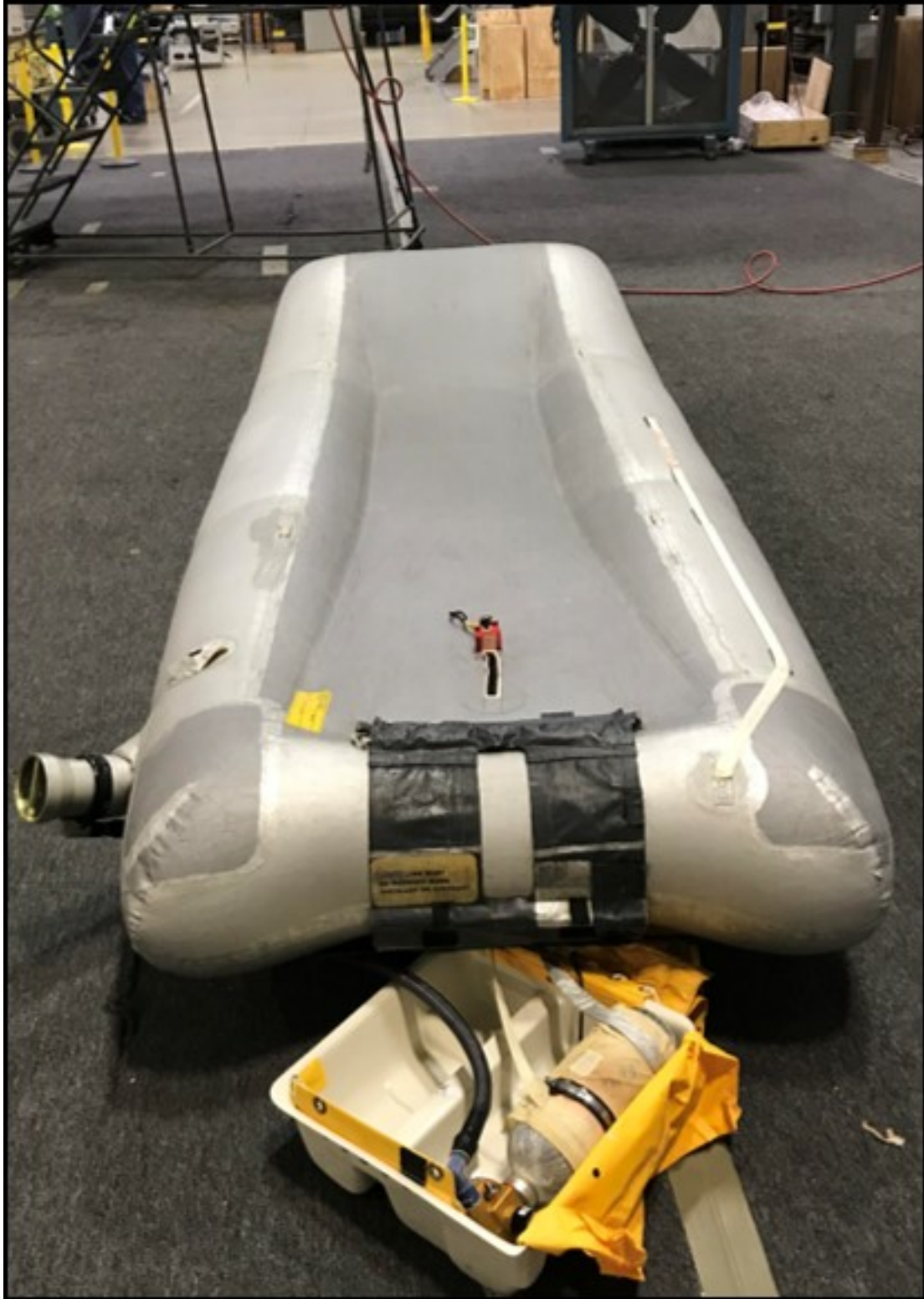
Photograph 4 – Successful floor run slide inflation.
