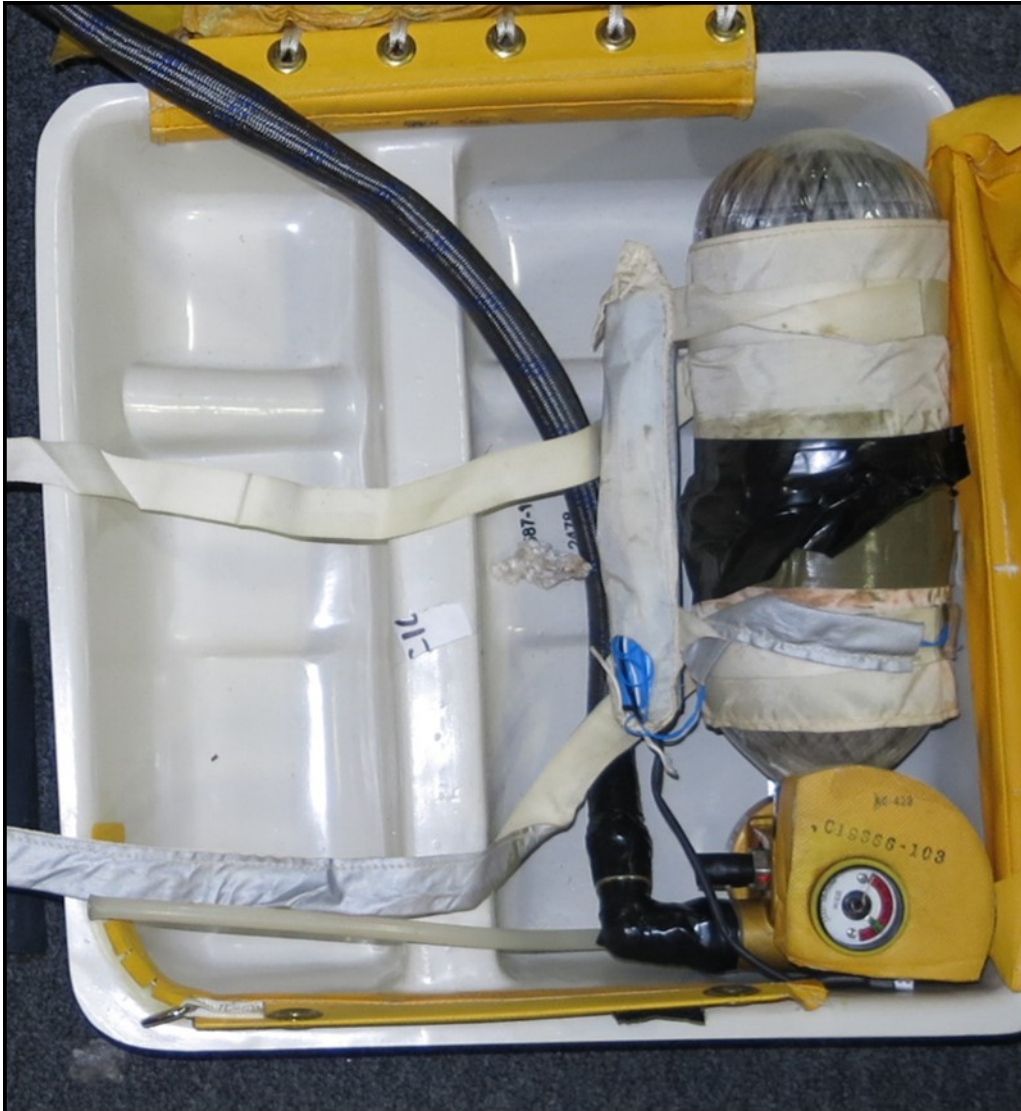
Photograph 2 – Reservoir and valve assembly (RVA) in packboard.
