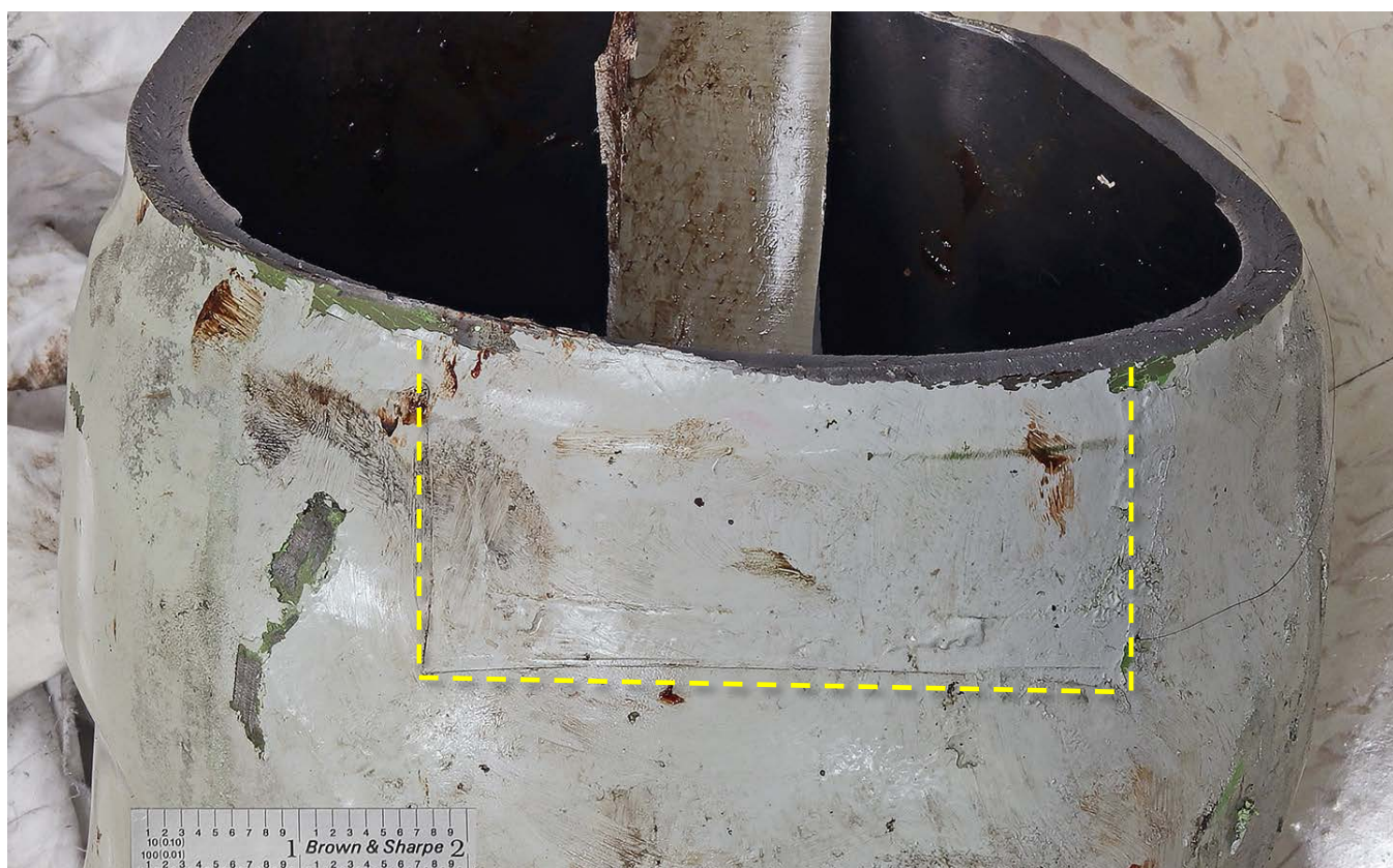
Figure 5 – View of the upper fracture surface, viewed from the forward side. The boxed area highlights the masked and repainted area.
