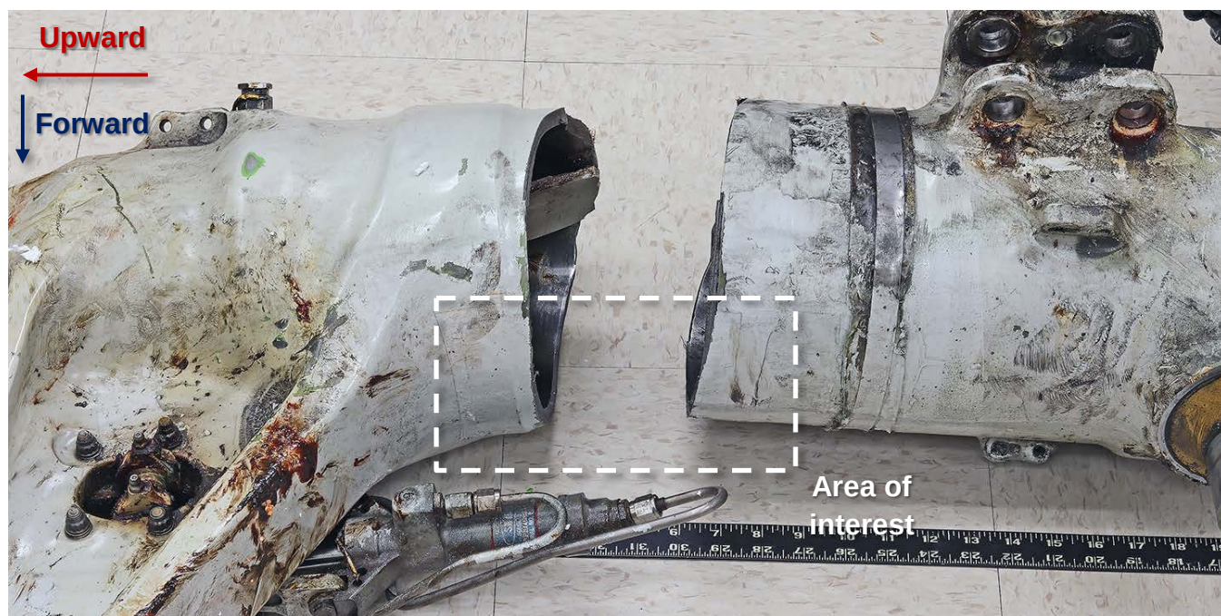
Figure 4 – Closer view of the forward side of the fractured landing gear, showing the area of fracture initiation on the forward side (white boxed area).
