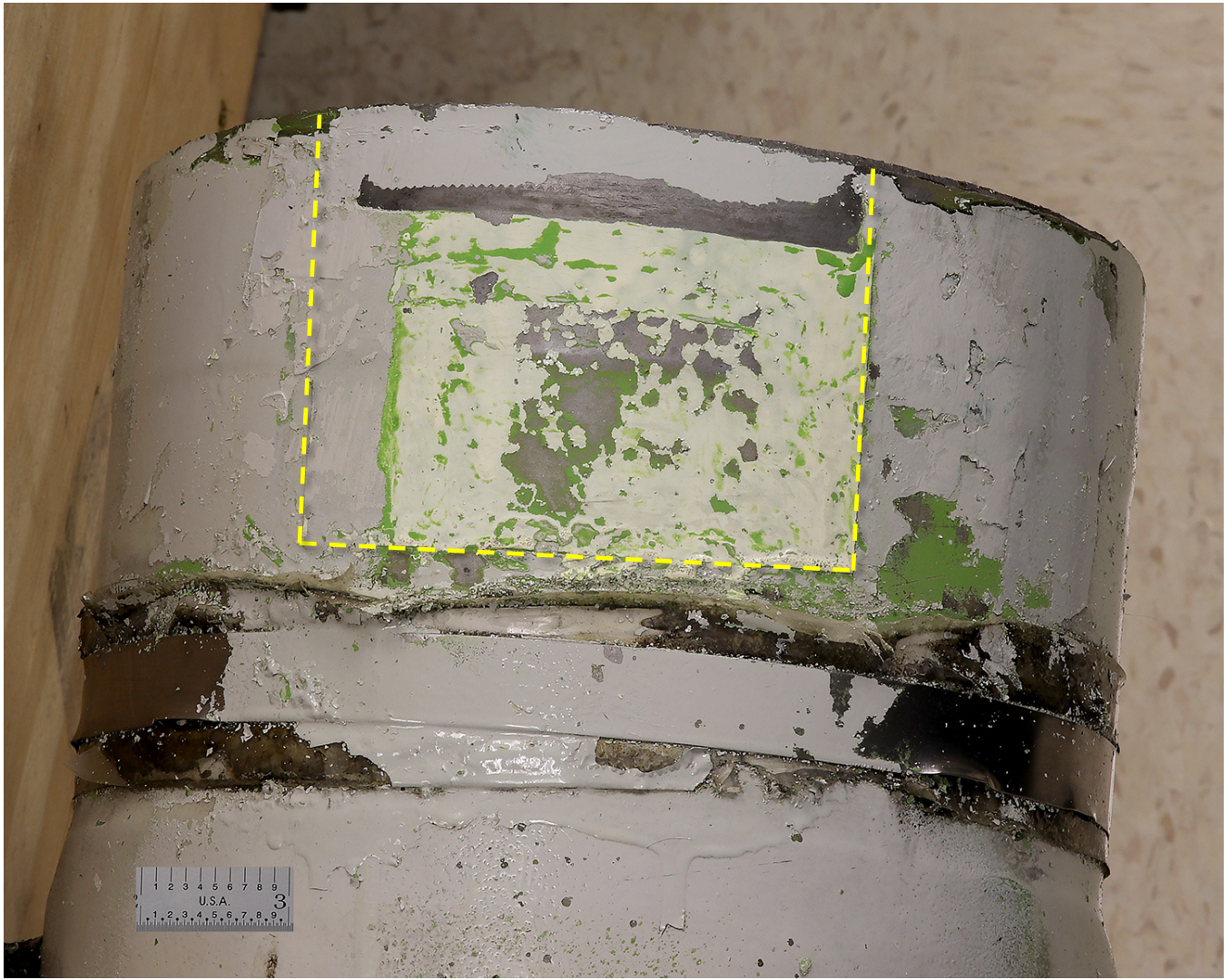
Figure 6 – View of the lower fracture surface, after some paint stripping. The boxed area highlights the masked and repainted area.
