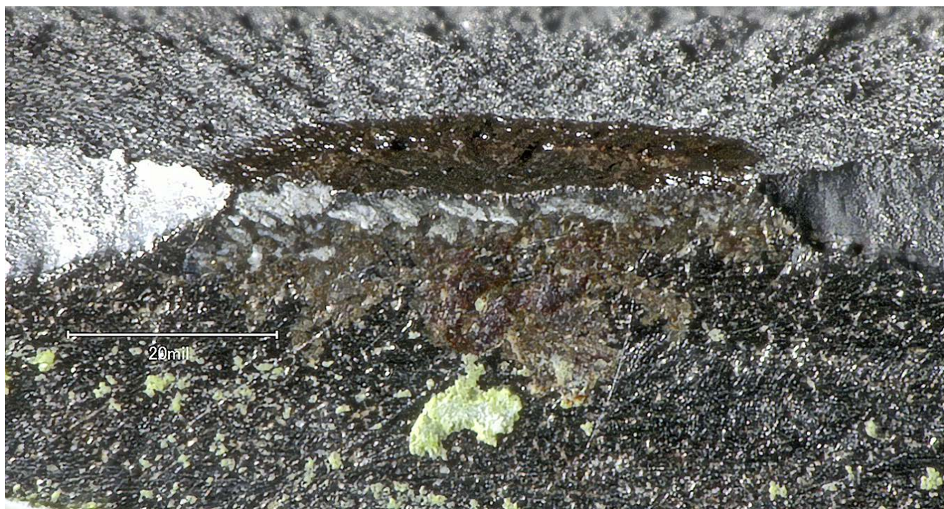
Figure 11 – The thumbnail crack in Figure 10, shown at an angle to show the exterior of the cylinder.
