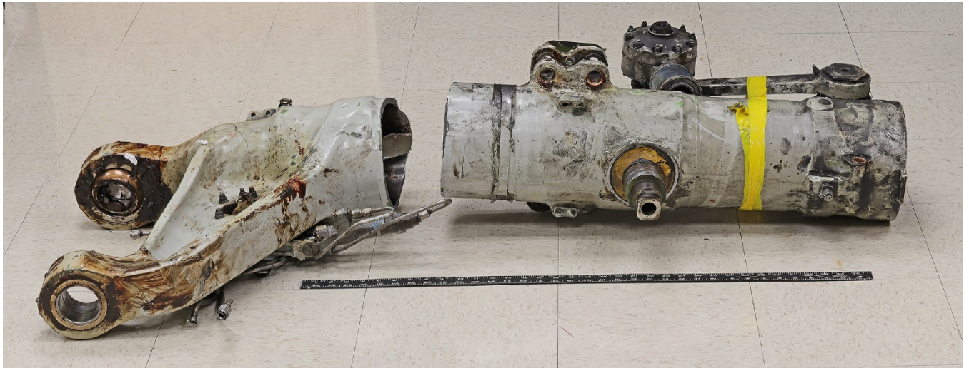
Figure 1 – The fractured right main landing gear, as received.
