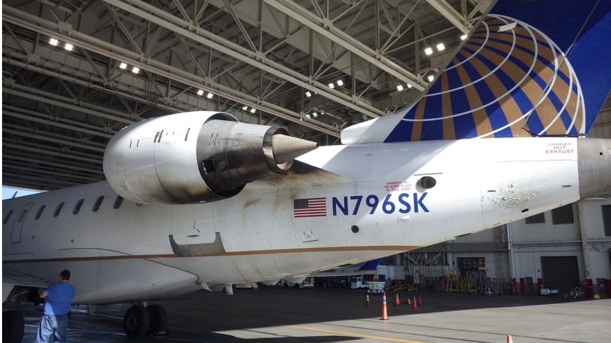
Figure 8. Thermal damage to left side of the airplane
