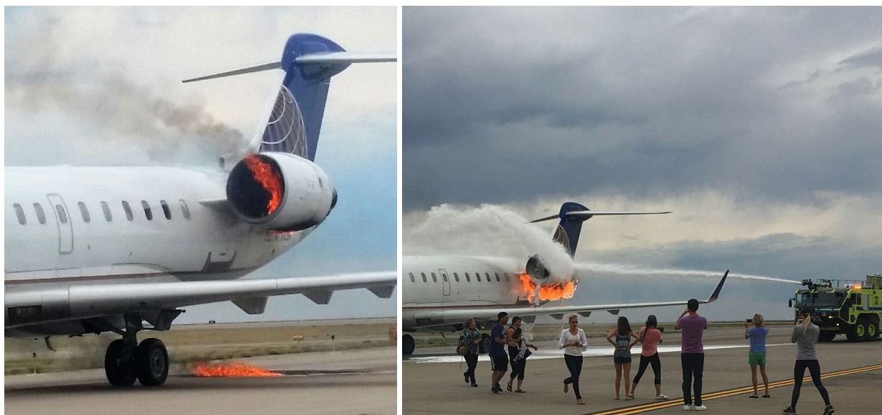
Figure 1. Left engine undercowl fire during passenger egress, two views
