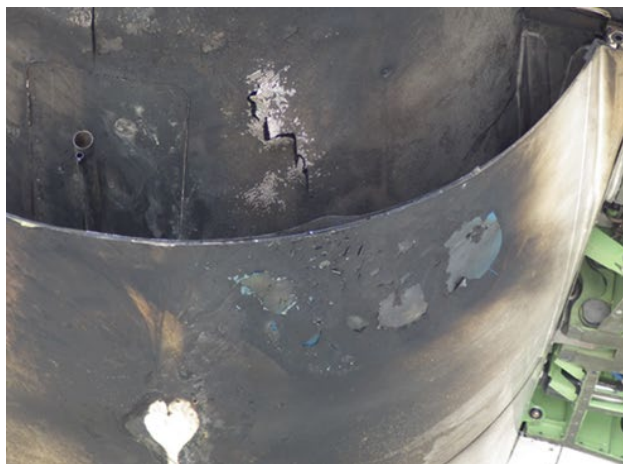
Fig 15. Lower transcowl and core cowl thermal distress
