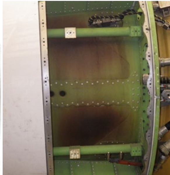
Figure 9. Inlet cowl inner barrel thermal damage Figure 10. FADEC compartment heat distress
