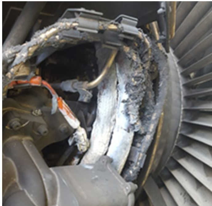
Figure 20. Exemplar engine externals fire damage
