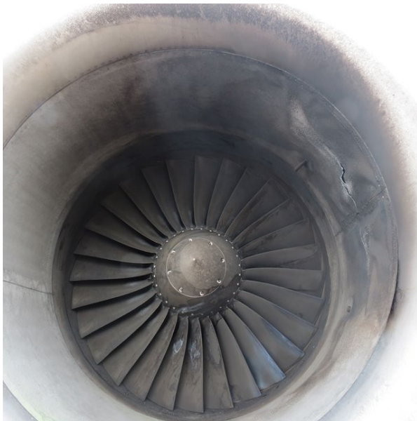
Figure 9. Inlet cowl inner barrel thermal damage Figure 10. FADEC compartment heat distress
