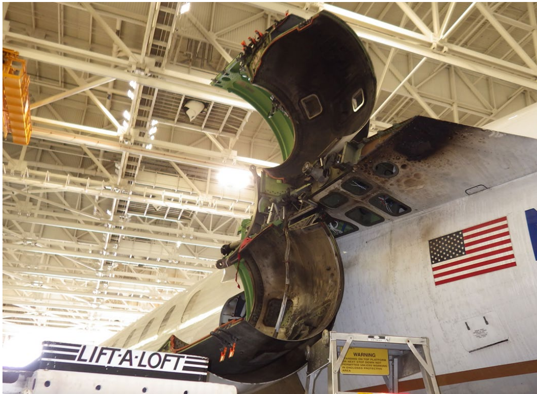
Figure 14. Open cowling doors and view of pylon damage
