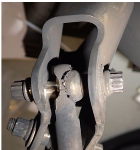
Figure 23. Forward left link. The backed-off nut was not as found
