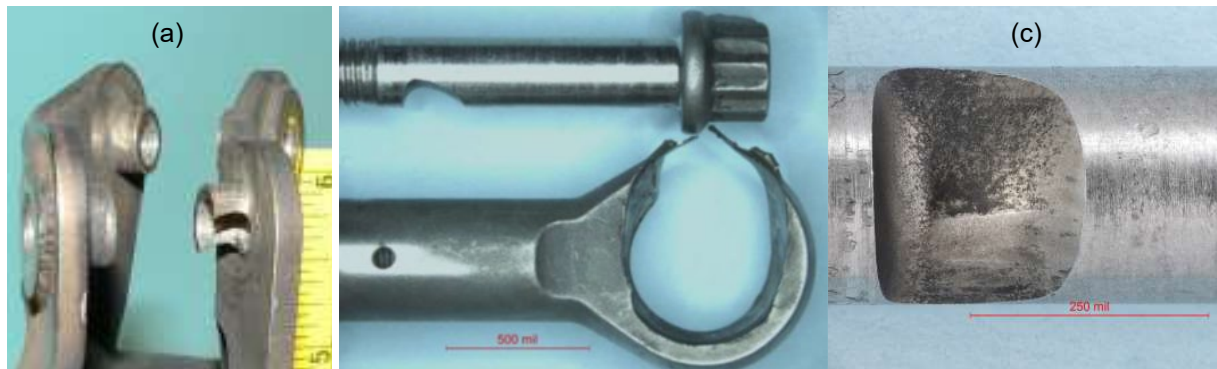
Figure 26. Left forward ECS link manifold-attachment hardware, showing (a) wear-through at manifold fork bushing (b) attachment bolt divot and rod end housing wear through, and (c) close up of bolt shank divot
