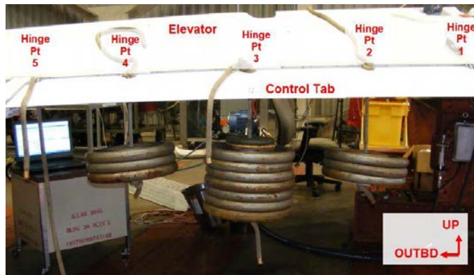
Weights Simulating Horizontal Wind Gust Loads
