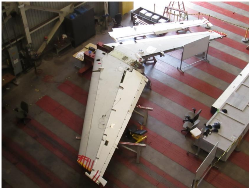
Overview of accident aircraft elevators on test stand at test facility
