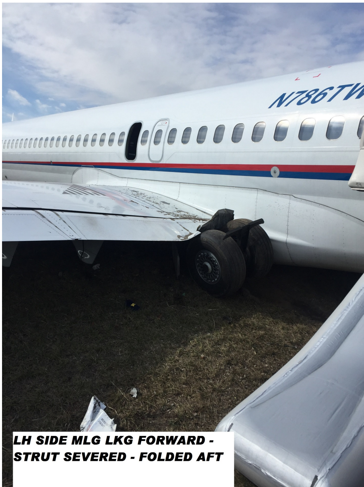
Figure 23 – Left hand main gear damage
