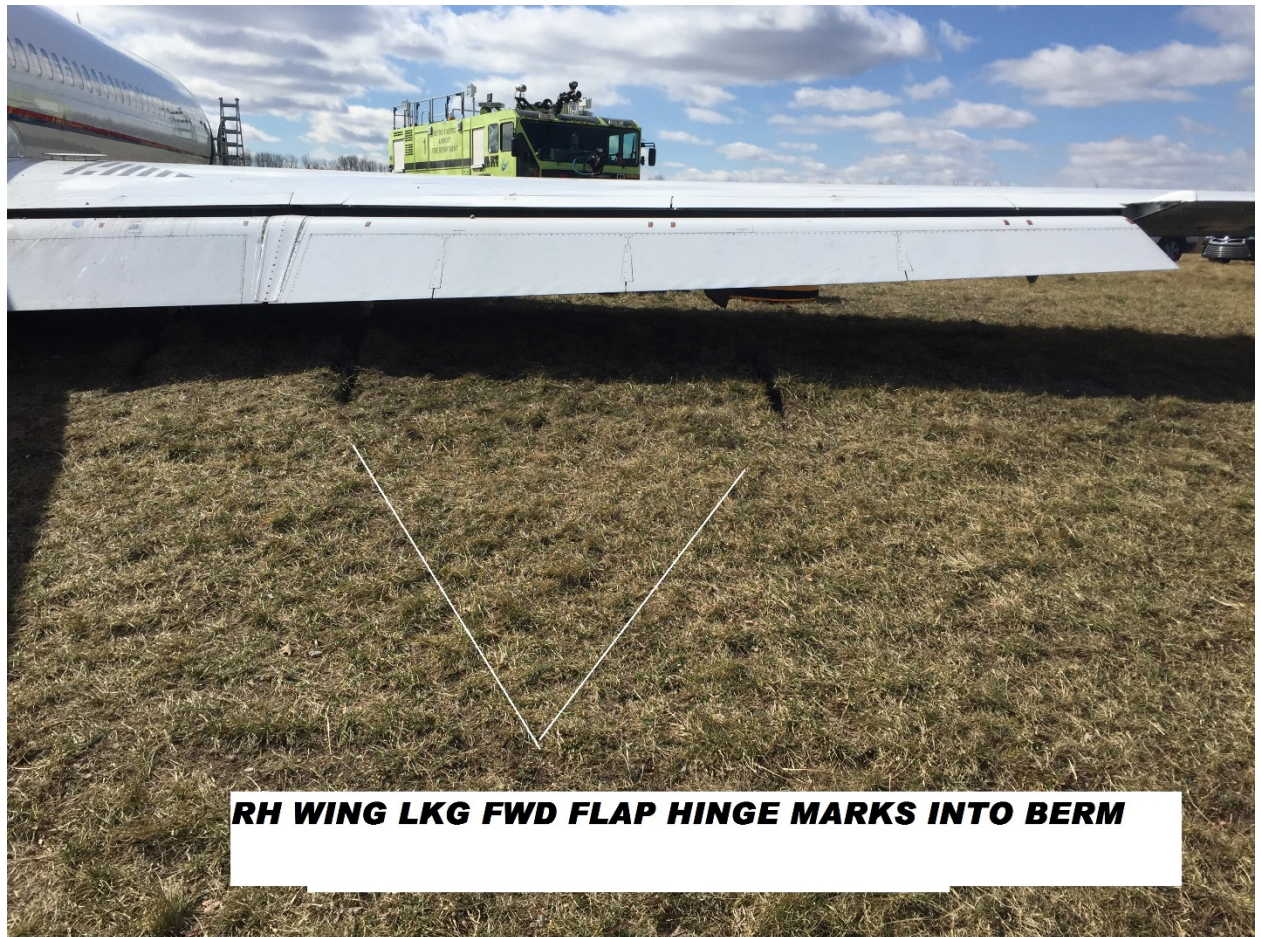
Figure 15 - Right wing flap track ground scars
