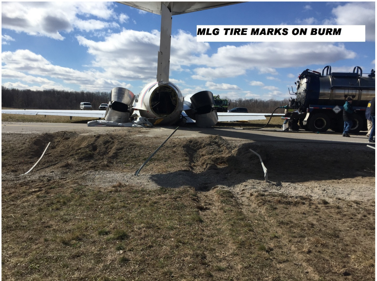
Figure 25 – Main gear marks at impact area
