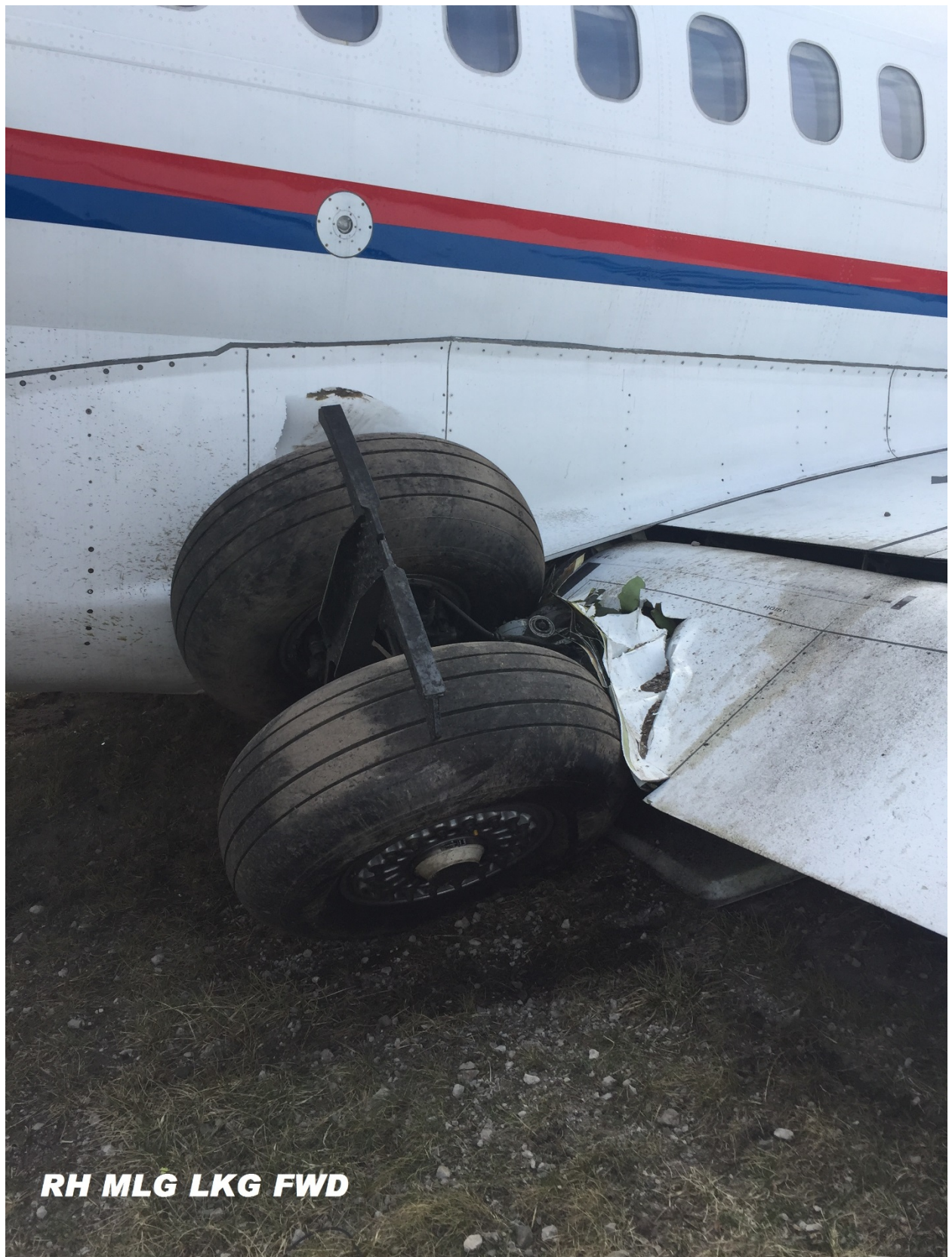
Figure 24 – Right hand main gear damage
