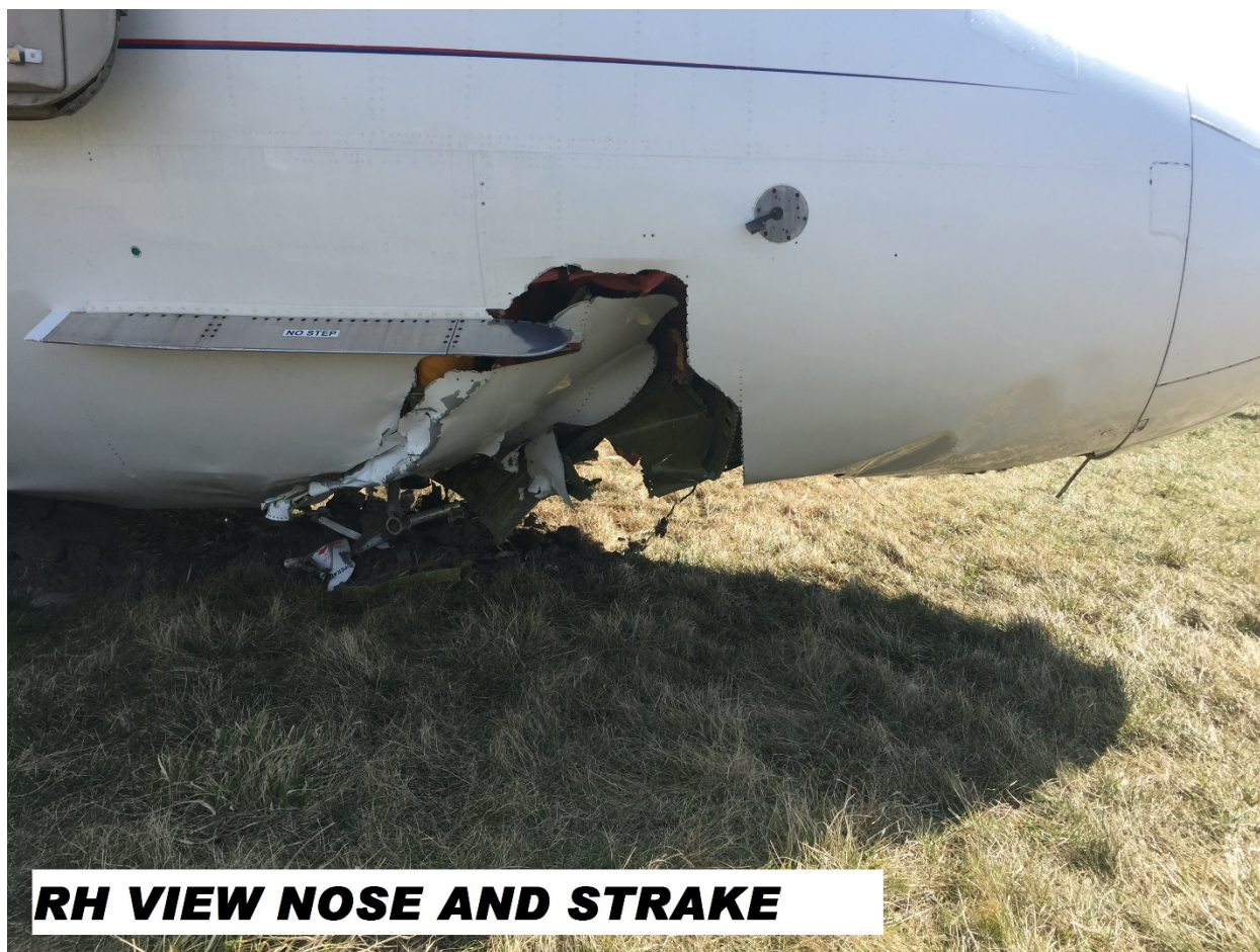
Figure 7 – Right nose damage close up
