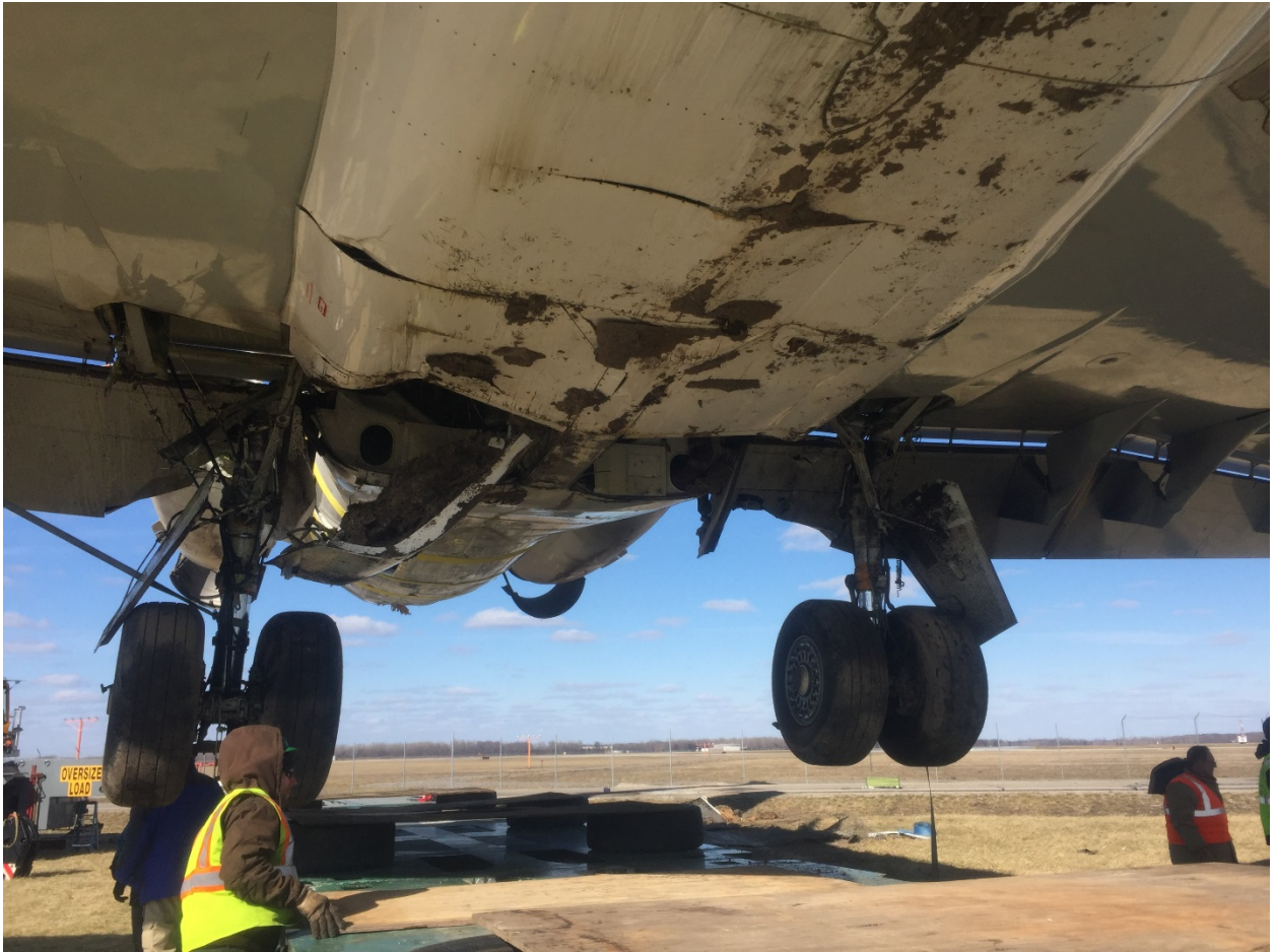
Figure 12 – Lower fuselage damage
