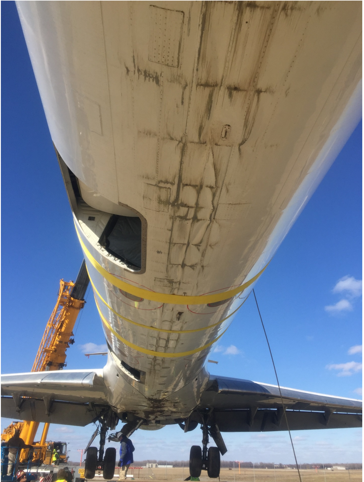
Figure 11 – Lower fuselage damage
