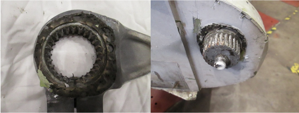
Figure 25 - Mating spline surfaces of the left elevator stop arm and torsion bar
