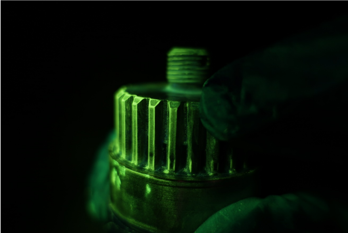
Figure 44 - Right torsion bar splines during magnetic particle testing
