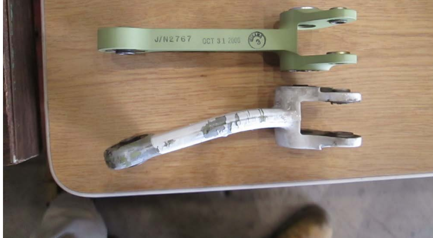
Figure 34 - View looking down at accident and exemplar RH elevator actuating crank
