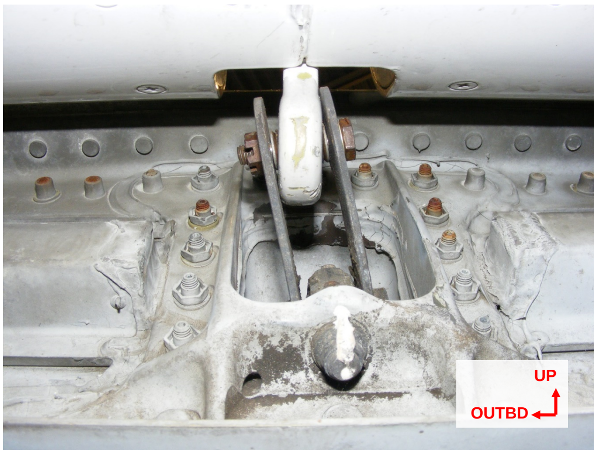
Figure 53 - Gear Tab Inboard Linkage in over-centered condition
