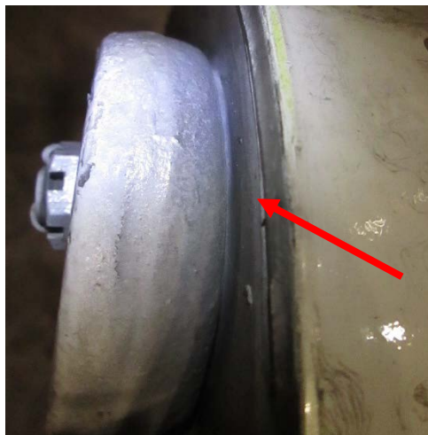
Figure 27 - Sealant between the RH elevator stop arm and closeout rib (noted by red arrow).
