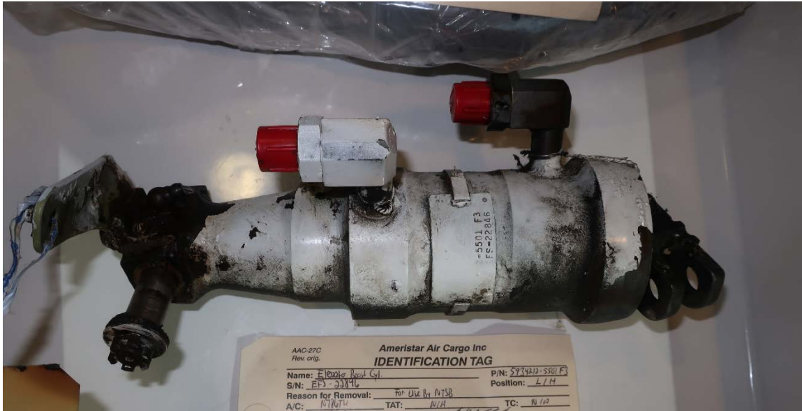
Figure 38 - LH Elevator boost cylinder prior to bench testing
