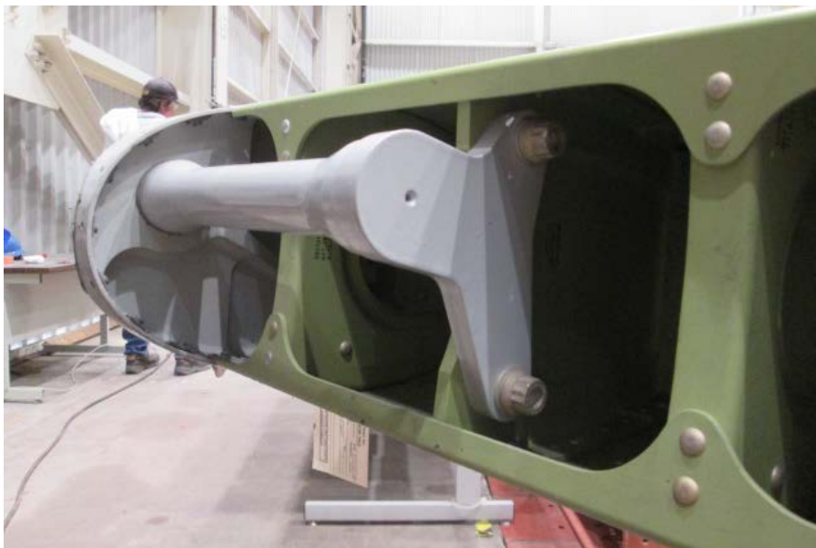
Figure 24 - Torsion bar installation on LH elevator
