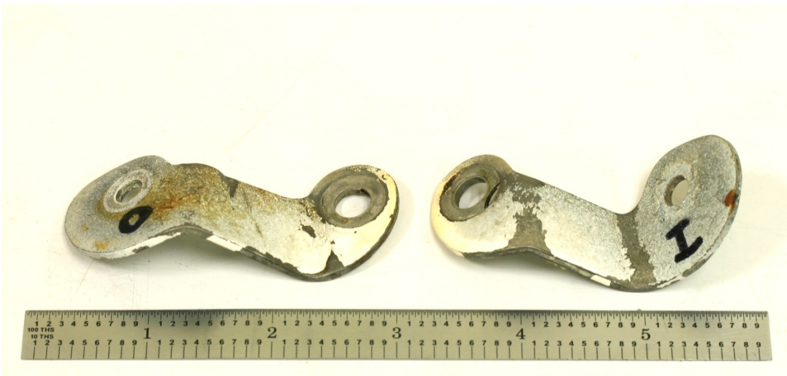
Figure 41 – Outboard (O) and inboard (I) links prior to hardness testing
