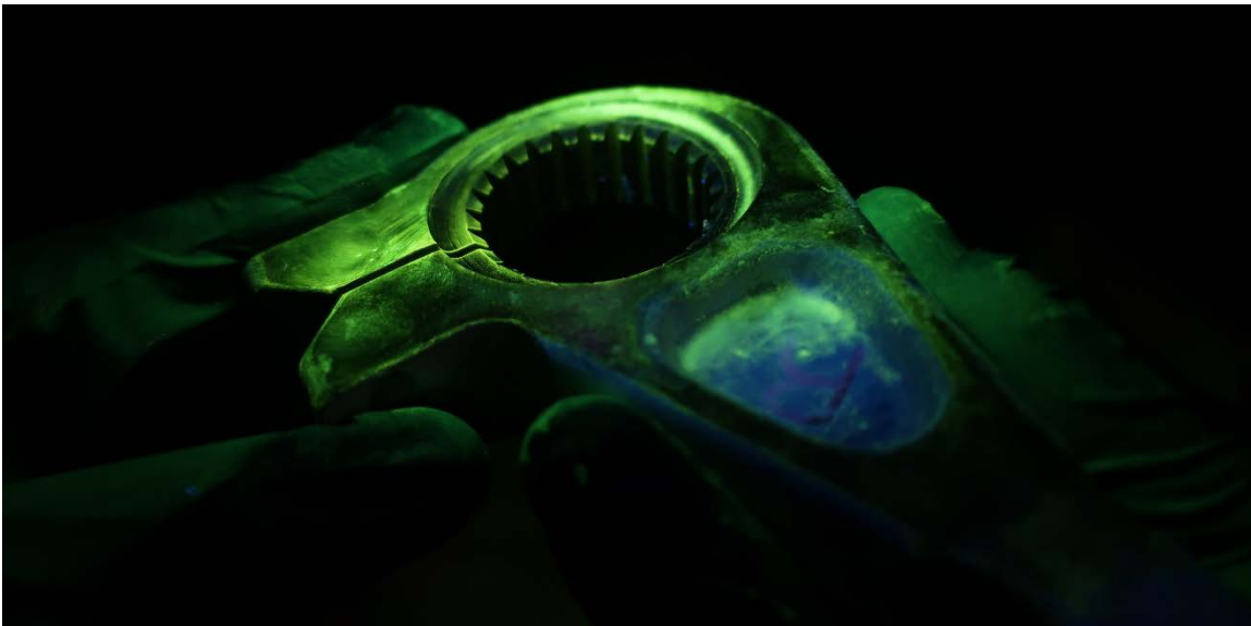
Figure 45 - Right stop arm splines during magnetic particle testing
