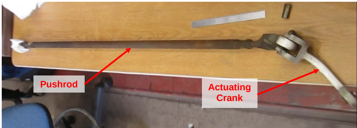
Figure 32 - RH Inboard geared tab pushrod and actuating crank
