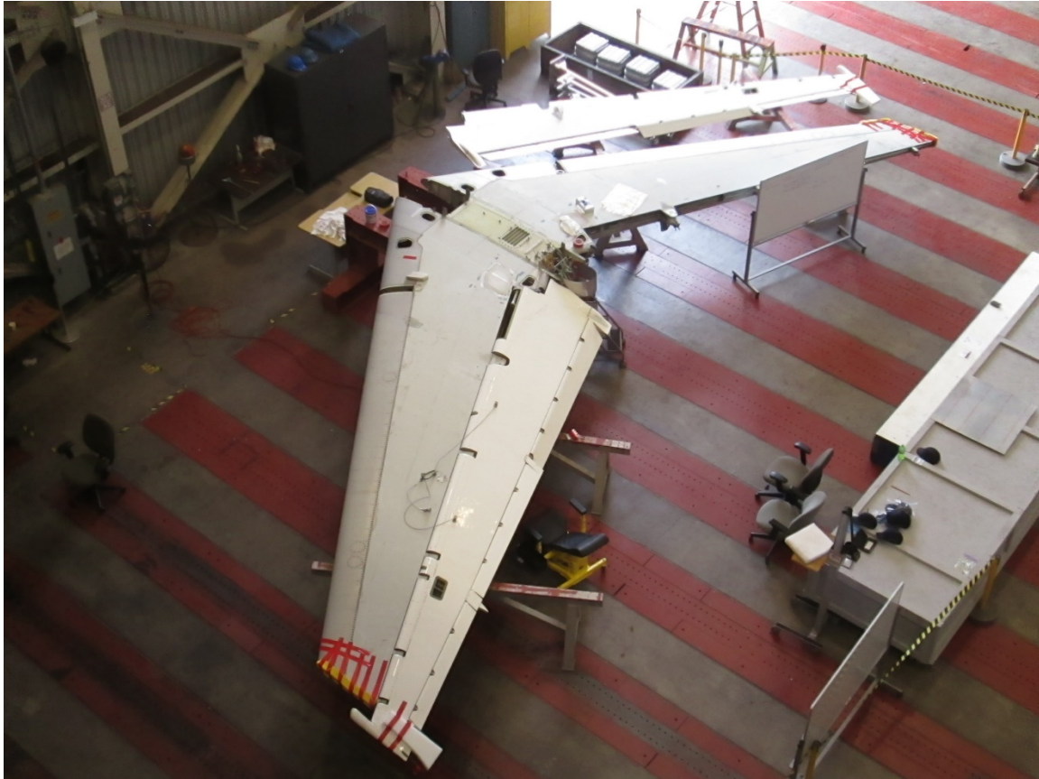
Figure 21 - Overview of accident aircraft elevators on test stand at test facility
