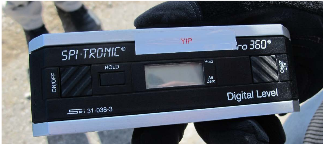
Figure 19 - Digital inclinometer used for travel checks
