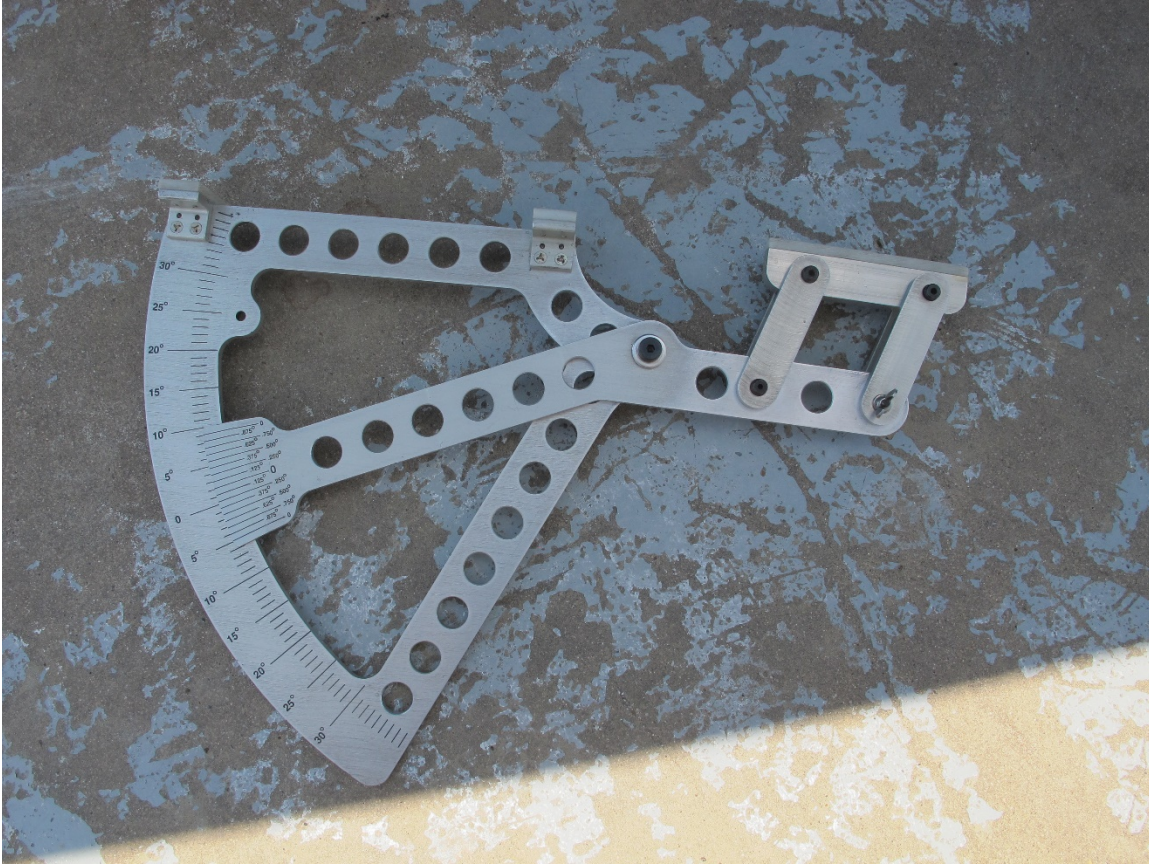
Figure 46 - Rigging protractor used during control tab travel tests
