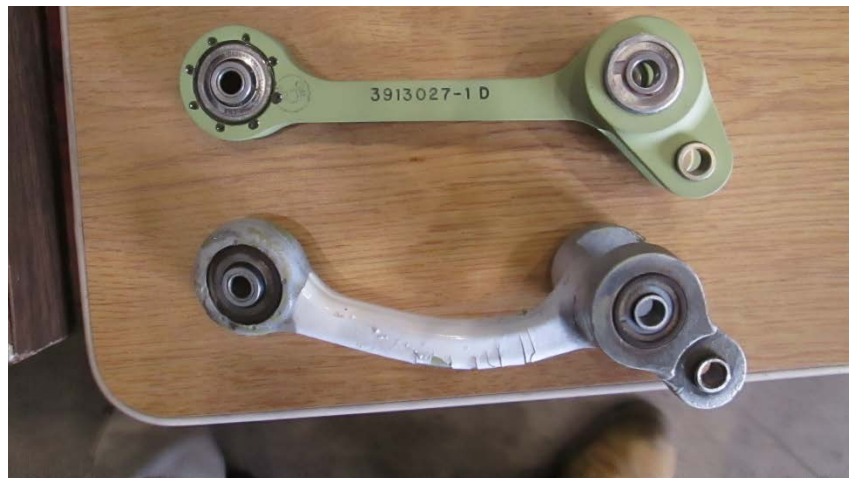
Figure 33 - Side view comparison of accident and exemplar RH actuating crank
