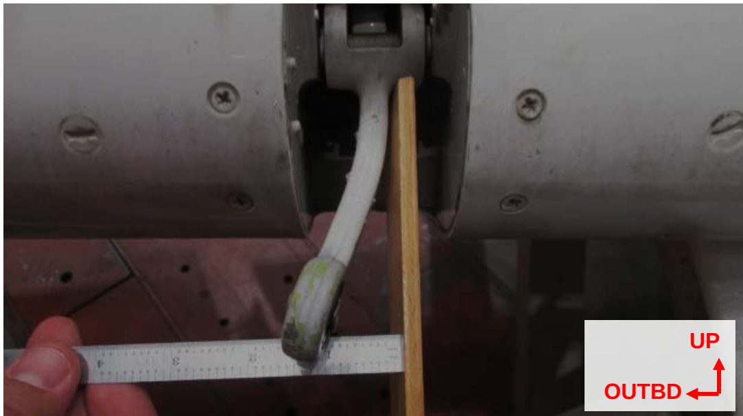
Figure 30 - RH Elevator actuating crank arm displacement
