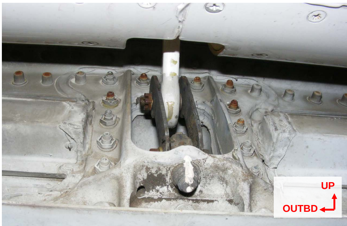
Figure 52 - Gear Tab Inboard Linkage in nominal condition
