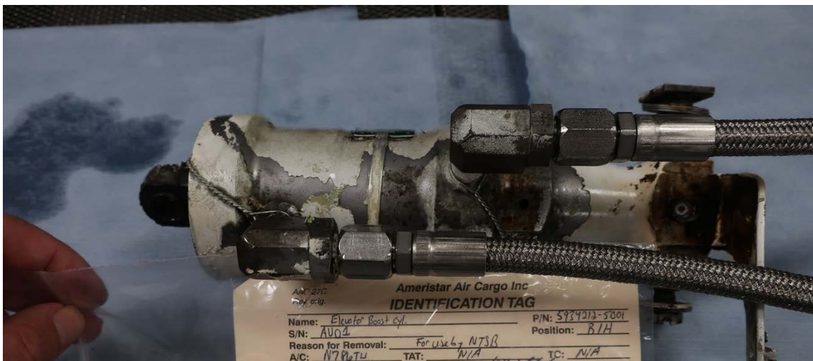
Figure 39 - RH Elevator boost cylinder hooked up to test bench
