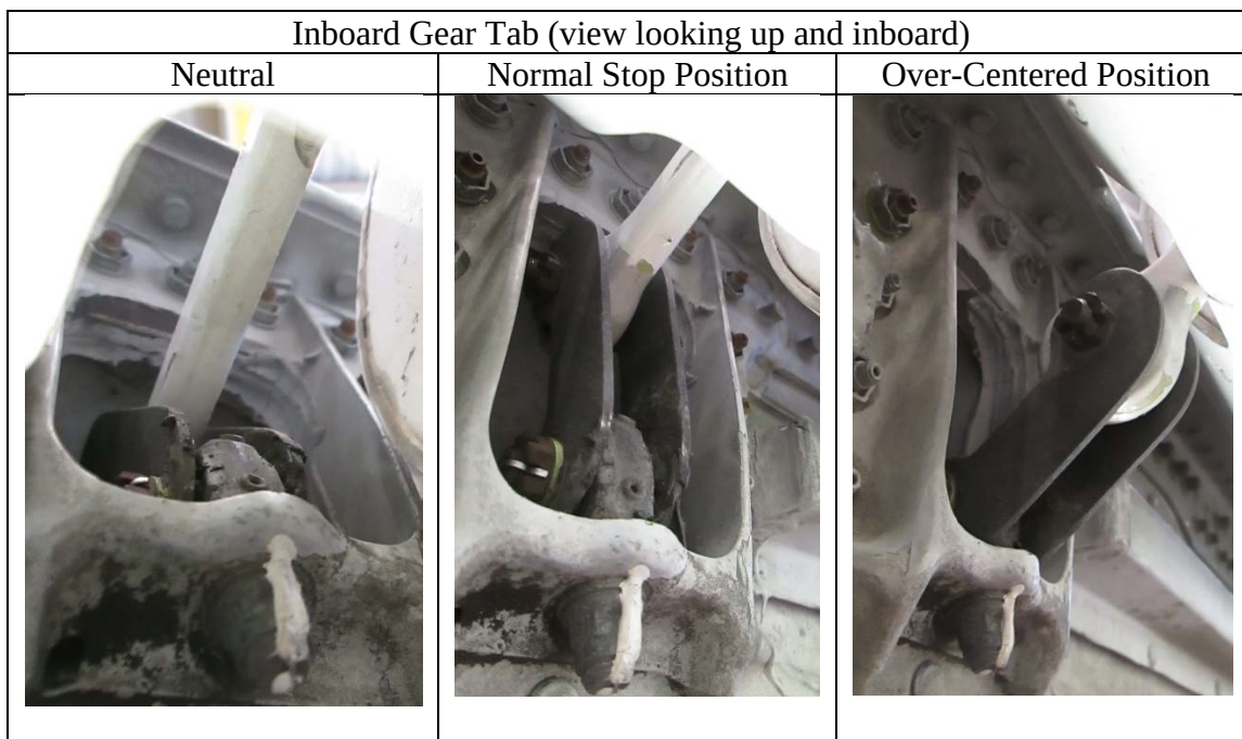
Figure 47 - Inboard geared tab link and actuating crank position compared to elevator position
