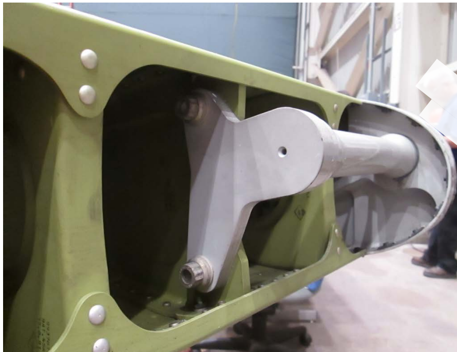
Figure 31 – Torsion bar installation on RH Elevator
