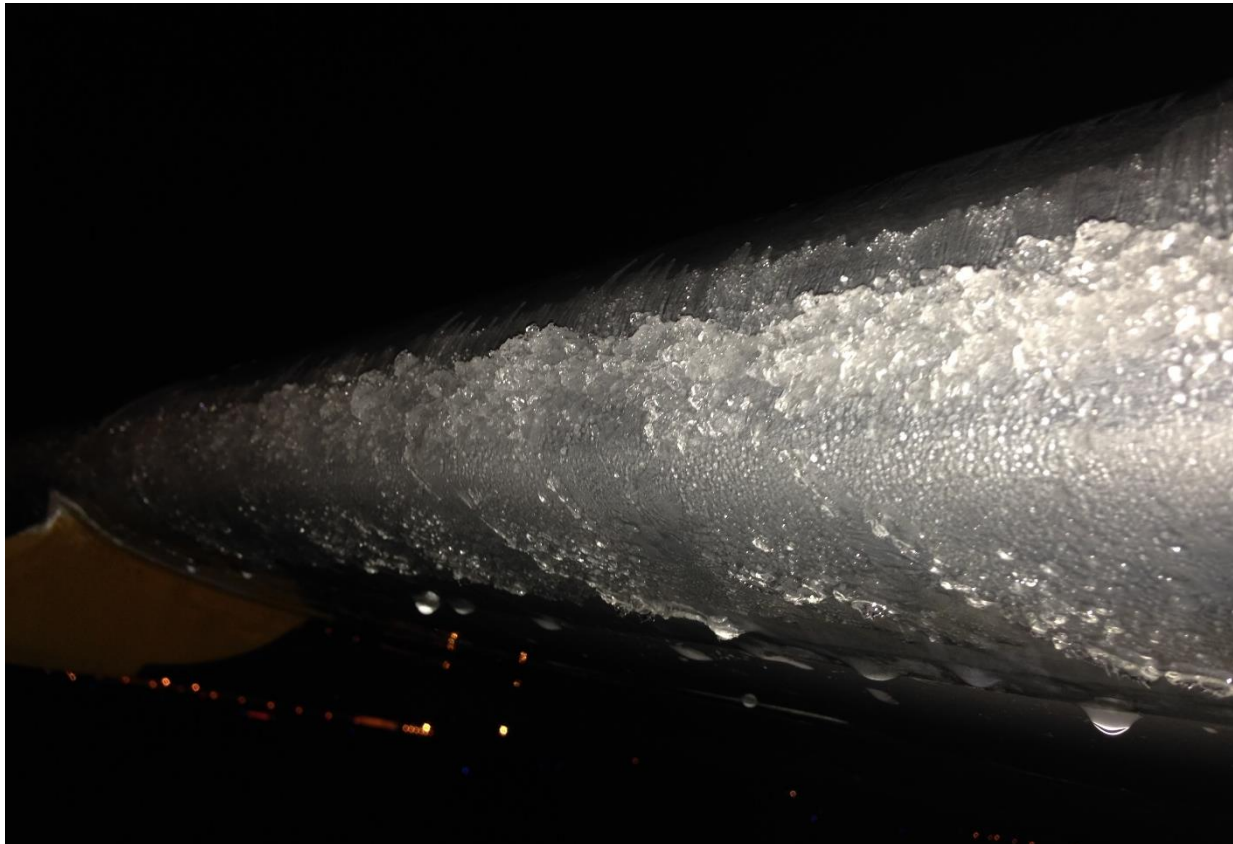
Figure 1: Picture Taken Approximately 40 Minutes After Gate Arrival of Ice Build-Up Discovered On Wing
