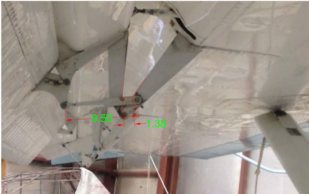
Figure 11 – N491K center flap hinge at flaps 30
