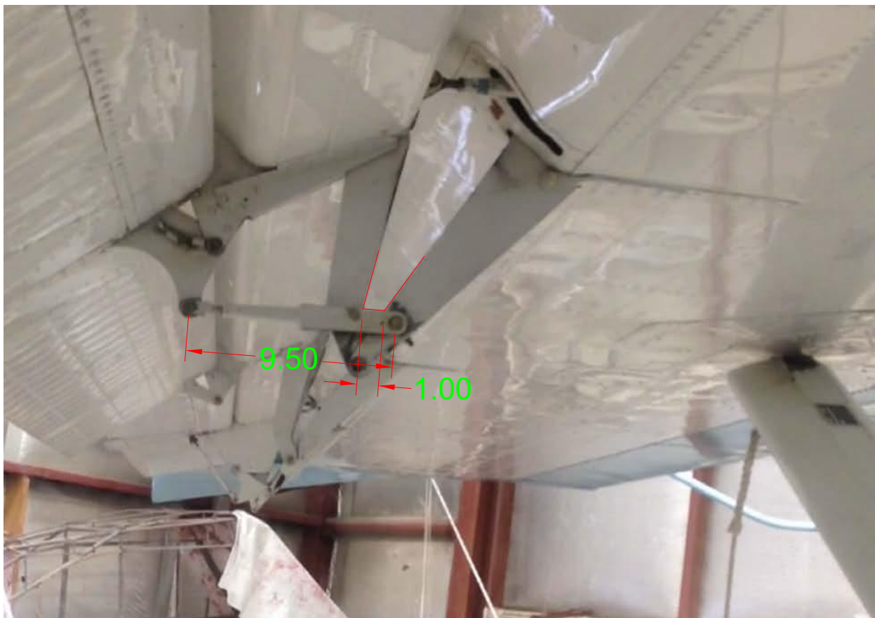
Figure 10 – N491K center flap hinge at flaps 20
