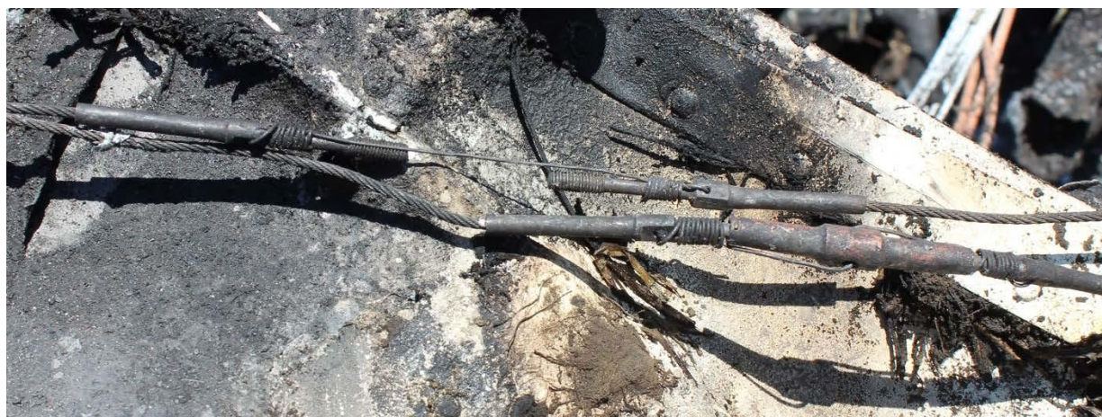
Figure 4 – Pitch trim cable turnbuckles
