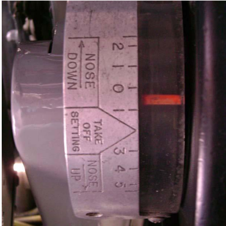
Figure 5 – Trim indication on similar, intact airplane
