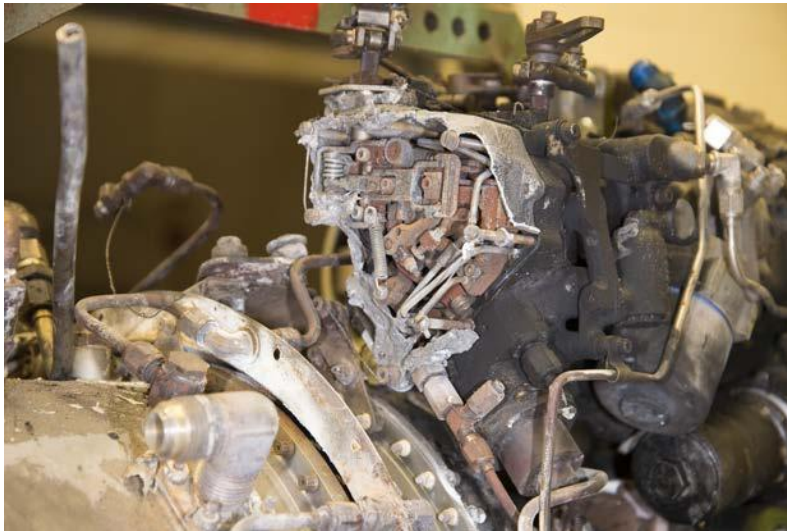
Figure 13 – Fuel Control Unit – Melted Aft Cover
