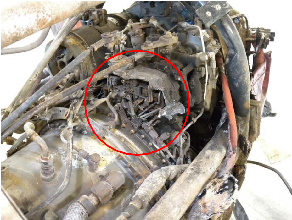
Figure 10 – Fuel Control Unit (FCU) - Breached
