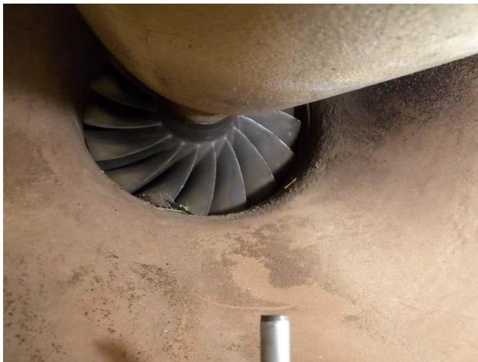
Figure 8 – 1 st Stage Impeller – Intact
