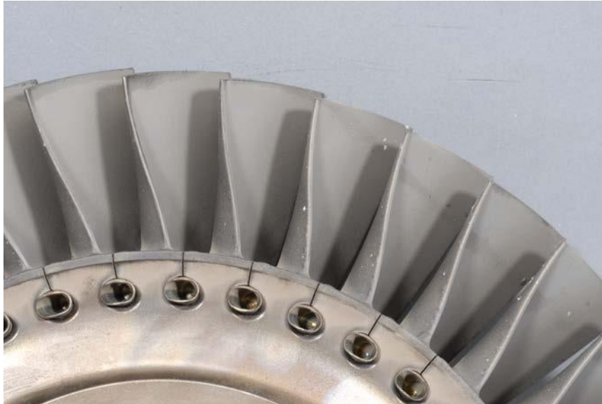
Figure 26 – 2 nd Stage Turbine Blisk – Metal Spray (Silver Speckles)
