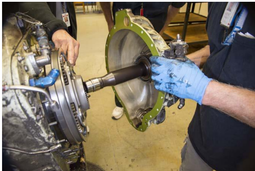
Figure 14 – Nose Cone & Propeller Shaft Being Removed
