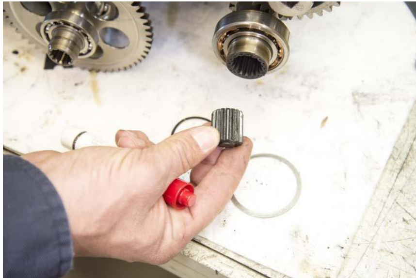
Figure 19 – Sheared Starter Generator spline
