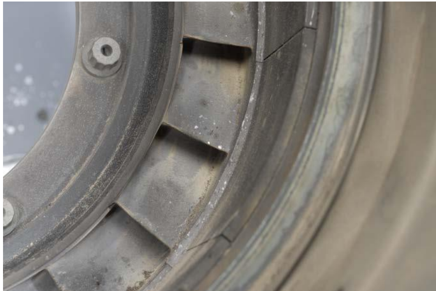
Figure 28 – 1 st Stage Turbine Nozzle – Metal Spray (White Speckles)
