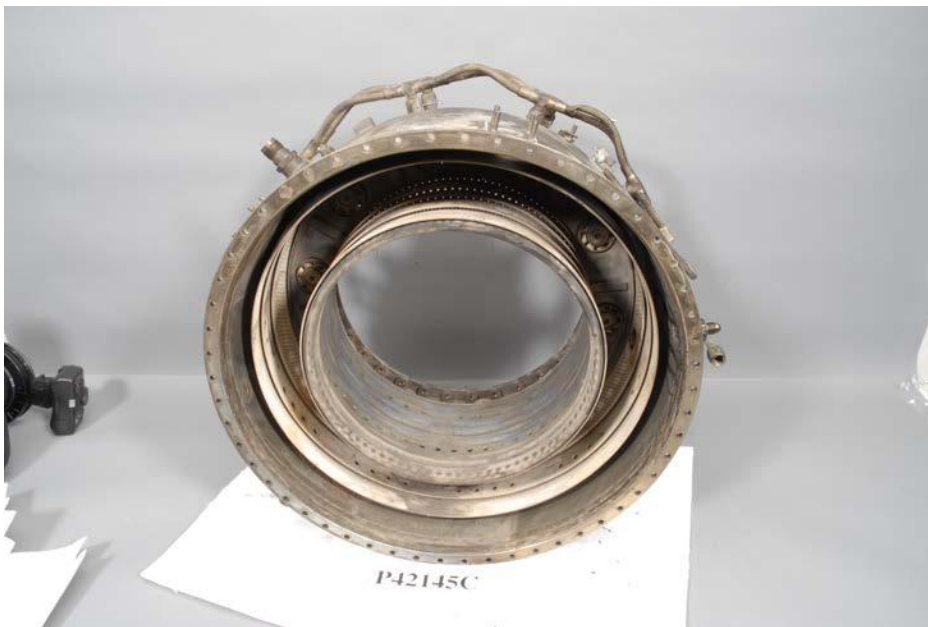
Figure 30 – Combustor Housing and Liner
