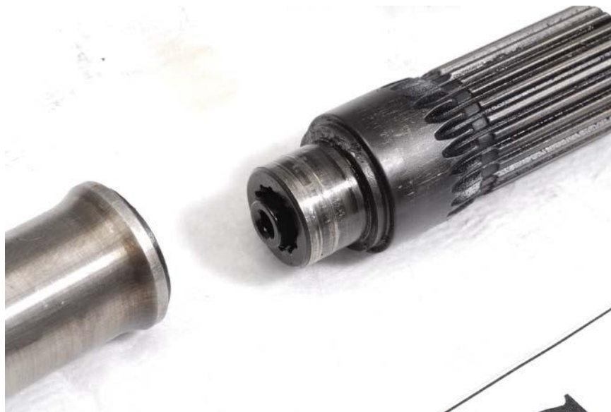
Figure 24 – Sheared Torsion Shaft
