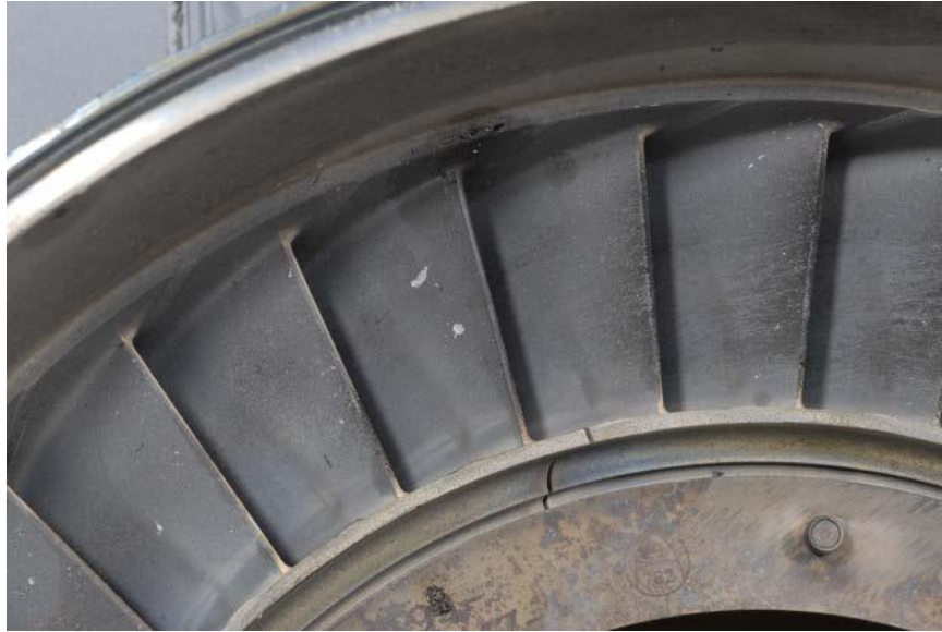
Figure 27 – 2nd Stage Turbine Nozzle – Metal Spray (Silver Speckles)
