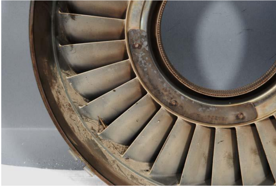
Figure 25 – 3 rd Stage Turbine Nozzle – Metal Spray (White Speckles)
