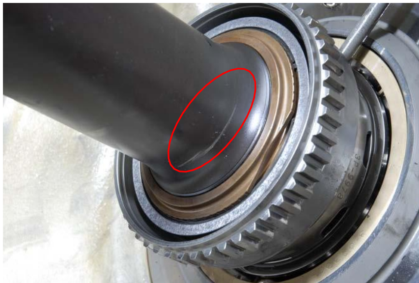
Figure 16 – Propeller Shaft – Rotational Scoring
