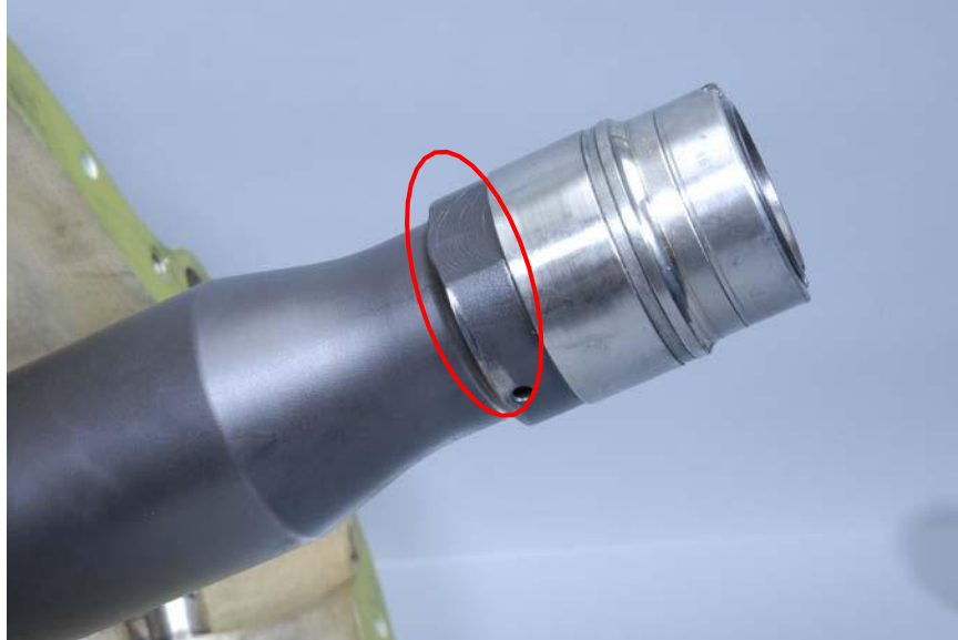
Figure 15 – Propeller Shaft – Rotational Scoring
