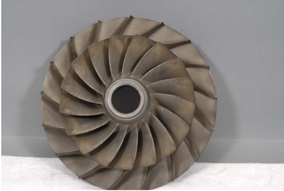
Figure 29 – 1 st Stage Impeller Wheel – Intact
