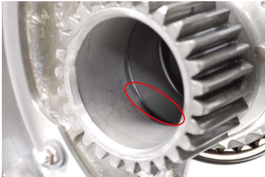
Figure 18 – Rotational Scoring On Inner Bore Of Sun Gear
