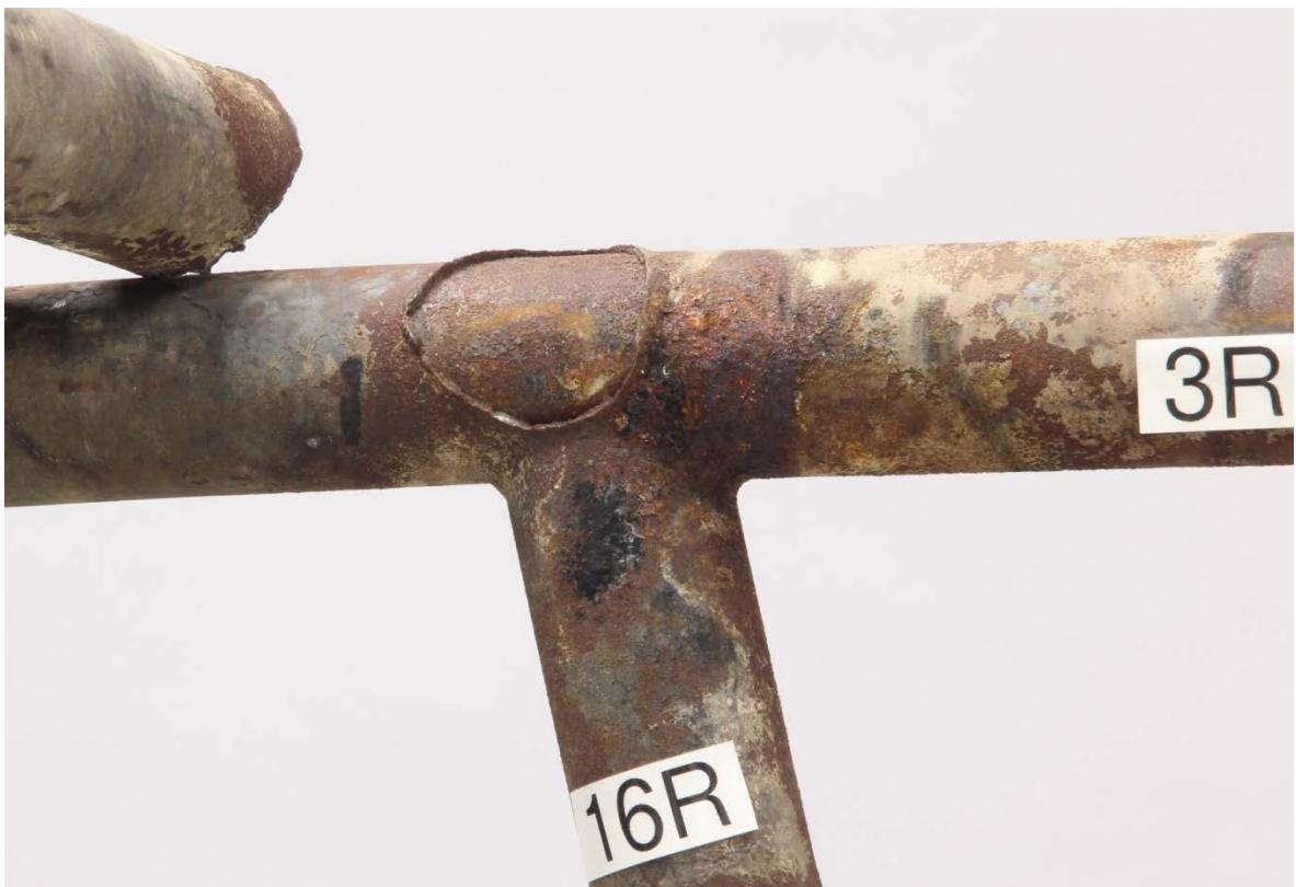
Figure 3. Two views of typical fractures and crack in the engine mount assembly.
