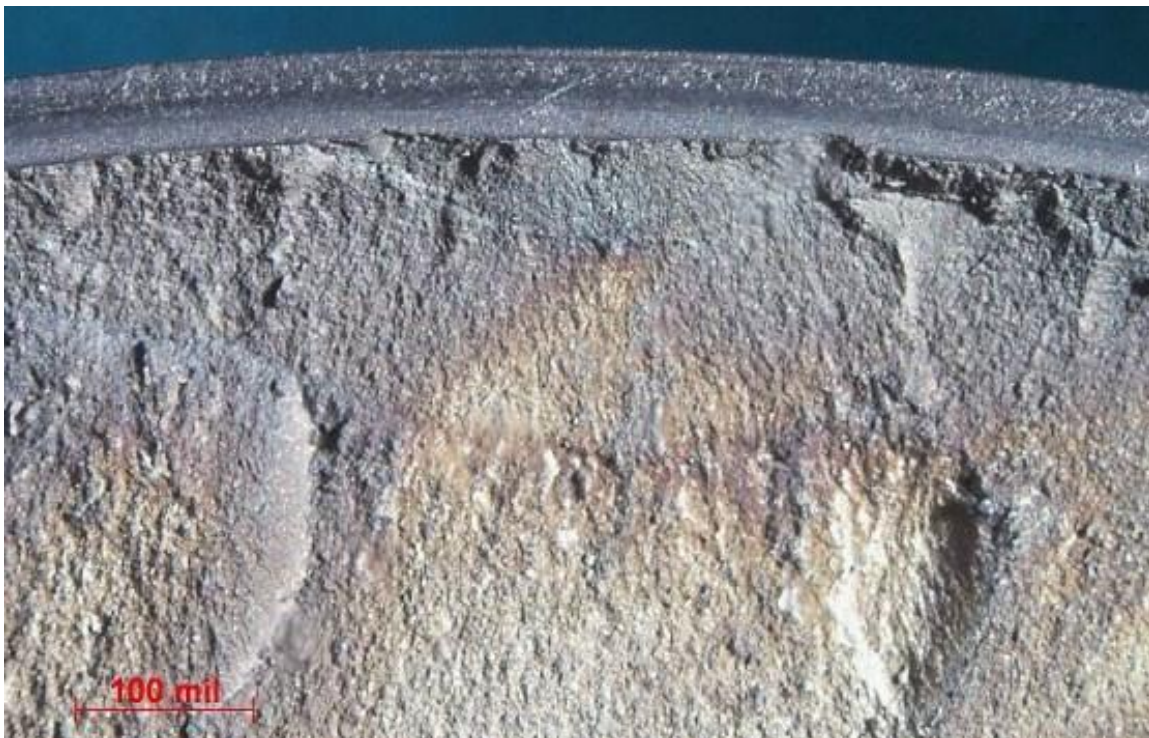
Figure 14 – Closer view of the thumbnail feature near the thread root depicted in Figure 10a.
