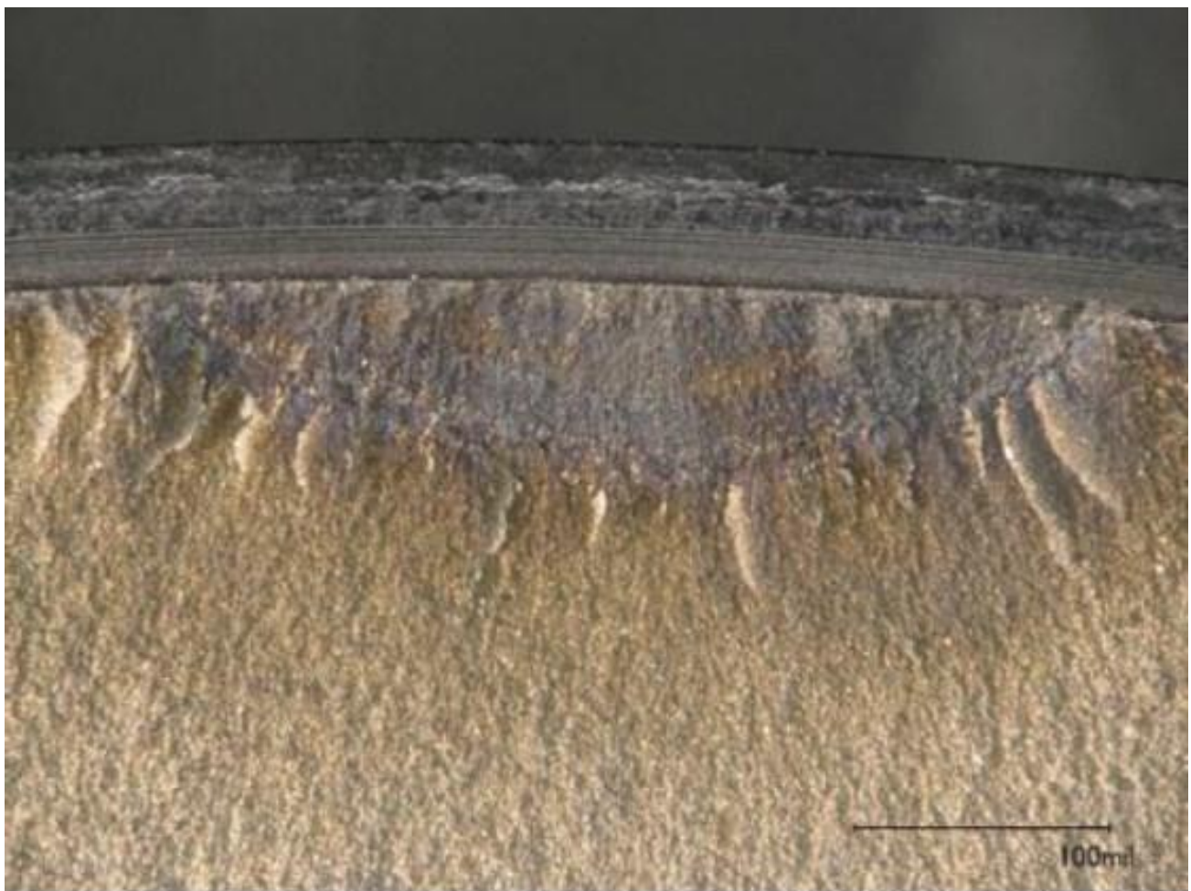
Figure 16 – Closer view of the thumbnail feature and discoloration in Figure 15b.
