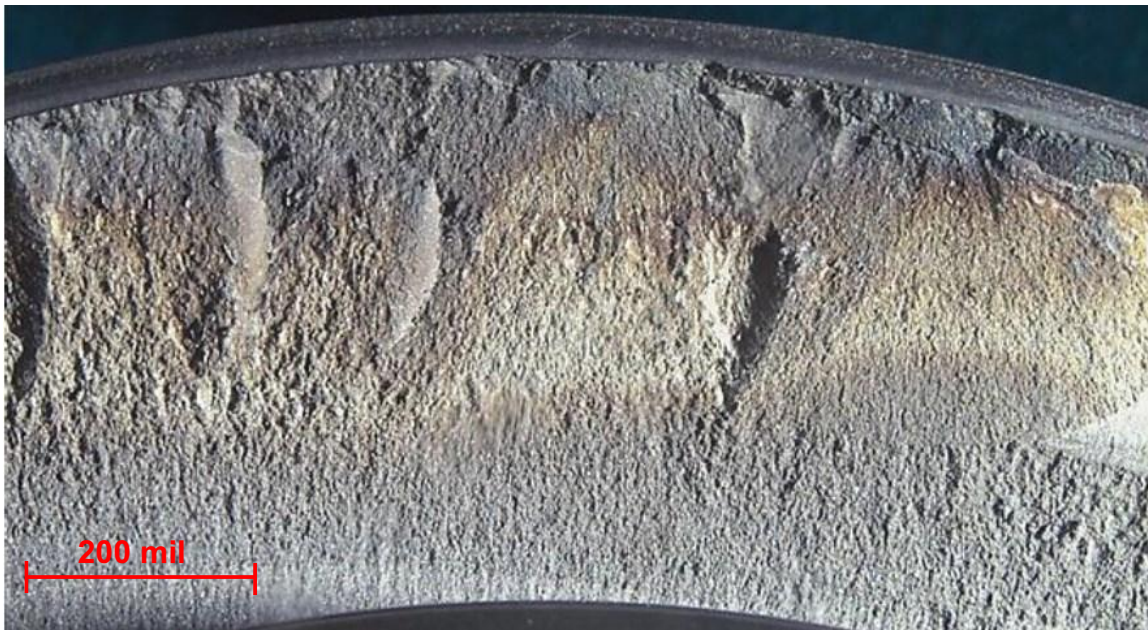
Figure 10 – Thumbnail features on the fracture surface (after cleaning).
