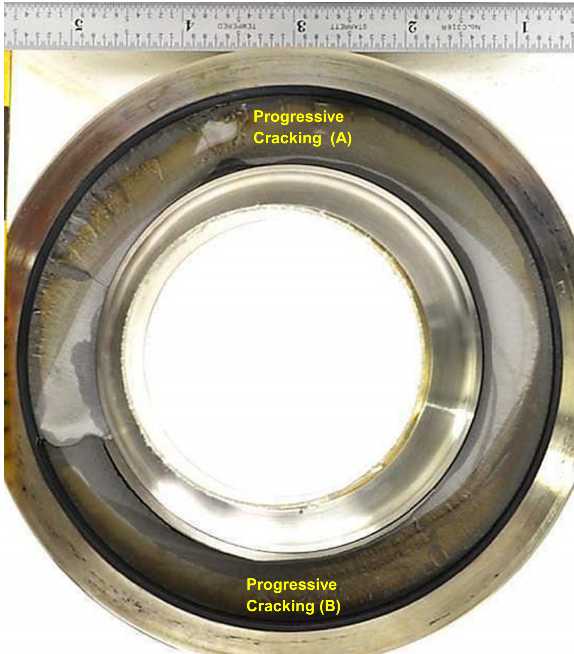
Figure 6 – The fracture surface of the fan midshaft forward section, aft looking forward. The fracture surface shows features consistent of two modes of failure: one progressive and one overstress.
