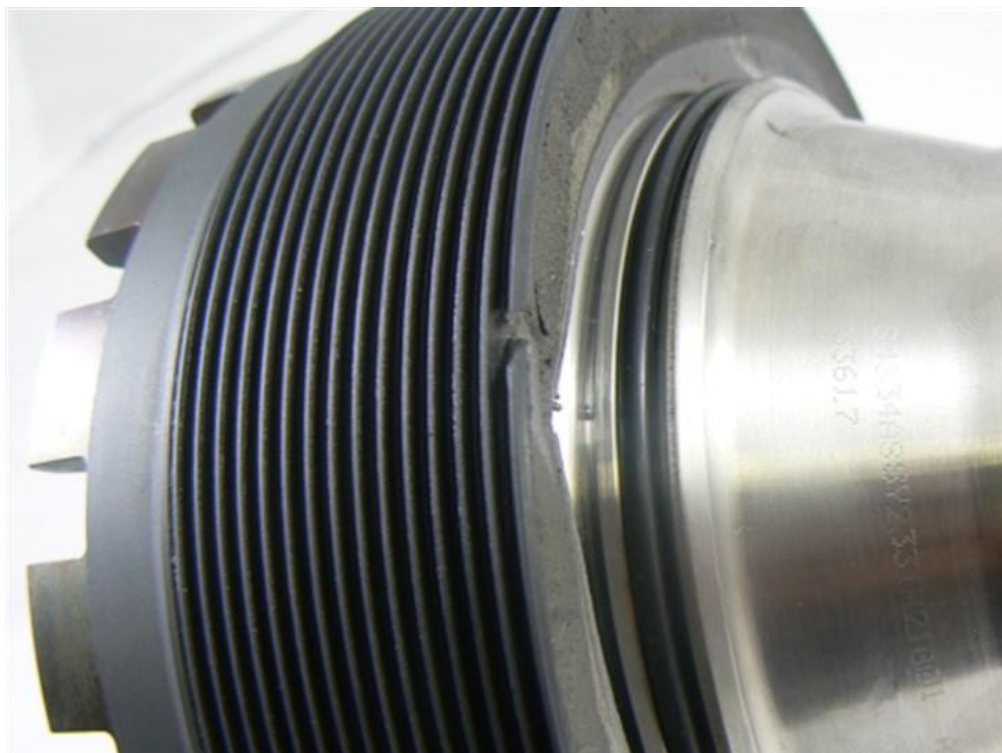
Figure 8 – The forward fan midshaft segment, showing a break in the aft most outer thread at the location of the fracture.
