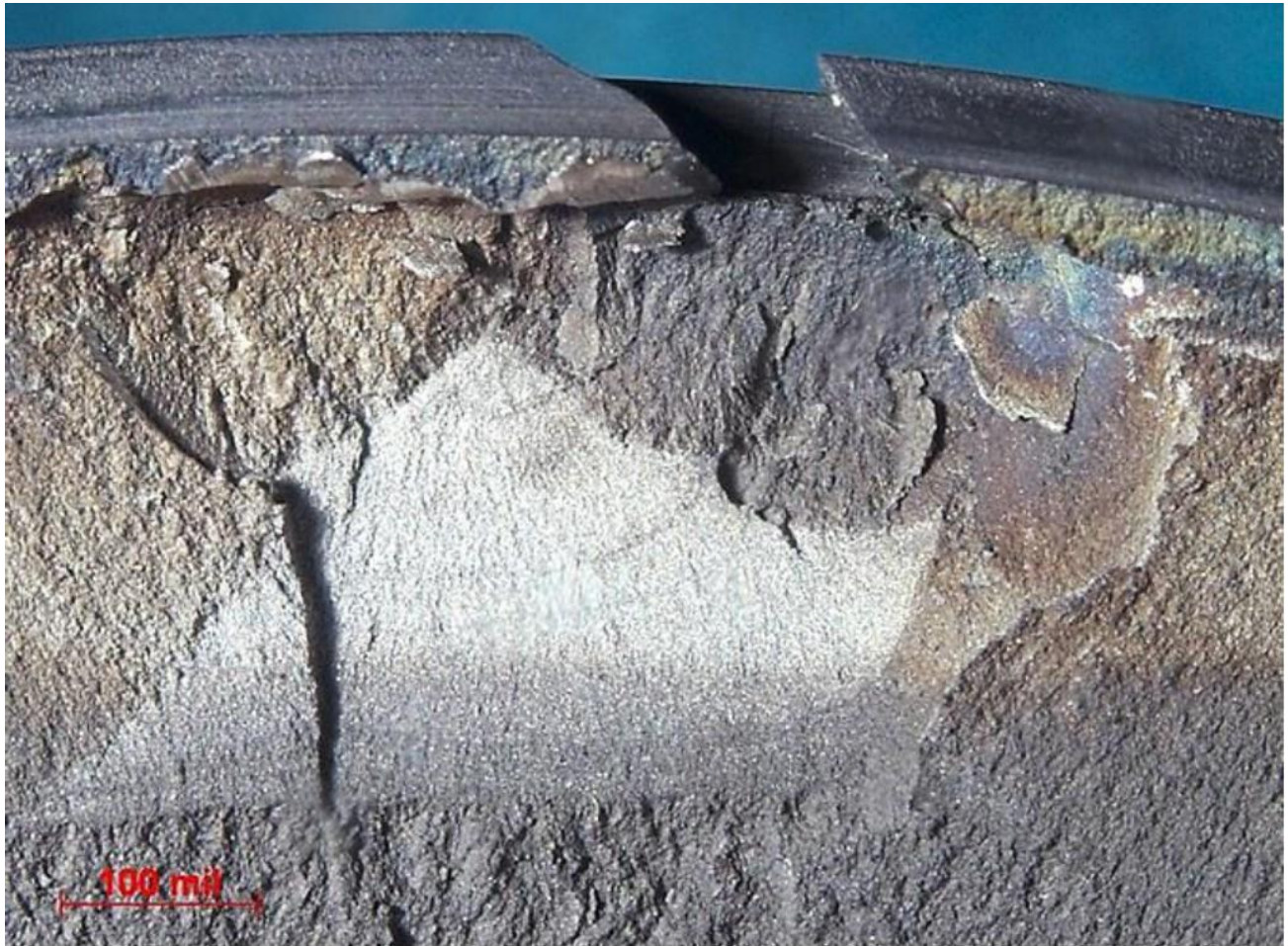
Figure 12 – Closer look at the fracture surface from Figure 11.
