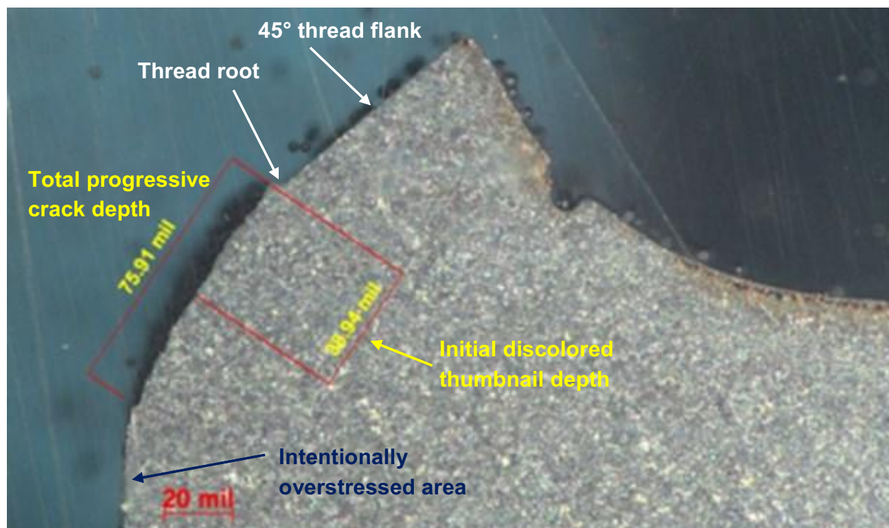
Figure 44 – Optical metallograph of a cross-section of the largest fracture surface at the aft most thread root.
