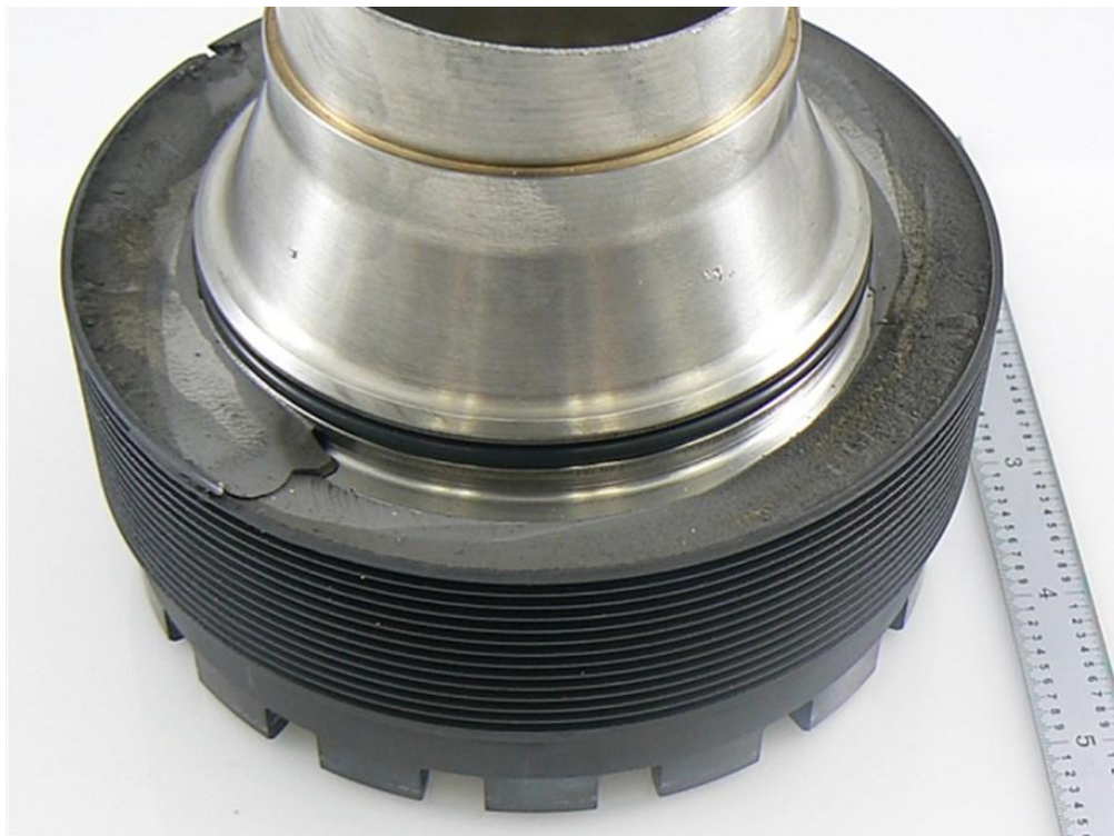
Figure 7 – The forward fan midshaft section illustrated in Figure 6, after removal of the coupling nut with the center vent tube still attached.
