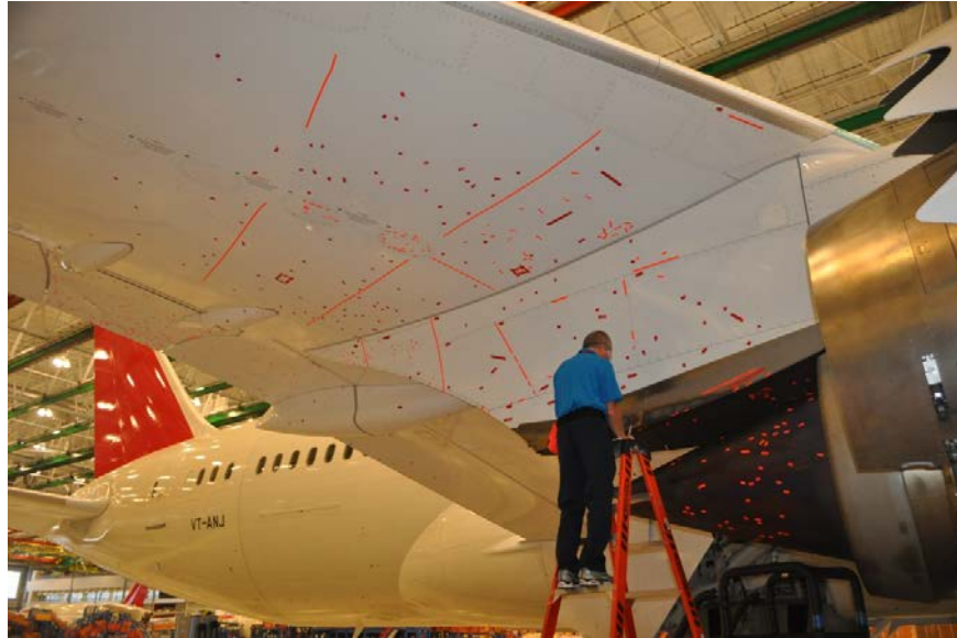
Photo No. 40: View of underside of right wing aft of engine showing impact marks marked with red tape. Also shown is outboard side of right engine's pylon showing impact marks marked with red tape. (GE)
