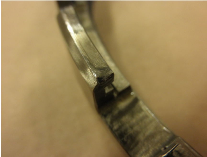
Photo No. 38: Close up of impact mark on No. 5 bearing retaining nut wrenching lug.
