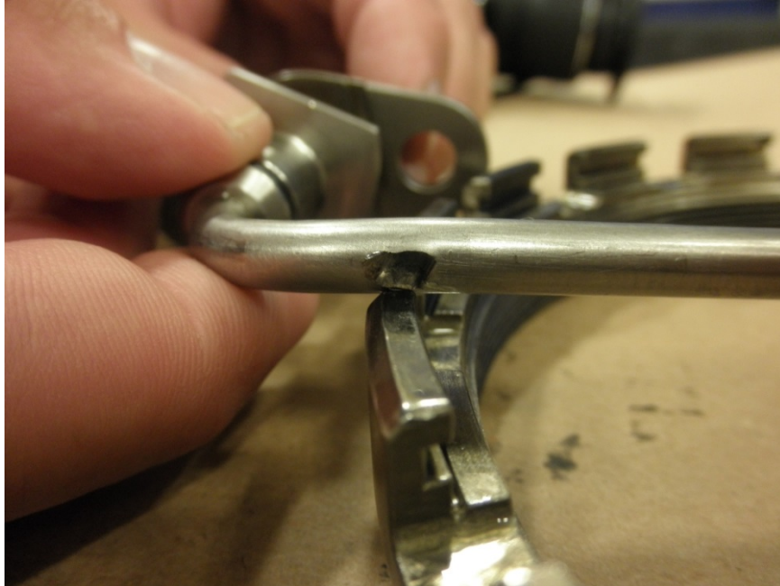
Photo No. 37: Close up of groove in side of No. 5 bearing oil jet that corresponded to the No. 5 bearing retaining nut wrenching lugs.
