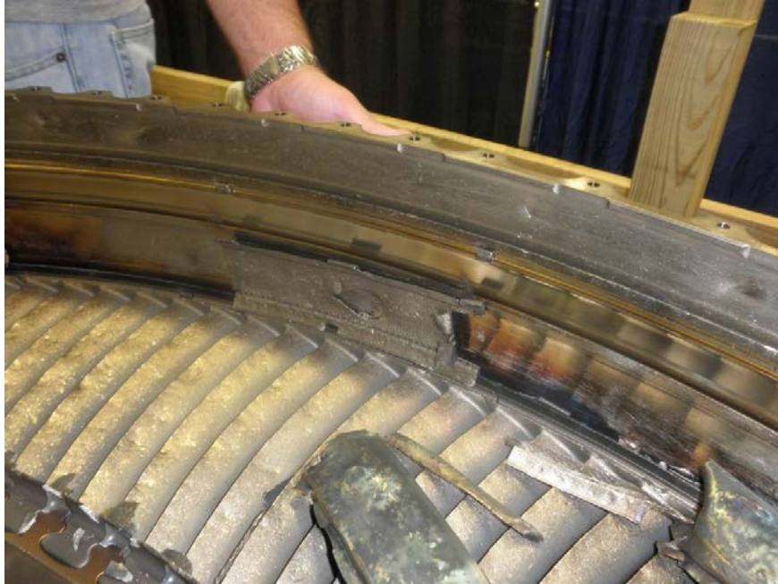
Photo No. 31: View of LPT stage 6 LPT nozzles showing battered airfoils.
