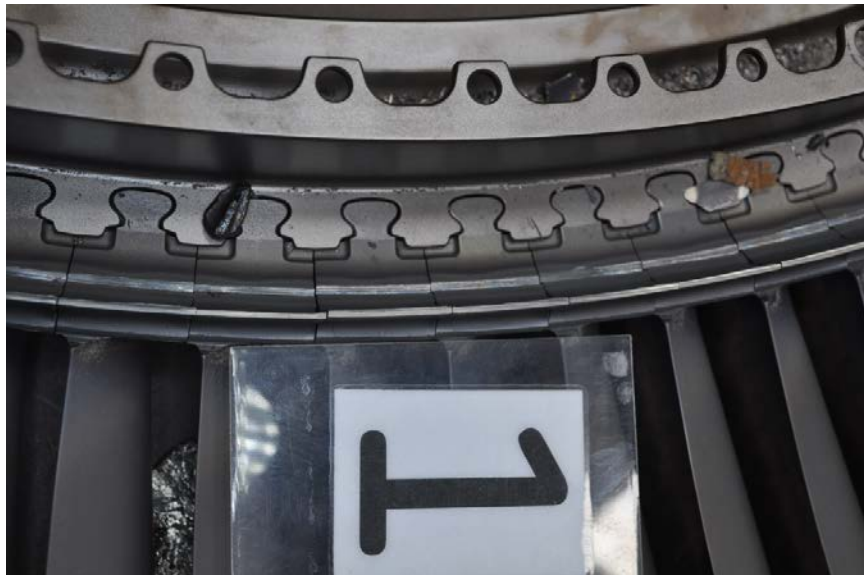
Photo No. 20: Close up view of rear of LPT stage 1 blade roots showing circumferential rub marks on rear face of blade root and on edge of rear angel wing. (GE)
