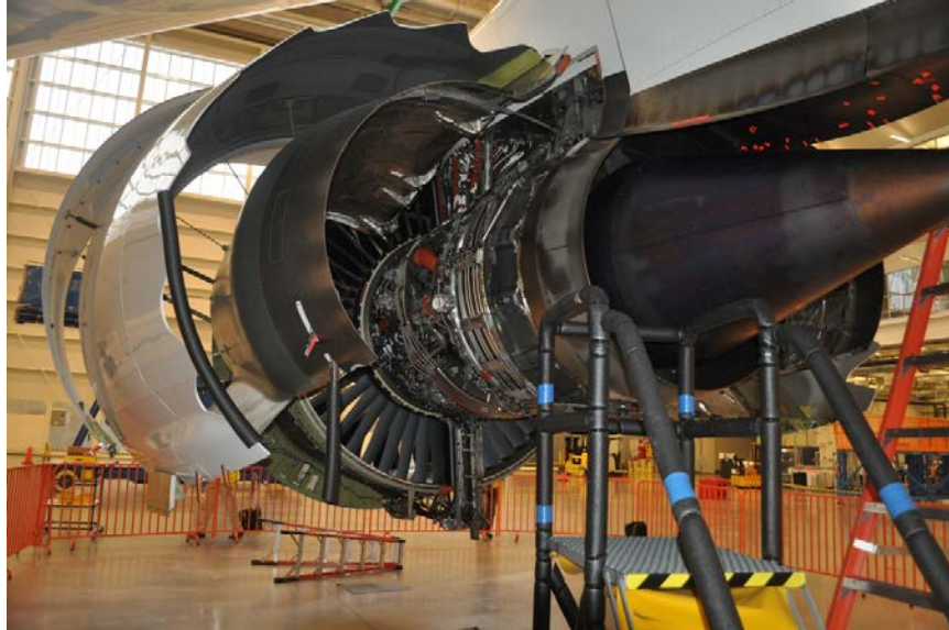
Photo No. 9: Left side of engine with cowls open showing no damage to the inner surfaces of the cowls and no soot or fire damage to the engine. (GE)
