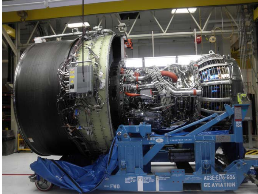
Photo No. 12: Left side of engine showing no uncontainments, case ruptures, or fire damage.
