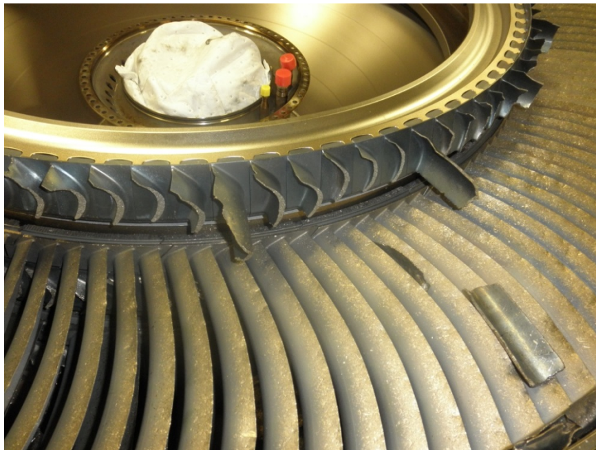
Photo No. 34: View of LPT stage 7 disk showing it is intact and that all of the blades are in place, but fractured at various lengths above the blade root platform.
