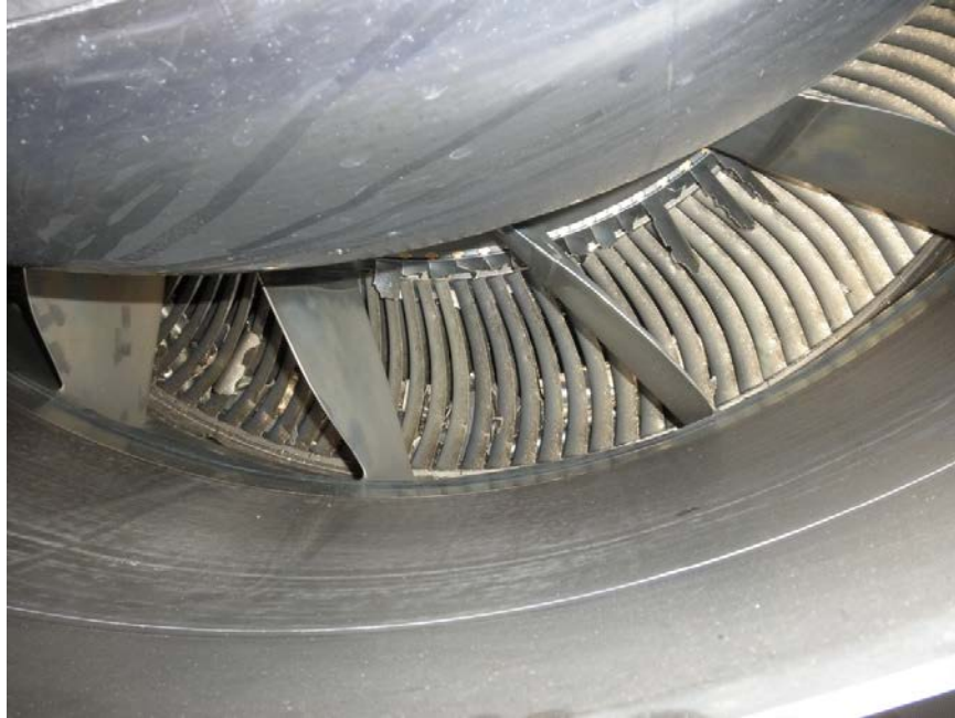
Photo No. 11: View of LPT stage 7 nozzles showing broken airfoil pieces in front of the nozzle airfoils and broken LPT stage 7 blades.
