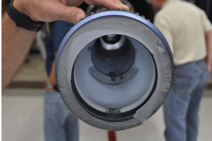
Photo No. 5: Close up of fractured forward end of fan mid shaft showing two areas with different gray colorations. (GE)
