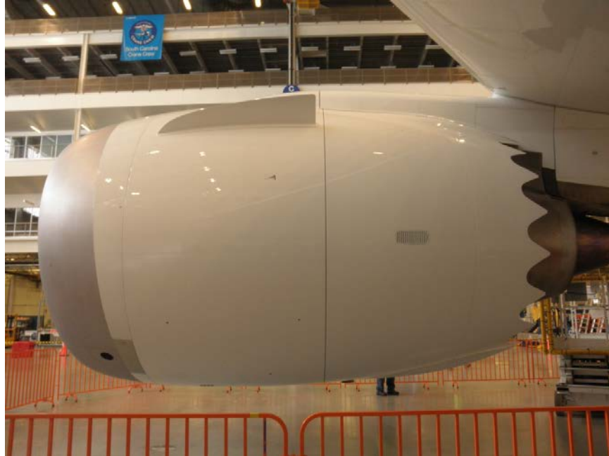
Photo No. 7: Left side of engine cowl showing no damage or heat distress.
