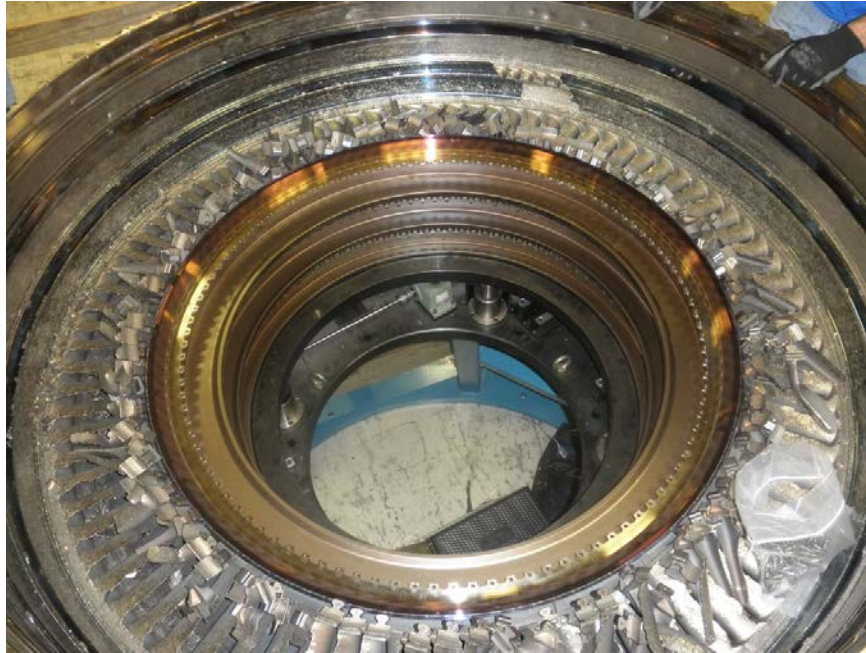
Photo No. 29: View of LPT stage 4 disk showing it is intact. (All of the LPT stage 4 blades had fallen out of the disk while the rotor was being disassembled.) Also shown is all of the LPT stage 4 LPT shroud segments missing except one and all of the LPT stage 5 nozzles missing except one. Also shown is all of the LPT stage 5 shroud segments missing.
