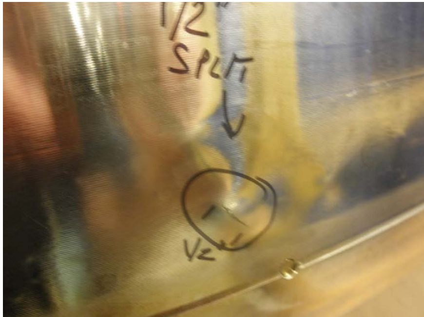
Photo No. 18: Close up of approximately 0.5-inch long split in LPT case at about 6 o'clock.
