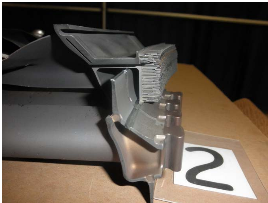
Photo No. 23: Close up view of LPT stage 2 blades and stage 3 nozzles showing contact points that corresponded with circumferential rub marks on each piece.
