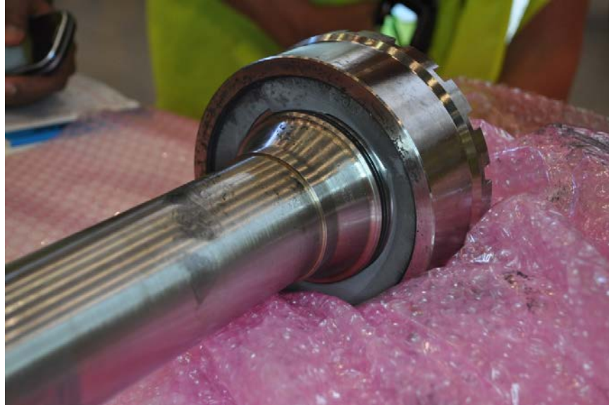
Photo No. 2: View of fractured forward end of fan mid shaft in retaining nut with center vent tube after removal from engine. (GE)
