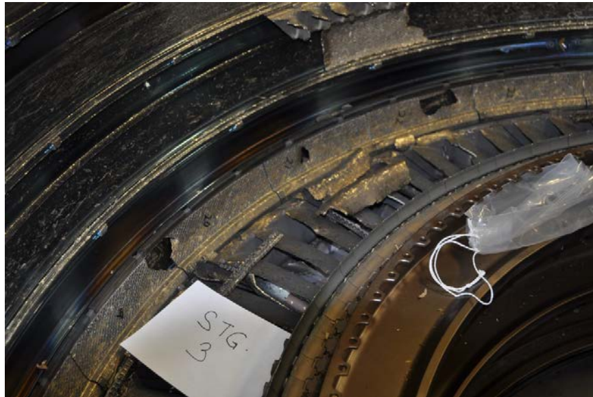
Photo No. 27: Close up view of LPT stage 3 shroud segments showing holes through several segments.
