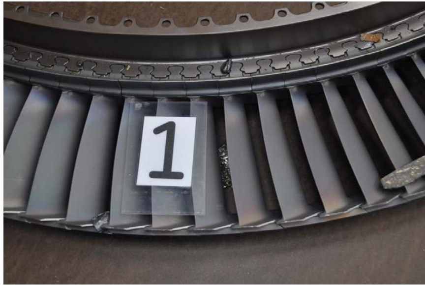
Photo No. 19: View of LPT stage 1 disk and blades showing no damage. (GE)
