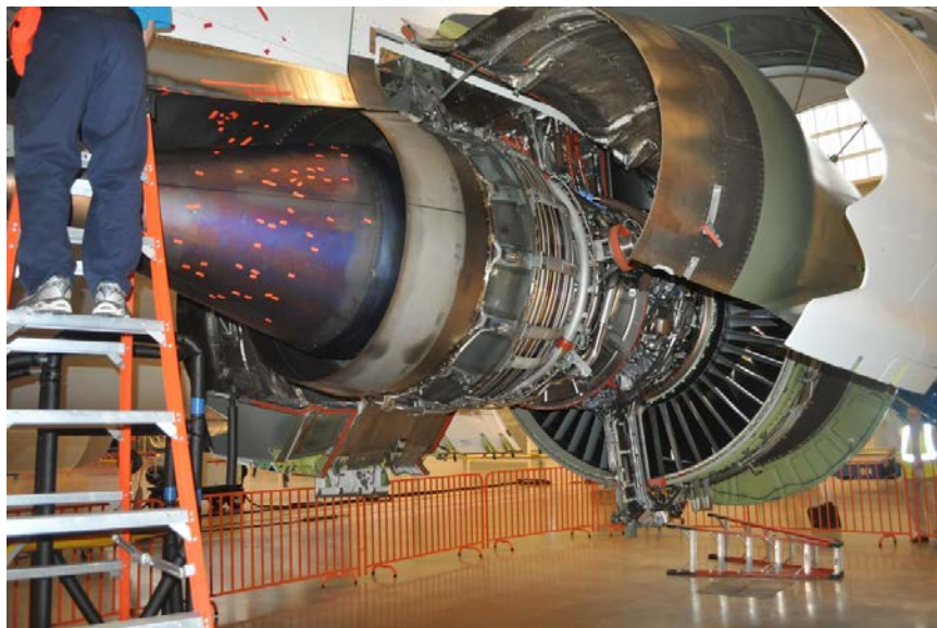
Photo No. 10: Right side of engine with cowls open showing no damage to the inner surfaces of the cowls and no soot or fire damage to the engine. The red pieces of tape mark the impact marks on the tailcone. (GE)
