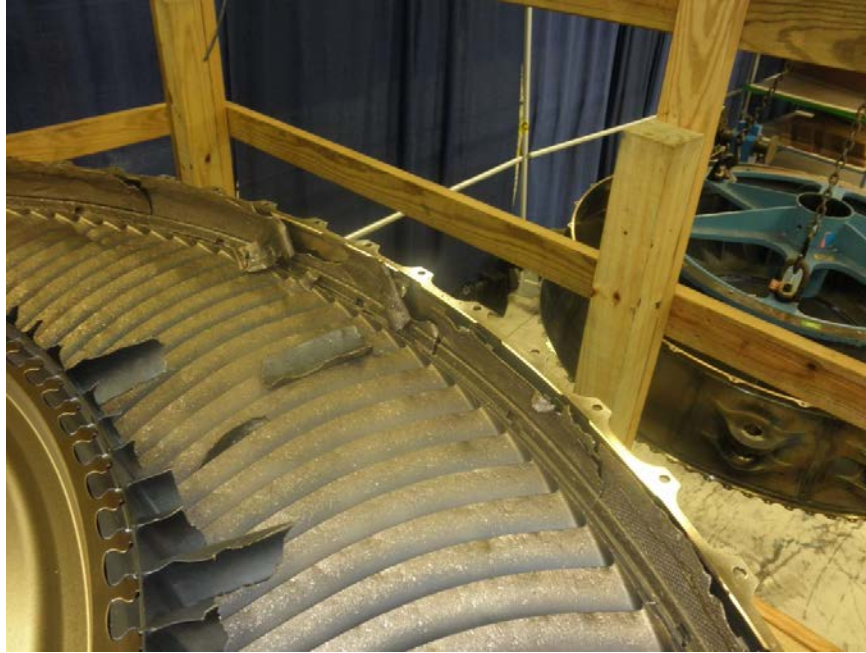
Photo No. 33: View of LPT stage 7 nozzles showing battered airfoils. Also shown are the LPT stage 7 shrouds in place in the case with the honeycomb rubbed down to the backing plate.
