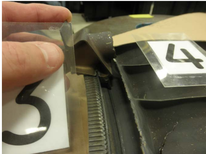
Photo No. 26: Close up view of LPT stage 3 blade and stage 4 nozzle showing contact points that corresponded to rub marks on each component.
