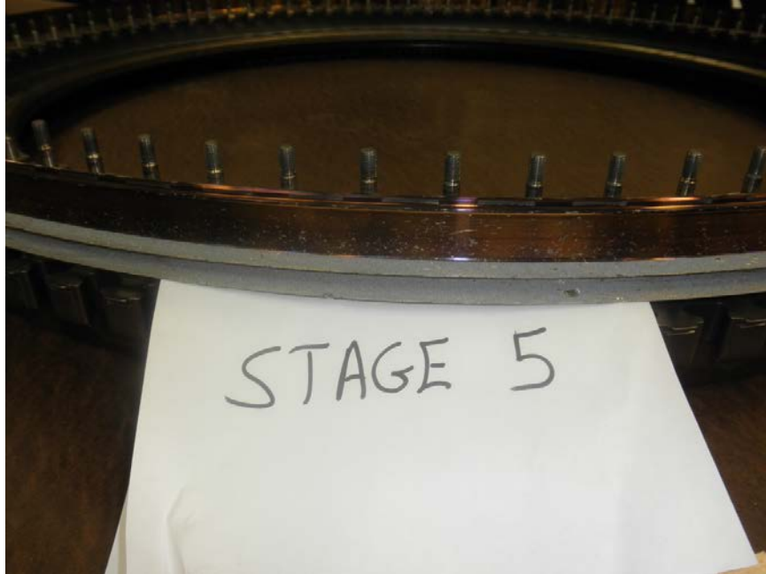
Photo No. 30: Close up of LPT stage 5 disk showing impact marks on outer diameter and chips on coating on knife edge seals.
