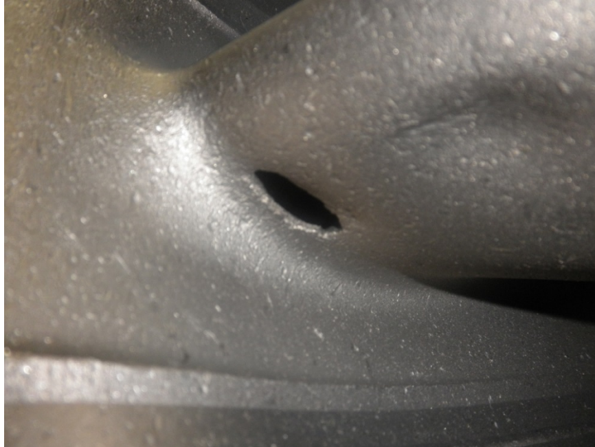
Photo No. 36: Close up view of hole in turbine rear frame strut.
