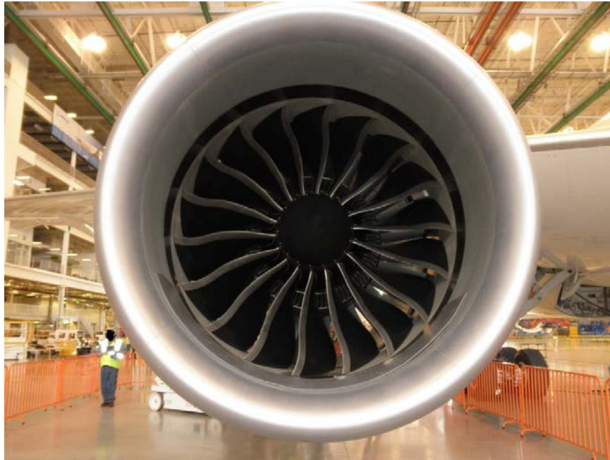
Photo No. 6: View of engine's inlet lip and duct showing no damage. Also shown are the fan blades with no damage or marks.
