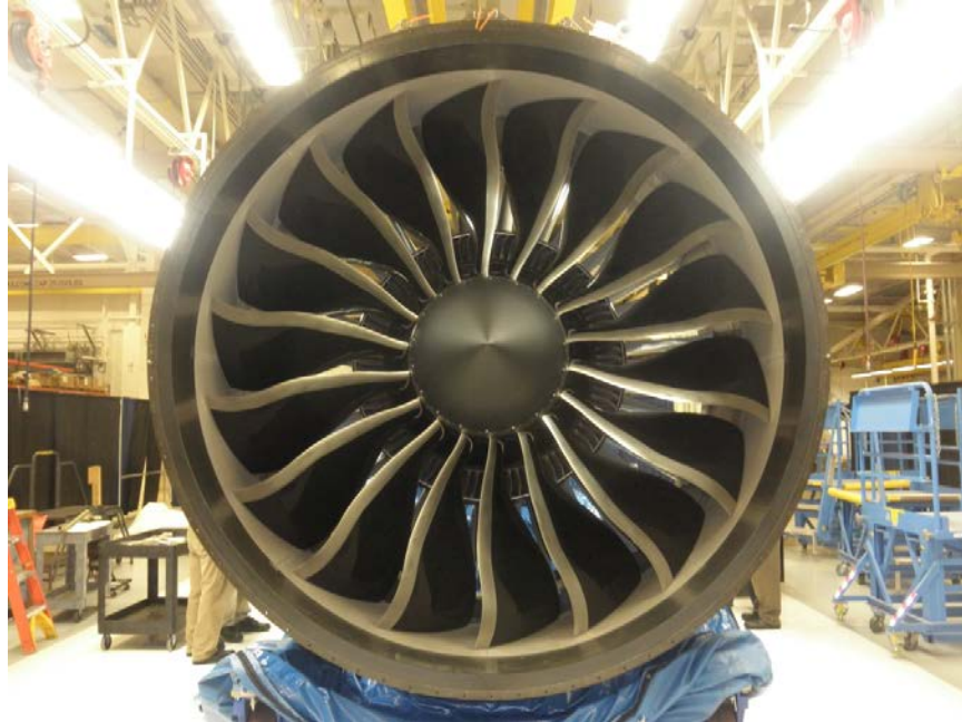
Photo No. 14: View of fan blades showing all are present and undamaged. Also shown is the fan blade rub strip showing no circumferential rub marks.
