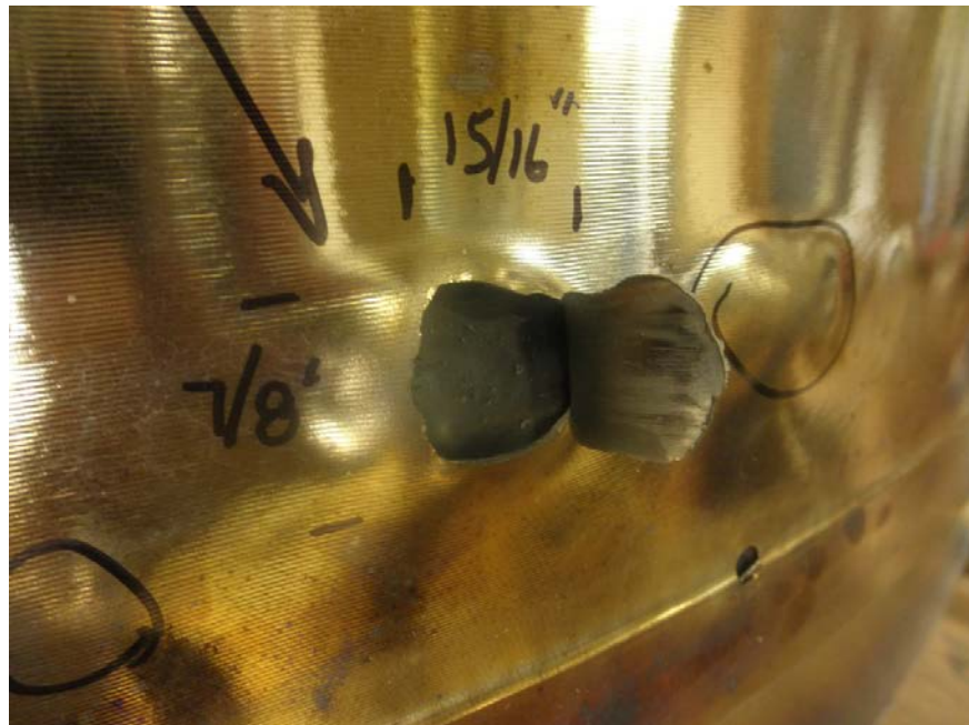
Photo No. 16: Close up of hole in LPT case.
