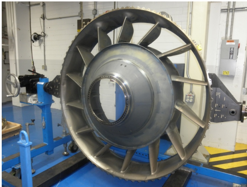
Photo No. 35: View of turbine rear frame showing that it is intact.
