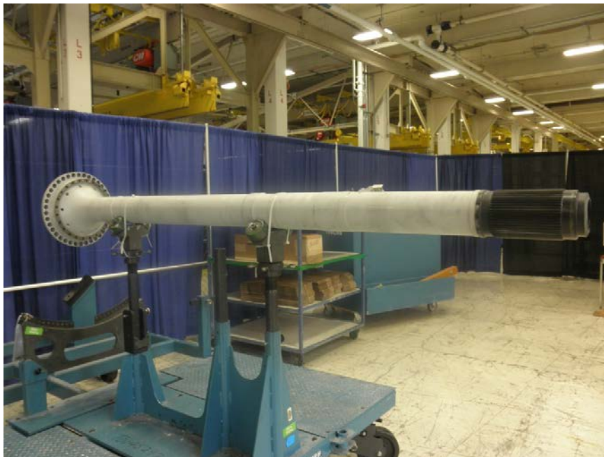
Photo No. 4: Fractured fan mid shaft.
