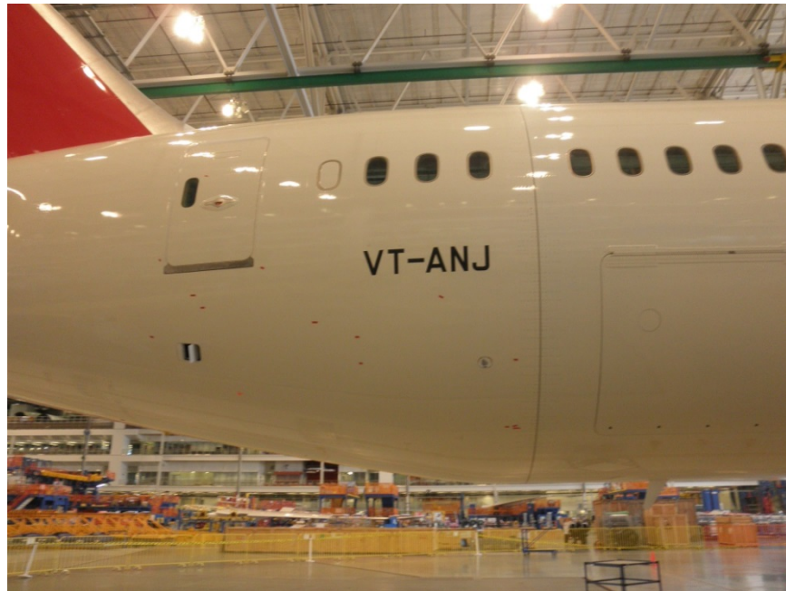
Photo No. 39: View of right side of aft fuselage with red tape showing impact marks.
