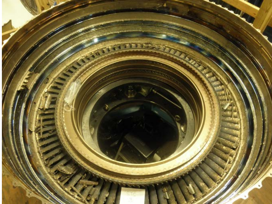
Photo No. 25: View of LPT stage 3 disk showing it is intact and all of the LPT stage 3 blade roots are in place. Also shown are all of the LPT stage 3 nozzles and LPT stage 3 shroud segments are in place in the LPT case.
