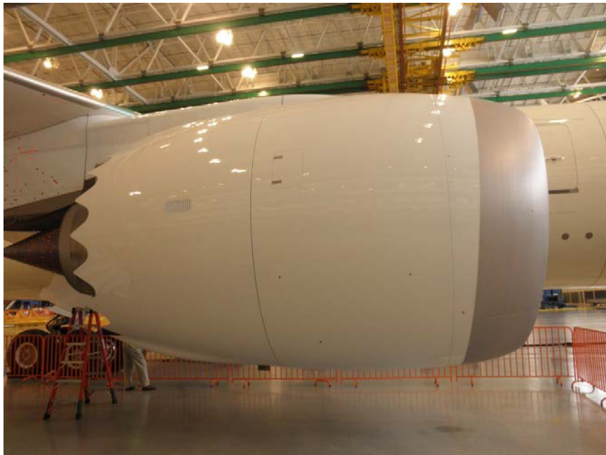
Photo No. 8: Right side of engine cowl showing no damage or heat distress.
