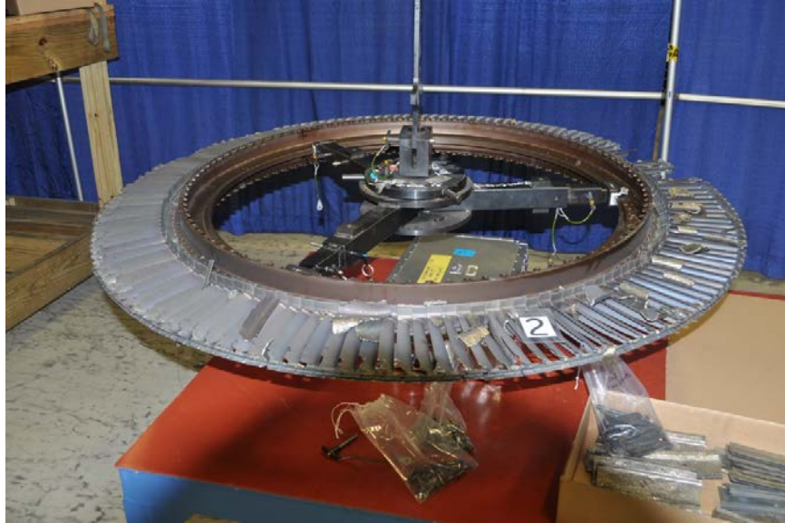
Photo No. 22: View of LPT stage 2 disk and blades after they were removed from the engine showing the disk is intact and all of the blades are in place in the disk.
