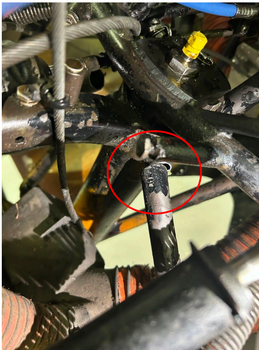
Photograph 2 - Engine mount damage (Courtesy of the FAA)
