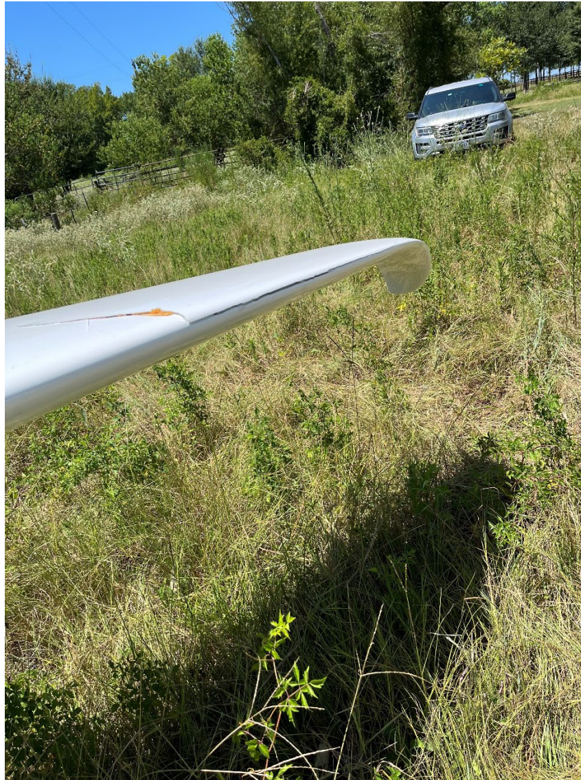
Photograph 2 - Right Wing Damage (Courtesy of Federal Aviation Administration)
