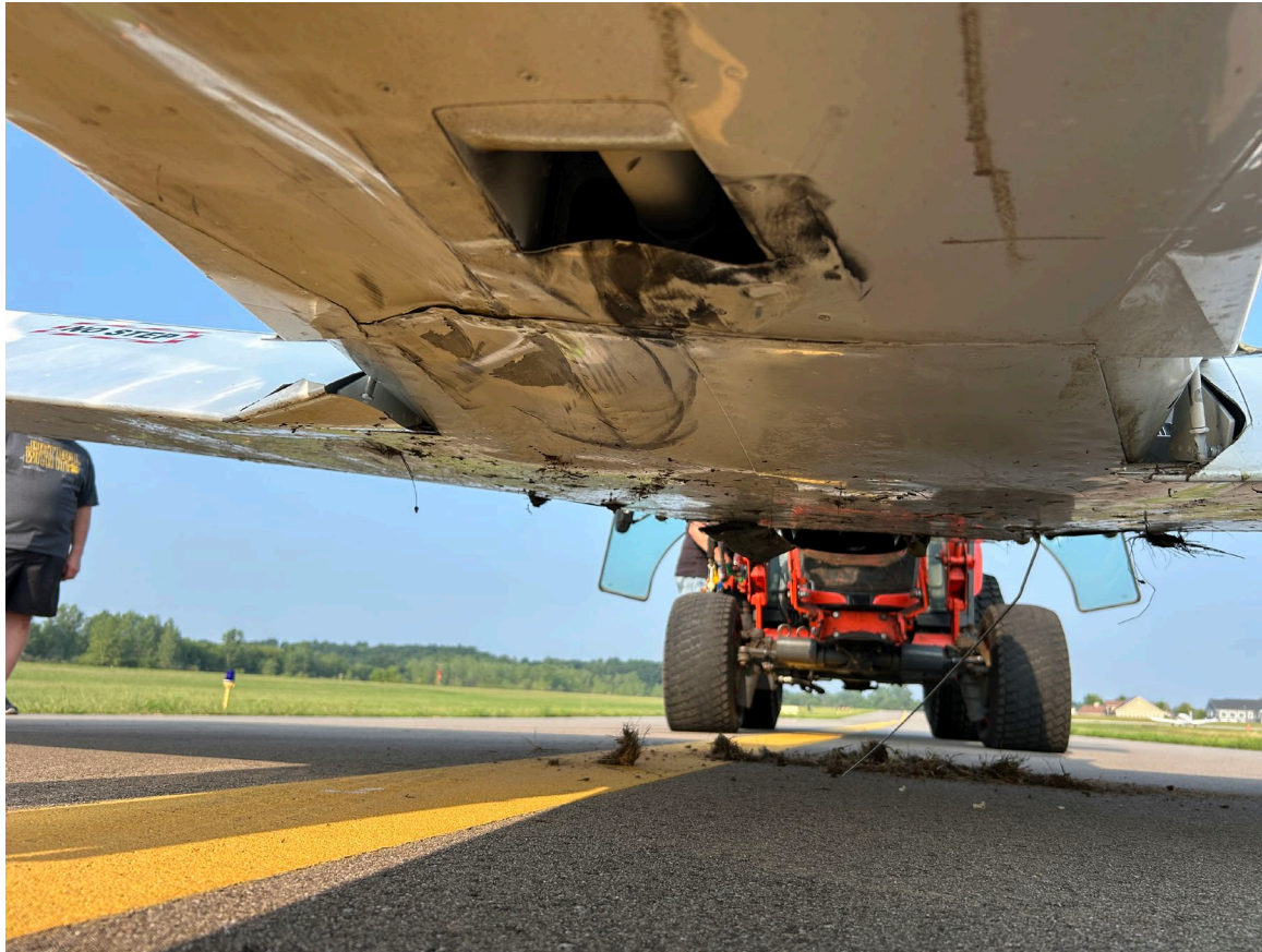
Photograph 1 - AFT Fuselage Damage (Courtesy of the FAA)
