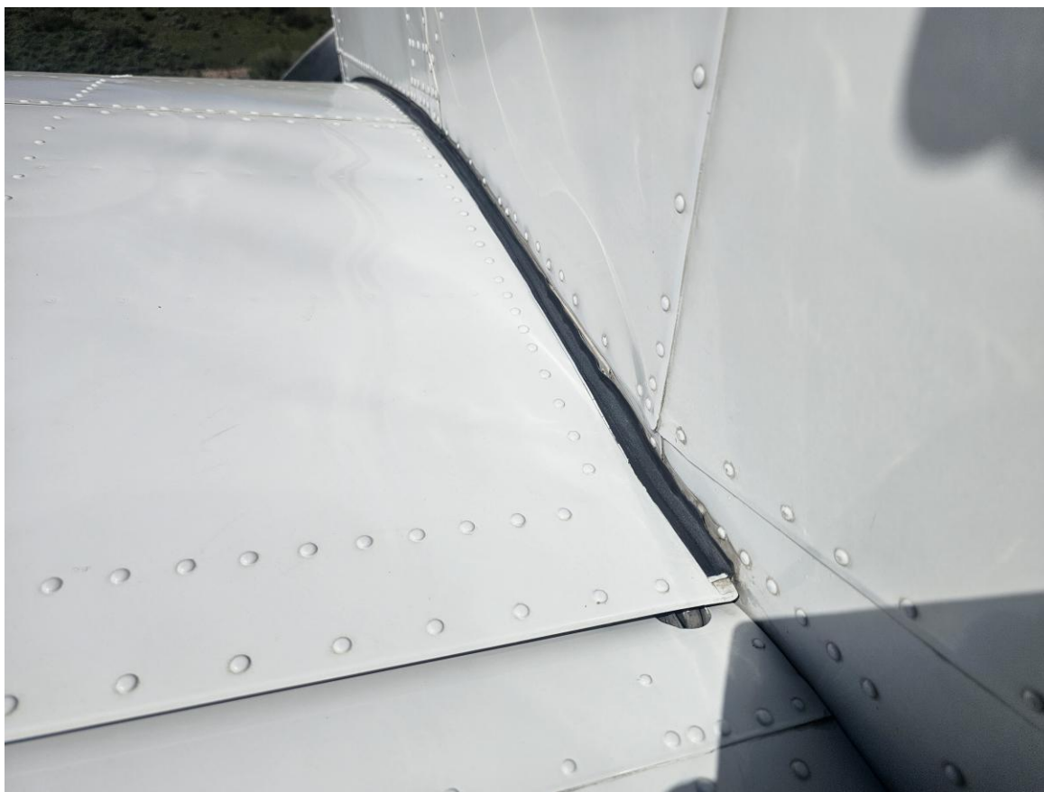
Photograph 2 - Left side fuselage damage at wing root (Courtesy of recovery company)
