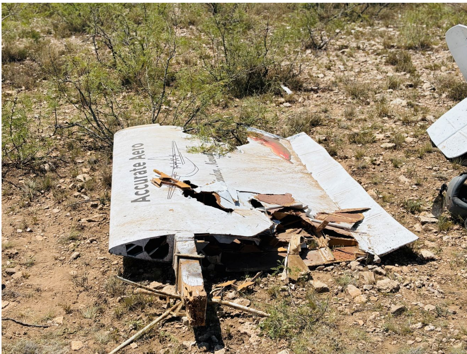
Photograph 6 - View of the right wing at the accident site (courtesy of the Federal Aviation Administration)
