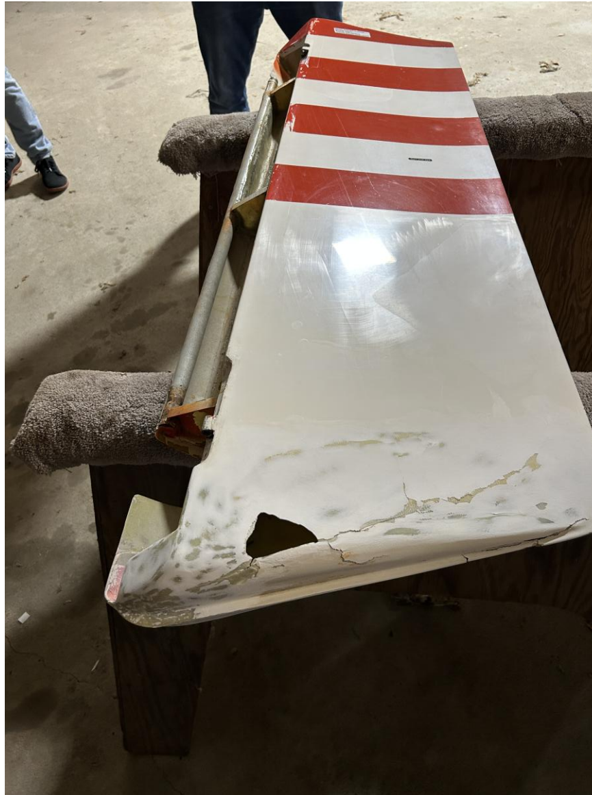
Photograph 2 - Accident glider rudder damage (Courtesy of operator)
