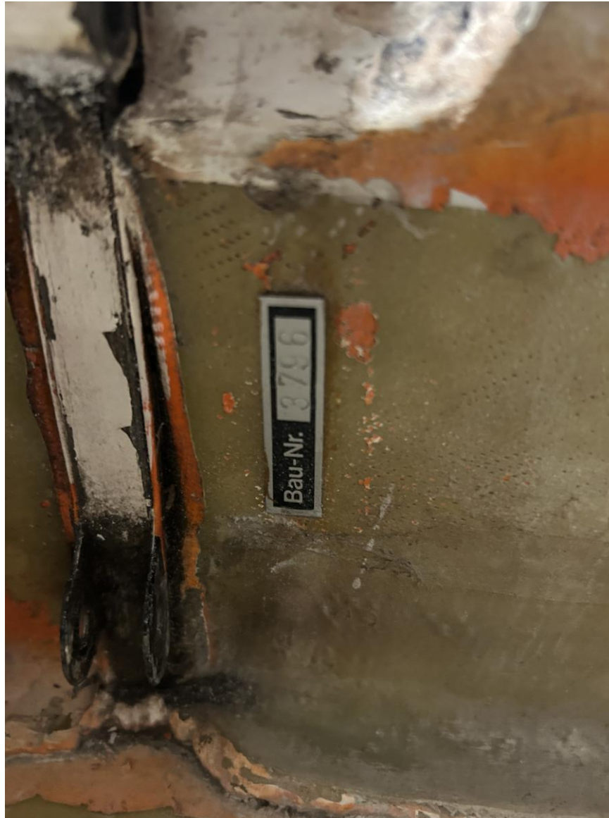
Photograph 3 - Accident glider composite damage (Courtesy of operator)
