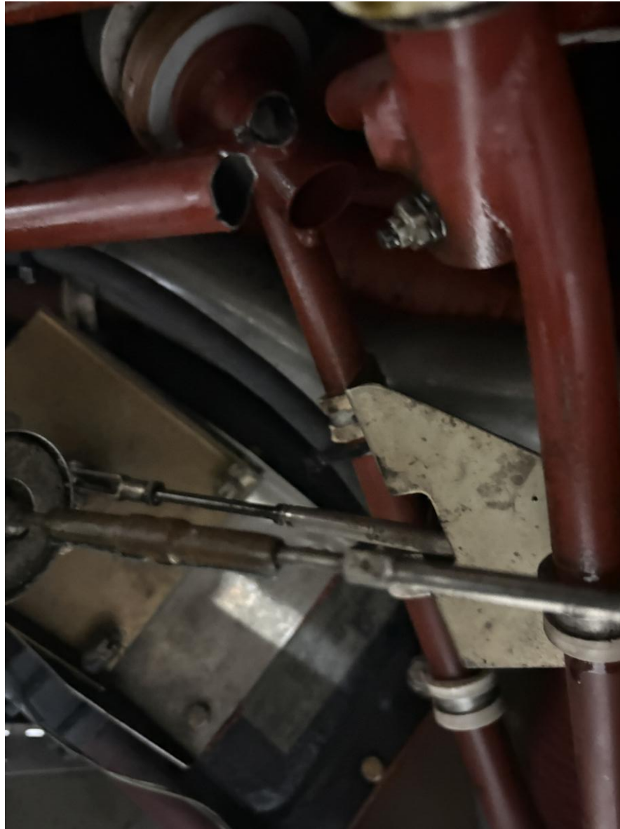
Photograph 1 - Fractured Engine Mount (Courtesy of FAA)
