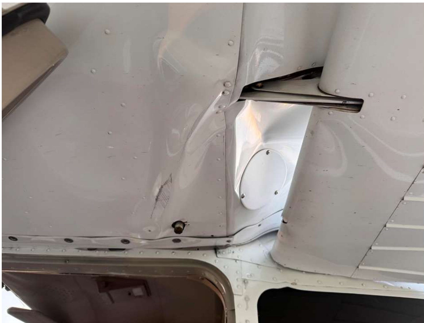
Photograph 3 - Left wing damage
