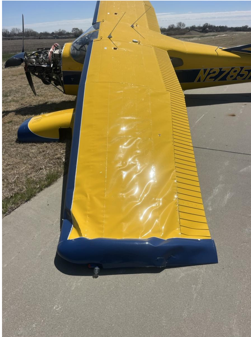
Photograph 2 - Left wing damage (Courtesy of owner)
