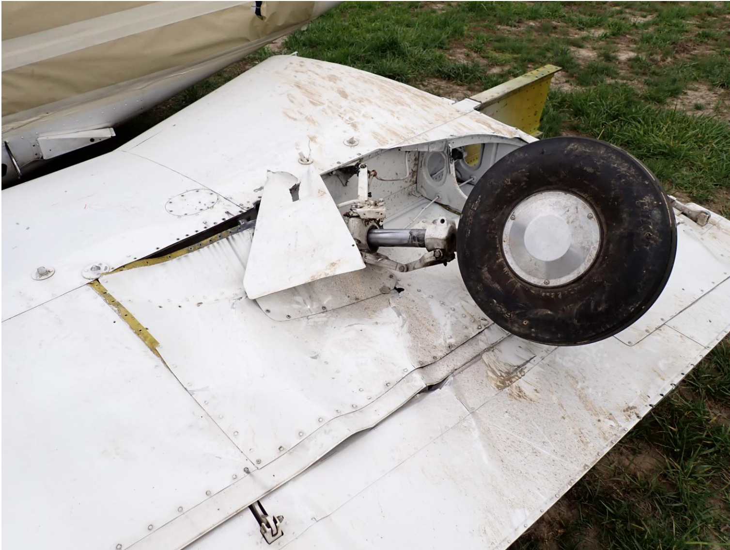
Photograph 2 - Right wing as removed for transport showing wing spar damage (Courtesy of NTSB)
