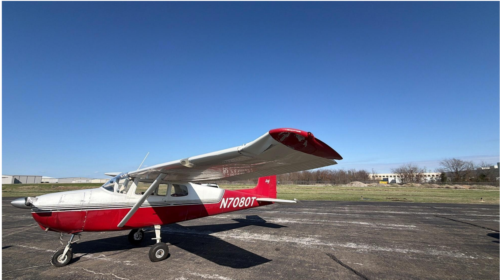
Photograph 2 – Left wing substantial damage (Courtesy of pilot)
