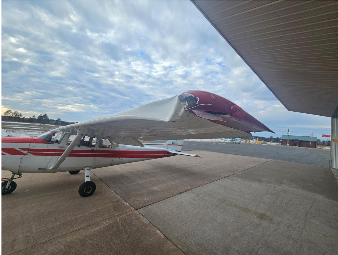
Photograph 2 - Airplane Left wing damage (Courtesy of owner)
