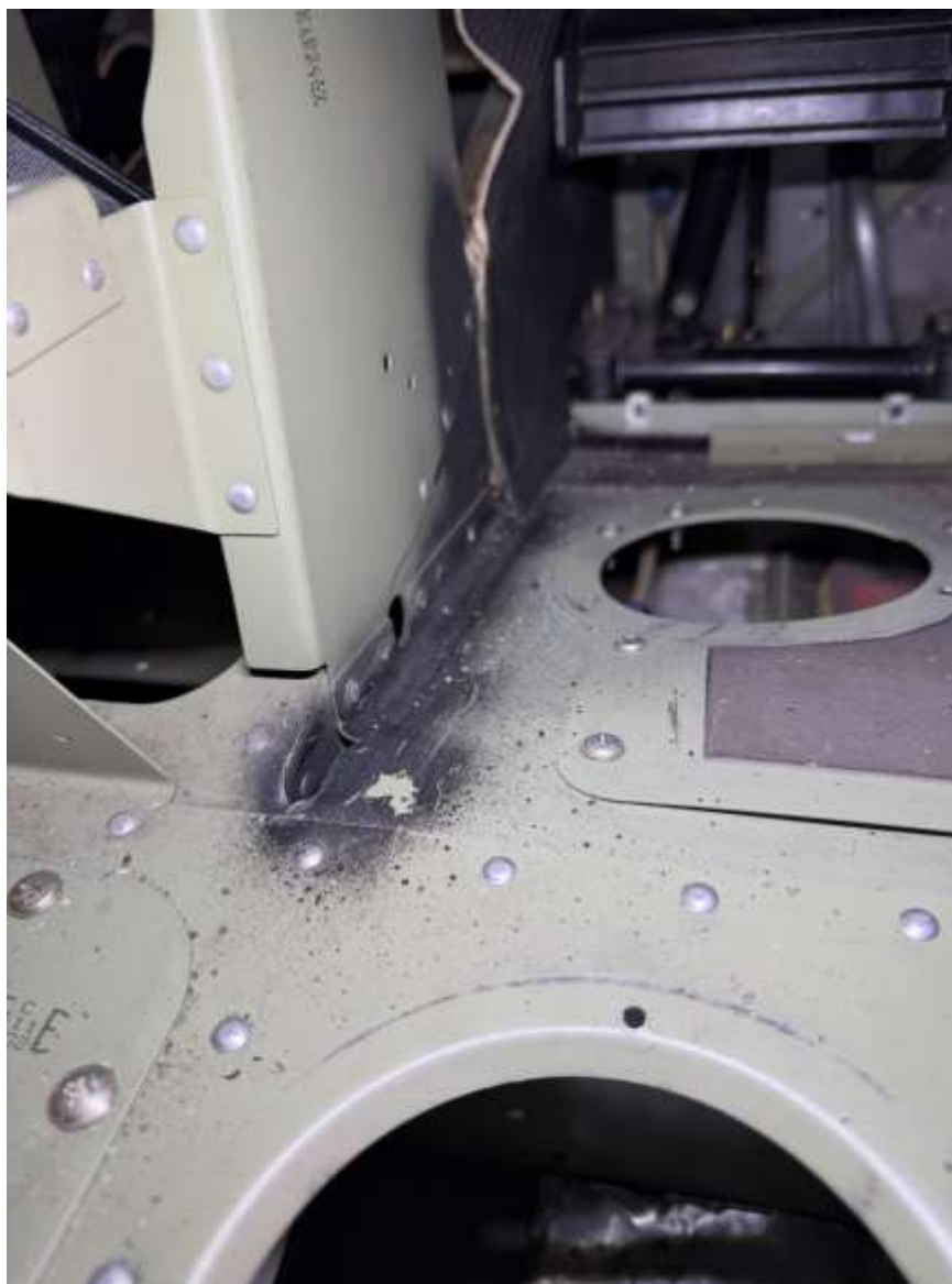
Photograph 2 - Fuselage damage - floor is bowed (Courtesy of pilot)
