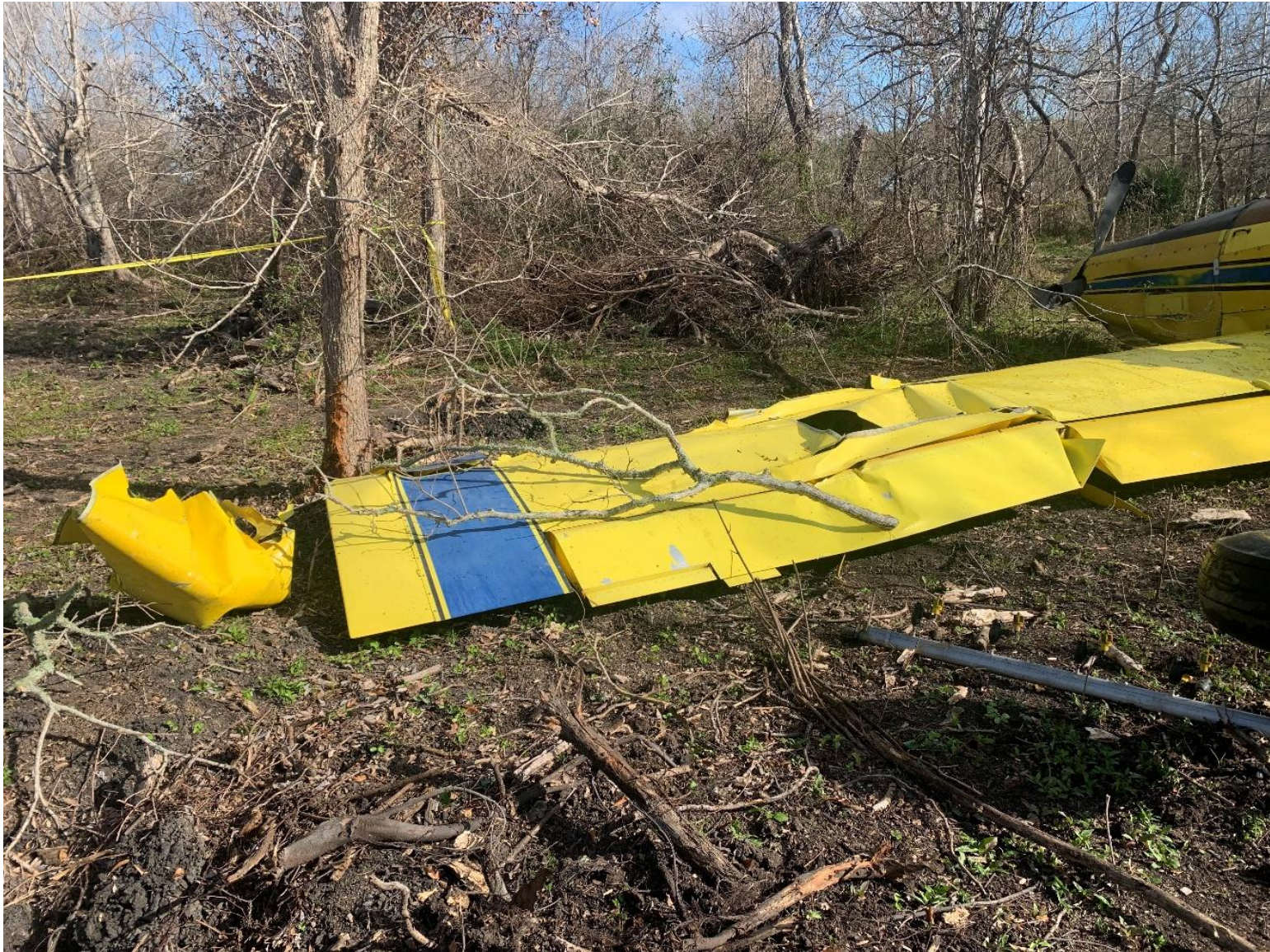
Photograph 4 - View of the left wing at the accident site (courtesy of the Federal Aviation Administration)
