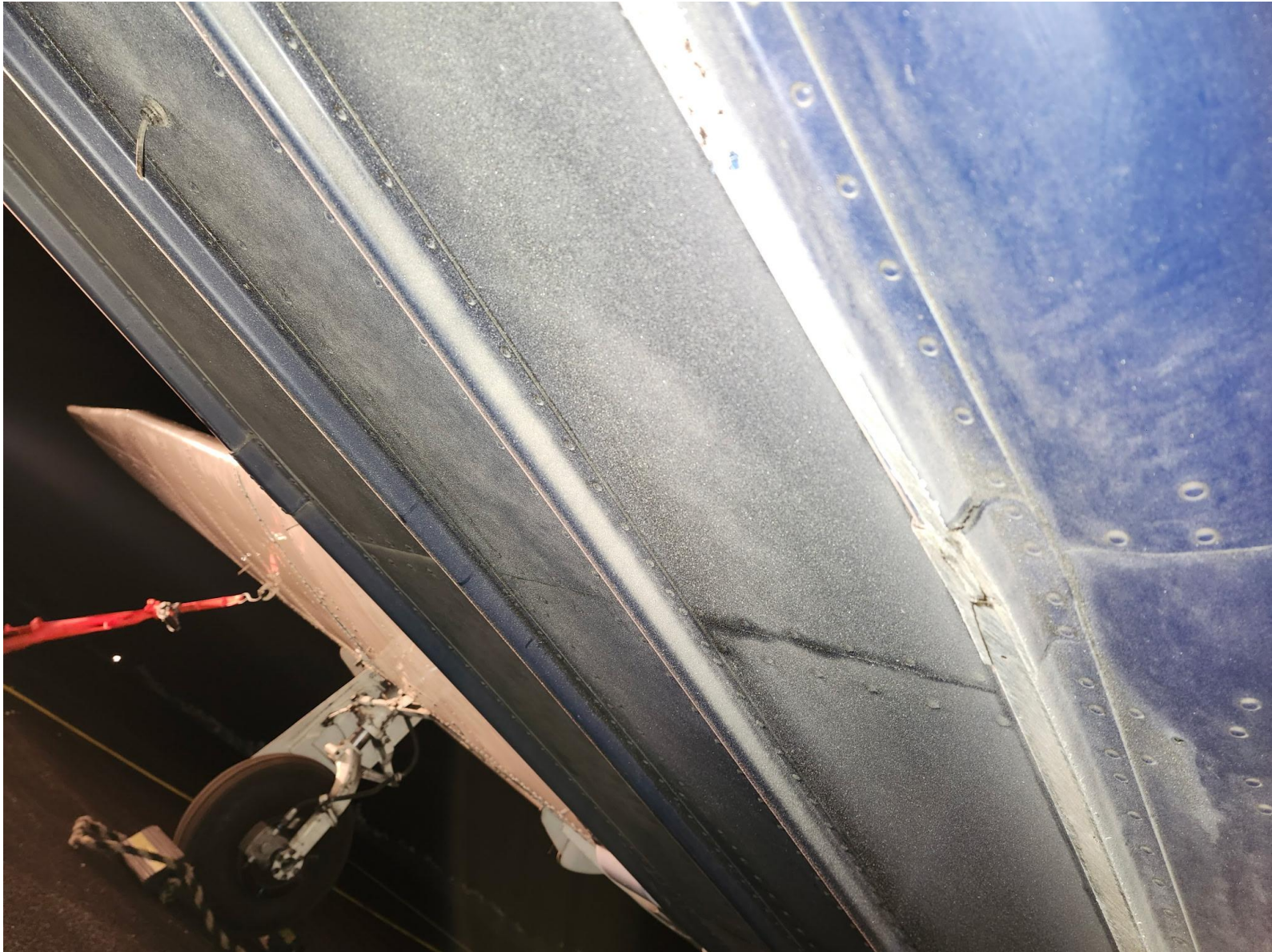
Photograph 2 - Substantially Damaged Longeron (Courtesy of Operator)
