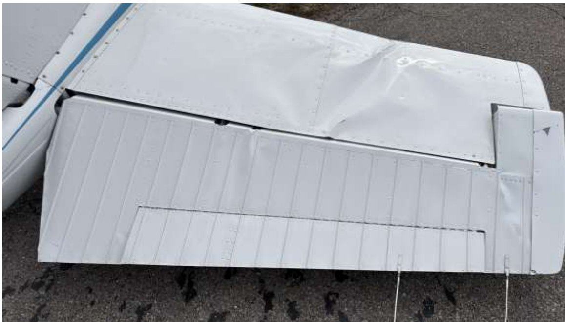
Photograph 2 - Damage to right horizontal stabilizer and elevator (courtesy of operator).
