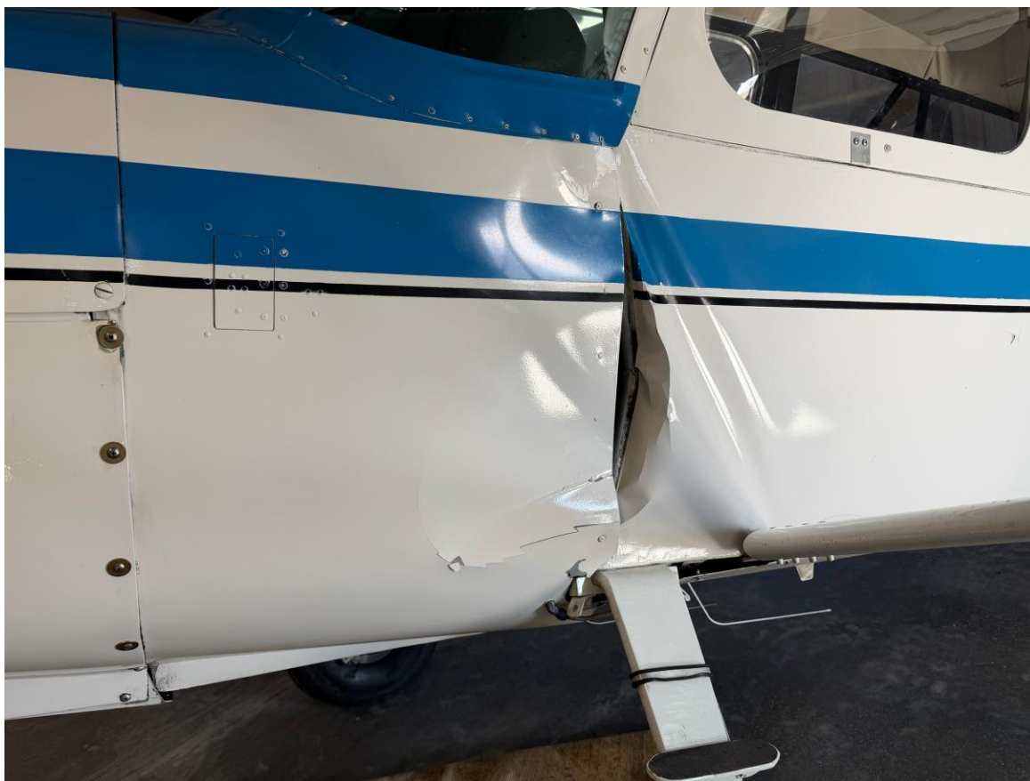
Photograph 3 - Left side fuselage damages (Courtesy of owner)
