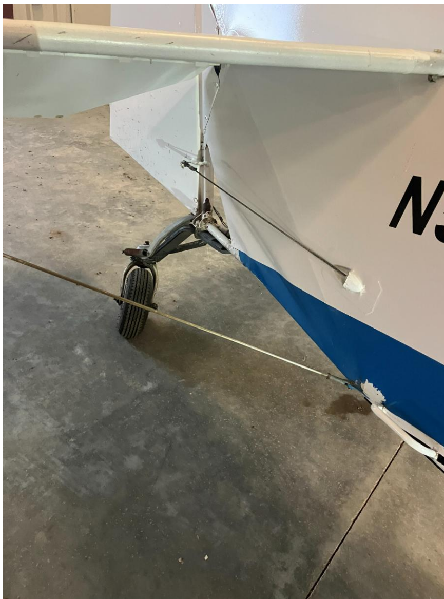
Photograph 4 - Showing bent aft fuselage structure (Courtesy of owner)
