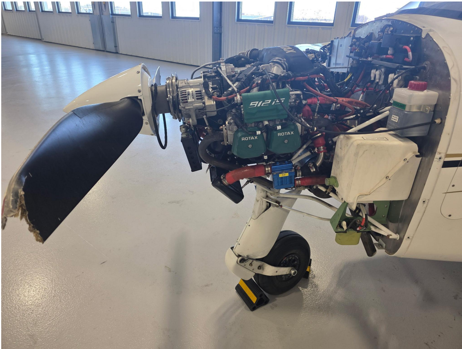
Photograph 5 - Damage includes lower engine mount, propeller, and nose wheel steering rods (Courtesy of director of maintenance)
