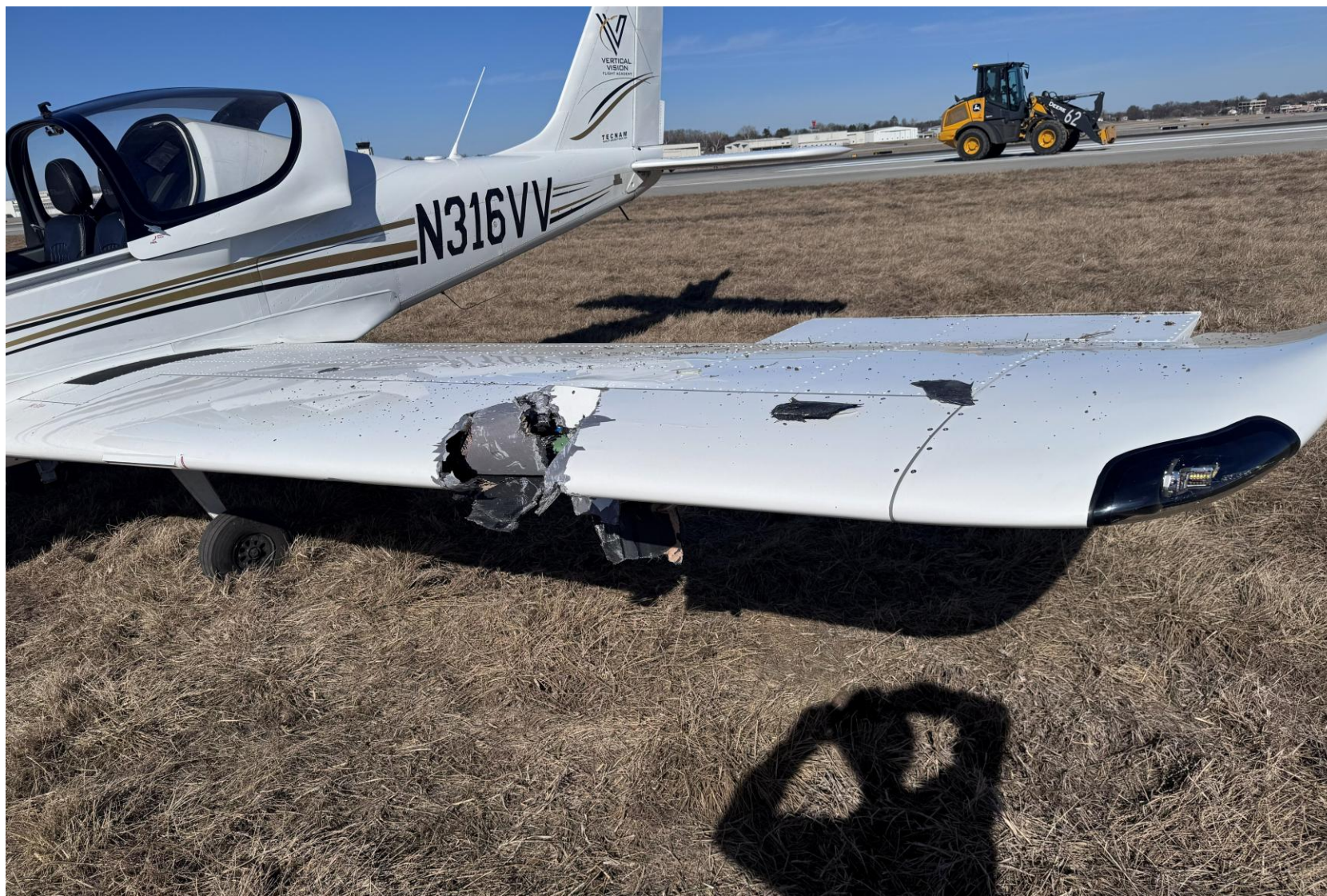
Photograph 3 - Left wing damage (Courtesy of flight school)
