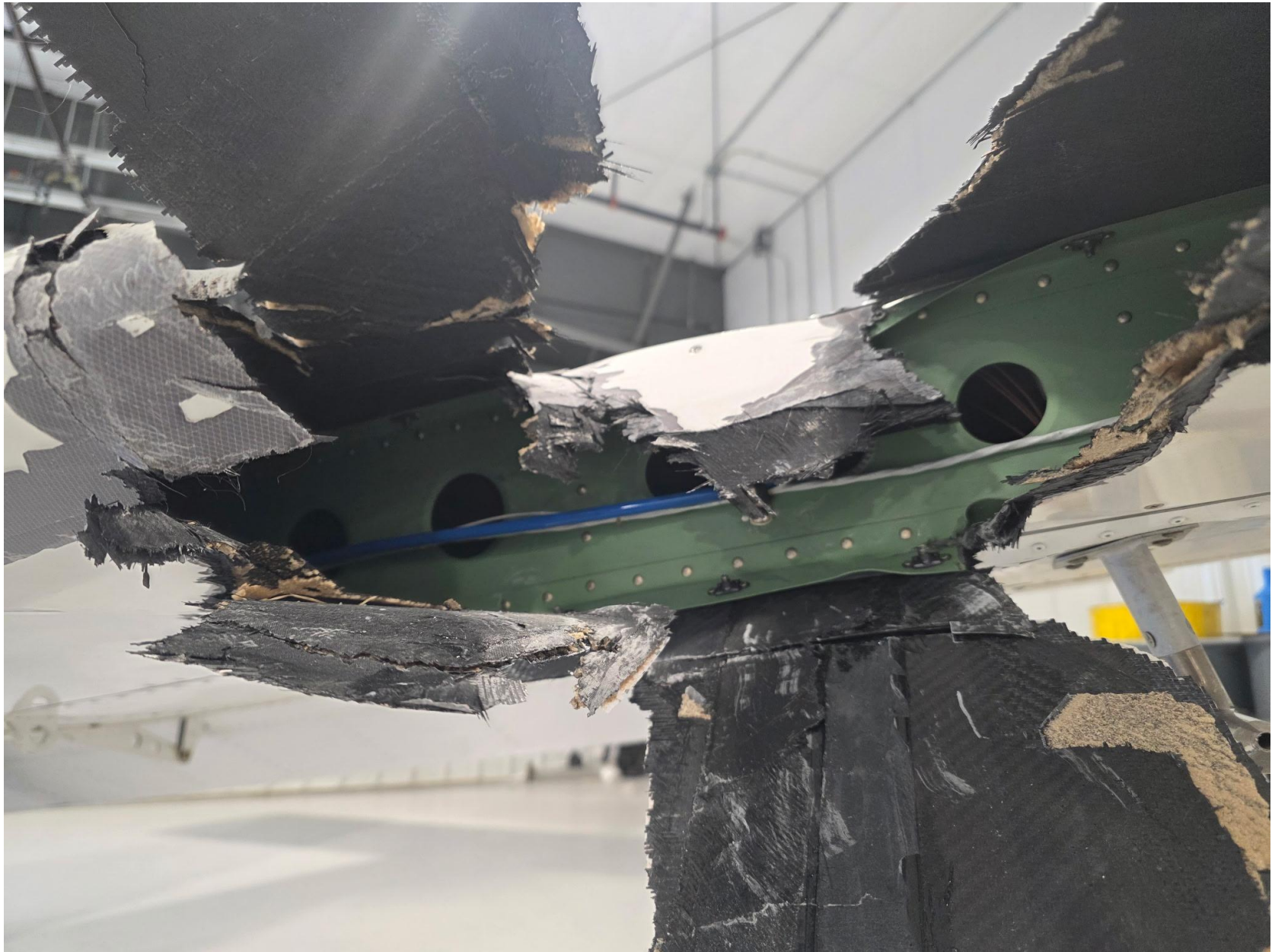
Photograph 4 - Left wing spar damage (Courtesy of director of maintenance)
