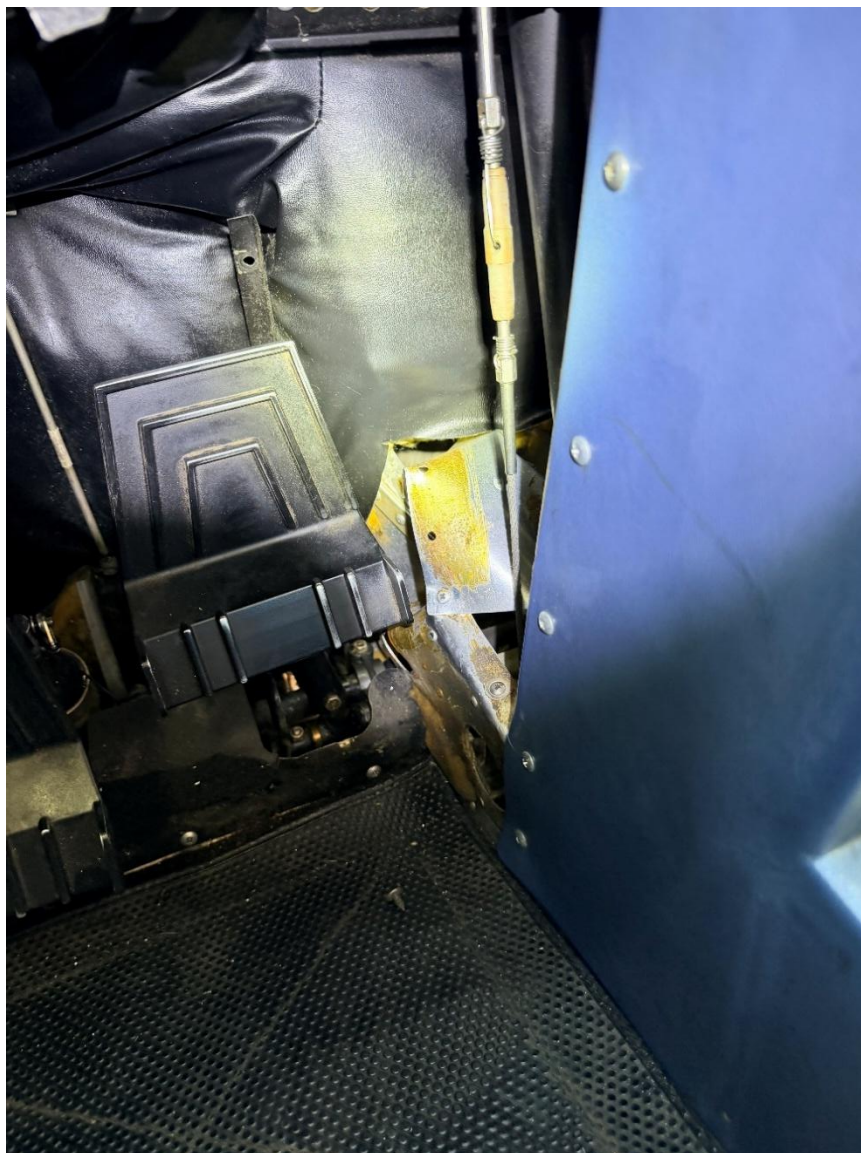
Photograph 1 - View of the substantial damage sustained to the lower fuselage near the cockpit (courtesy of the Federal Aviation Administration)
