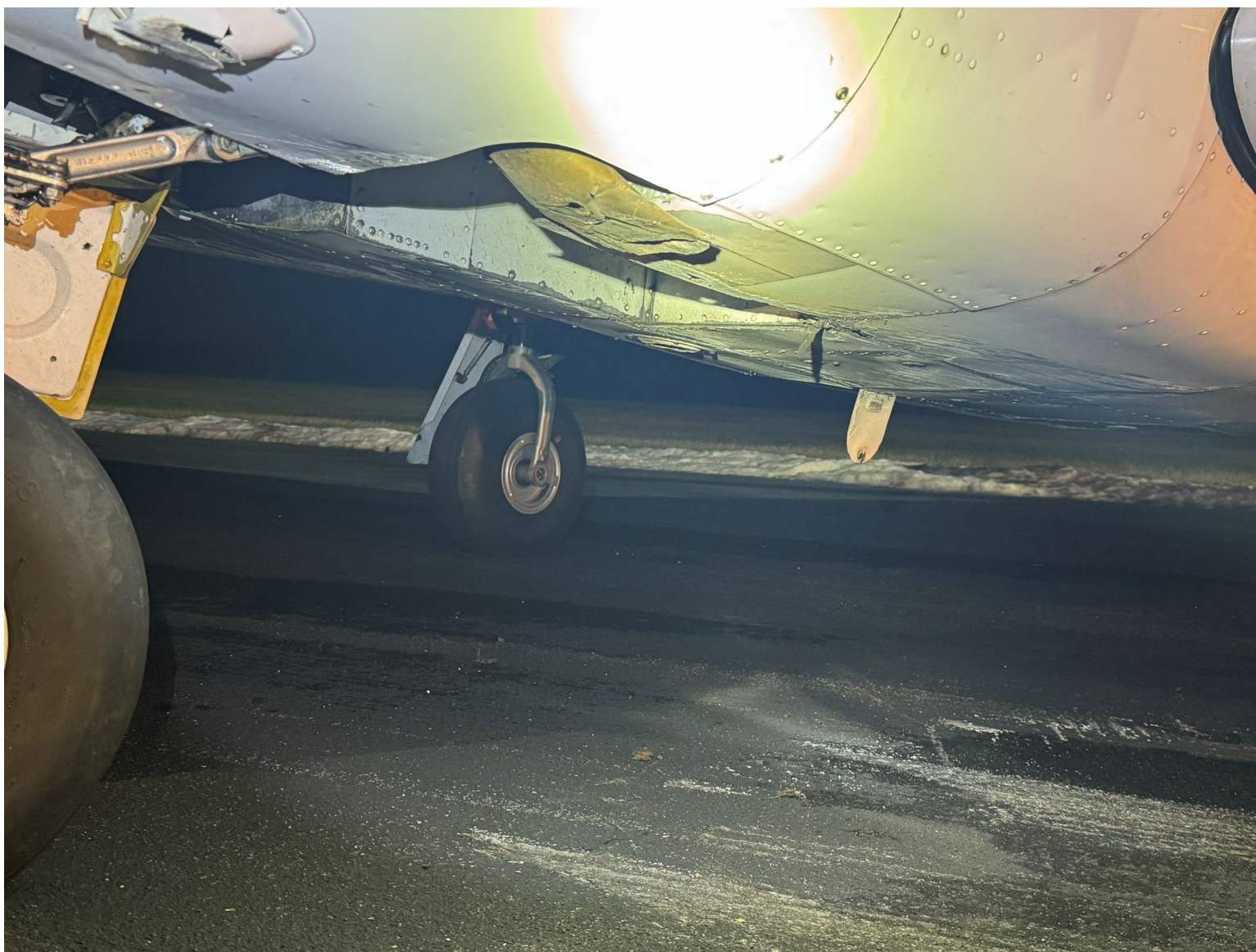
Photograph 3 - Belly damage on accident airplane (Courtesy of owner)
