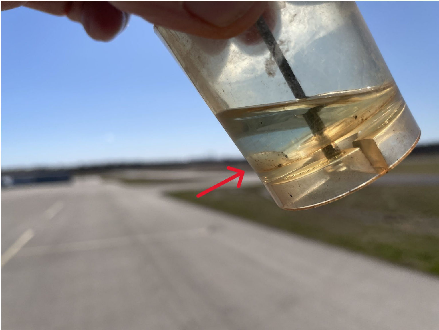
Photograph 5 - View of the fuel sample obtained from the right wing fuel tank. The red arrow shows water contamination (courtesy of the Federal Aviation Administration)
