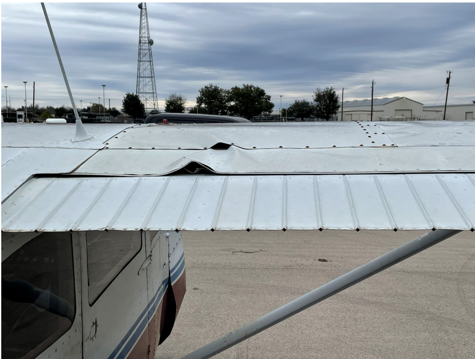
Photograph 4 - View of the substantial damage sustained to the right wing (courtesy of the Federal Aviation Administration)
