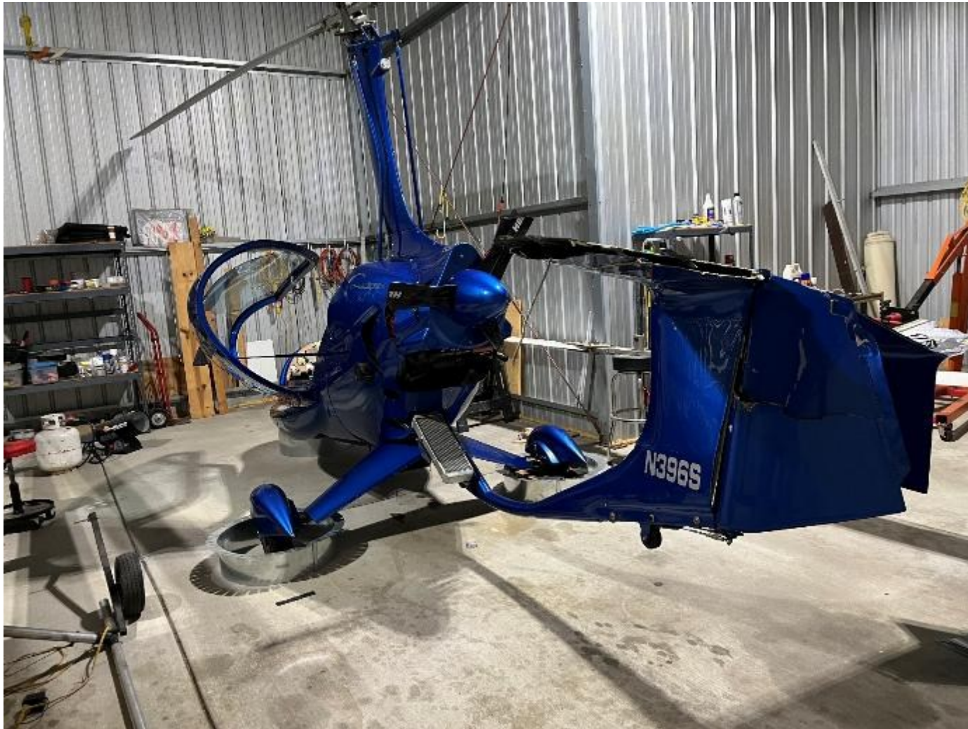
Photograph 3 - Empennage damage (Courtesy of FAA)
