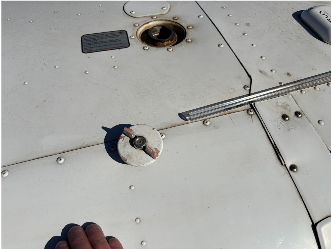
Picture 5 Right Fuel Tank Vented Fuel Cap (Courtesy of the FAA)
