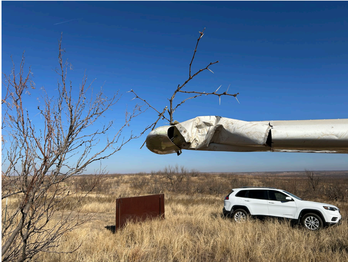
Picture 2 Damage to Outer Right Wing (Courtesy of the FAA)
