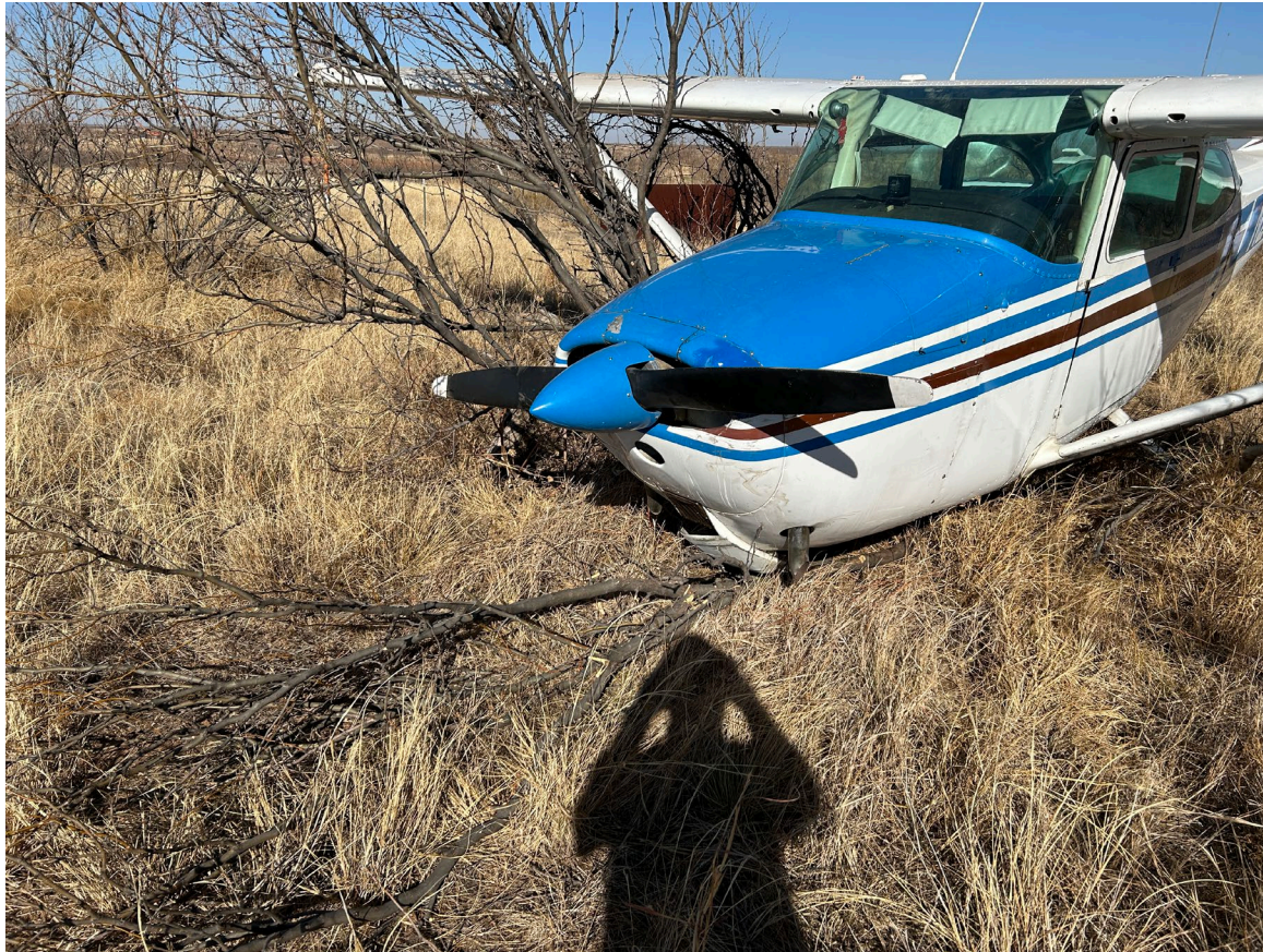
Picture 3 Collapsed Nose Landing Gear (Courtesy of the FAA)
