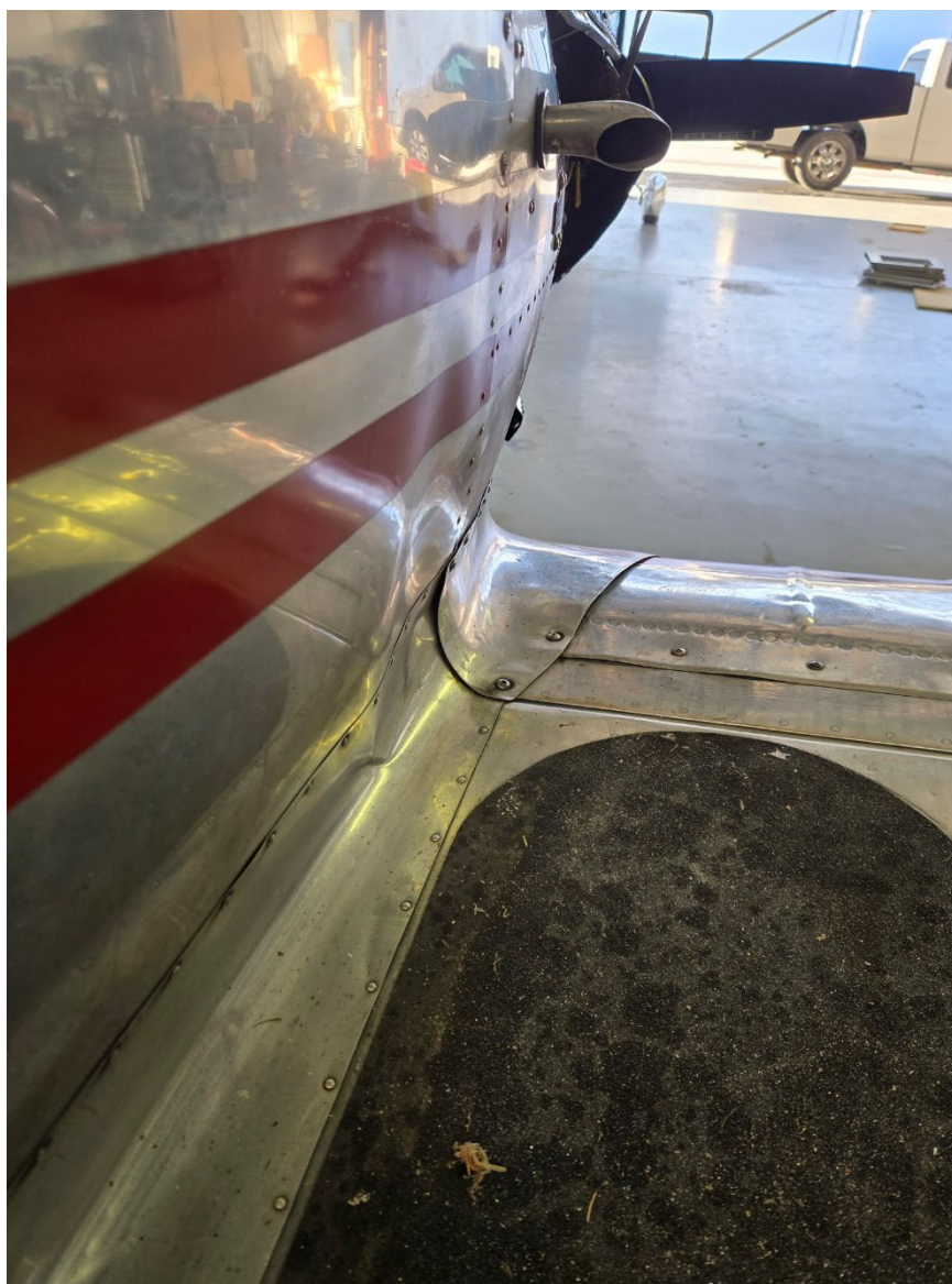
Photograph 1 - Fuselage and Wing Damage (Courtesy of Owner)
