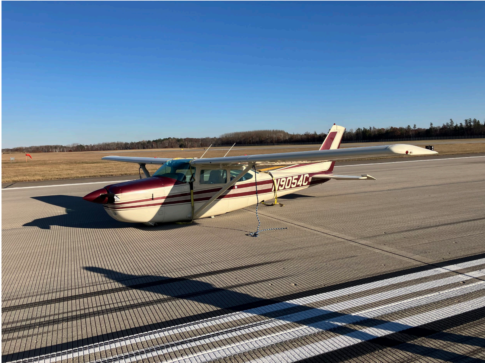
Photograph 1 - Airplane on the runway with gear retracted (Courtesy of FAA)
