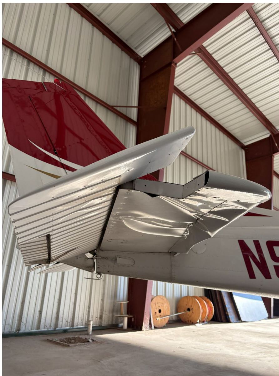
Photograph 3 - View of the bottom of the right side horizontal stabilizer (courtesy of the pilot)
