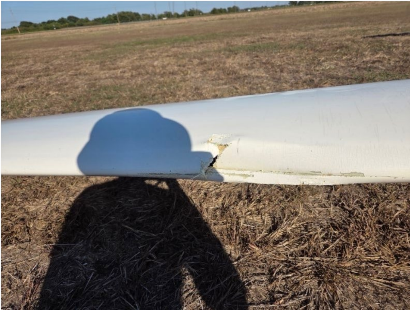
Photograph 2 - N137SS Damage (Courtesy of Greater Houston Soaring Association)
