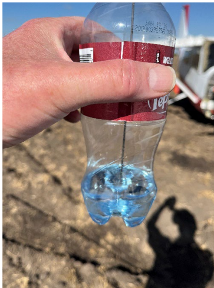
Figure 1 Fuel From the Left Fuel Tank
