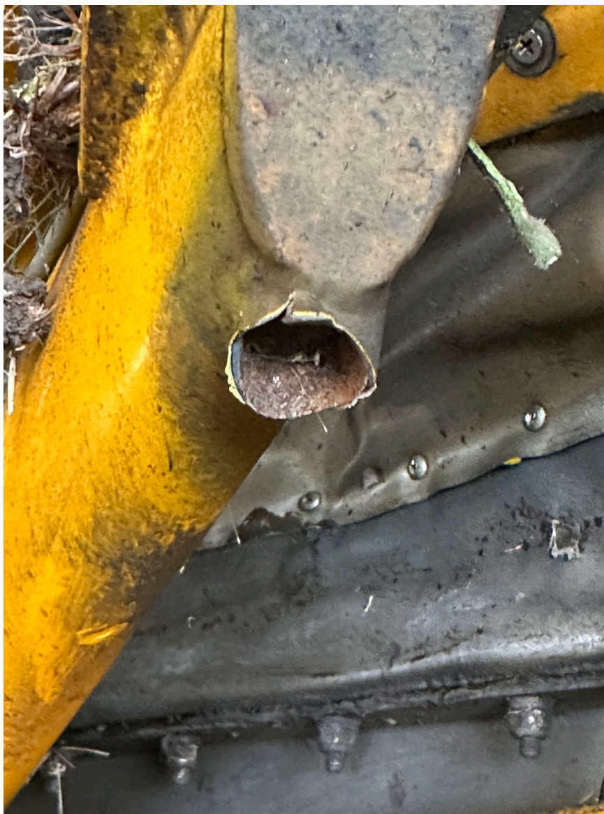
Photograph 4 - Broken structural tube (Courtesy of FAA)
