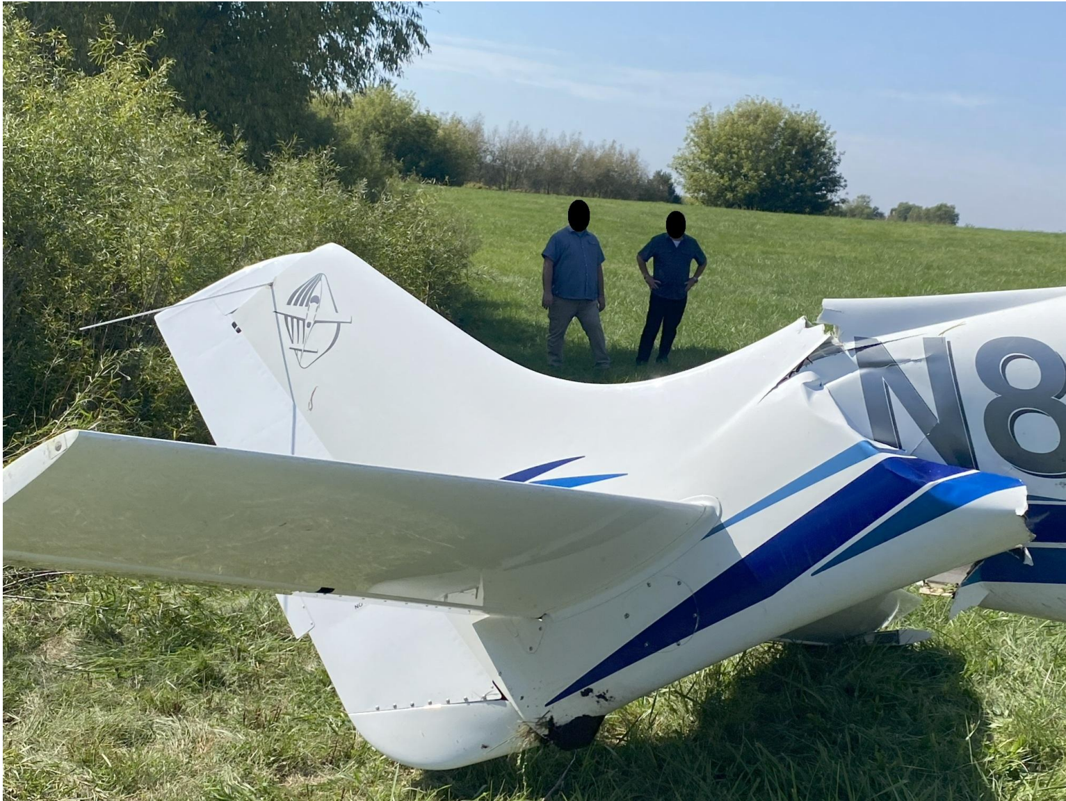
Photograph 3 - Airplane aft fuselage damage (Courtesy of Airplane Operator)
