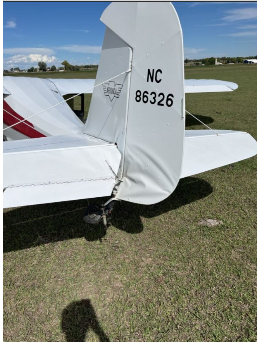
Photograph 1 - Substantial damage to rudder (Courtesy of FAA)
