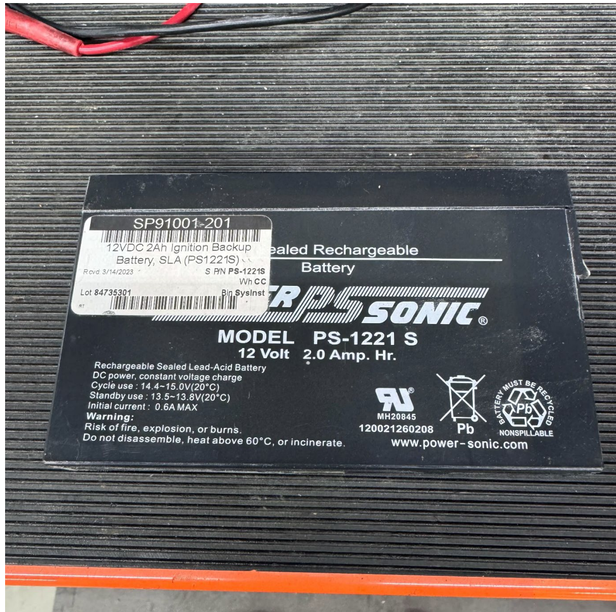
Photograph 8 - View of the backup ignition battery (courtesy of the pilot)
