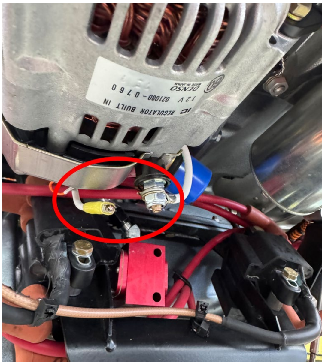
Photograph 6 - View of the broken ring terminal in the red circle (courtesy of the pilot)
