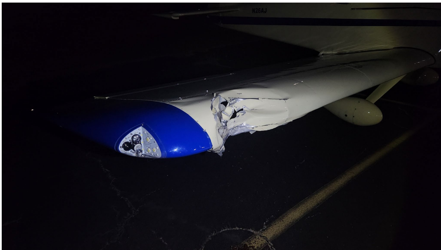
Photograph 3 - Right Wing Leading Edge Damage (Courtesy of Airport Manager)
