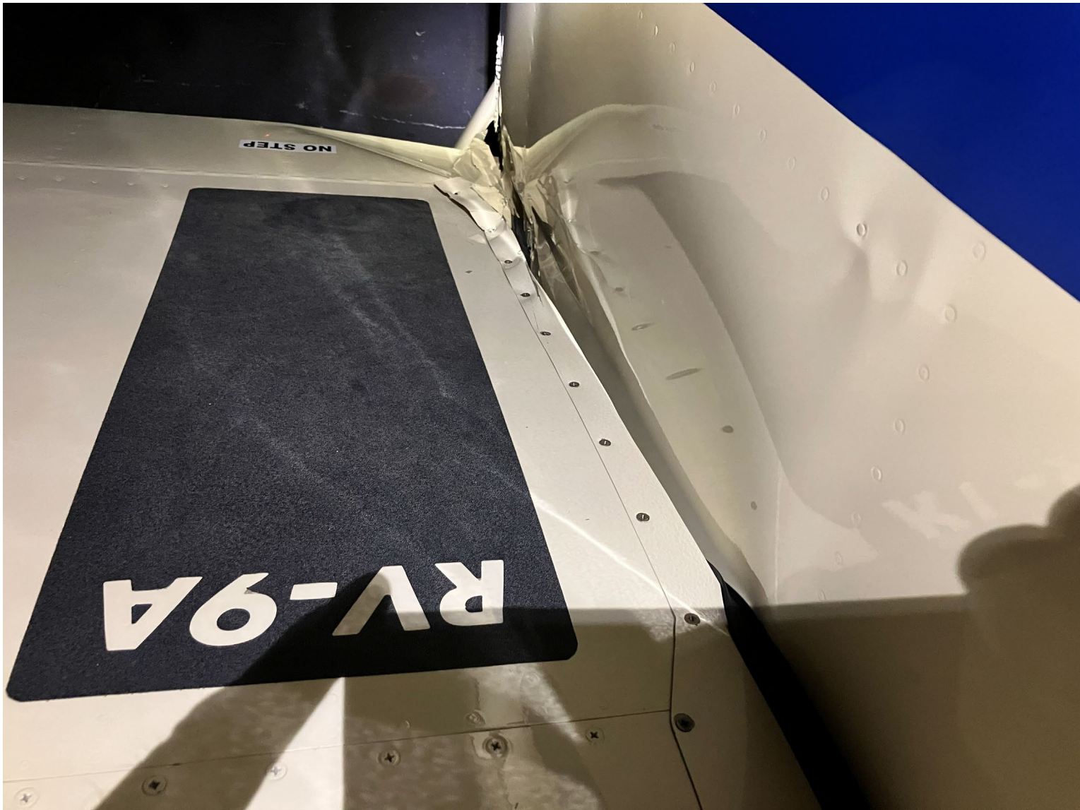
Photograph 2 - Right Wing Root Damage (Courtesy of Federal Aviation Administration)
