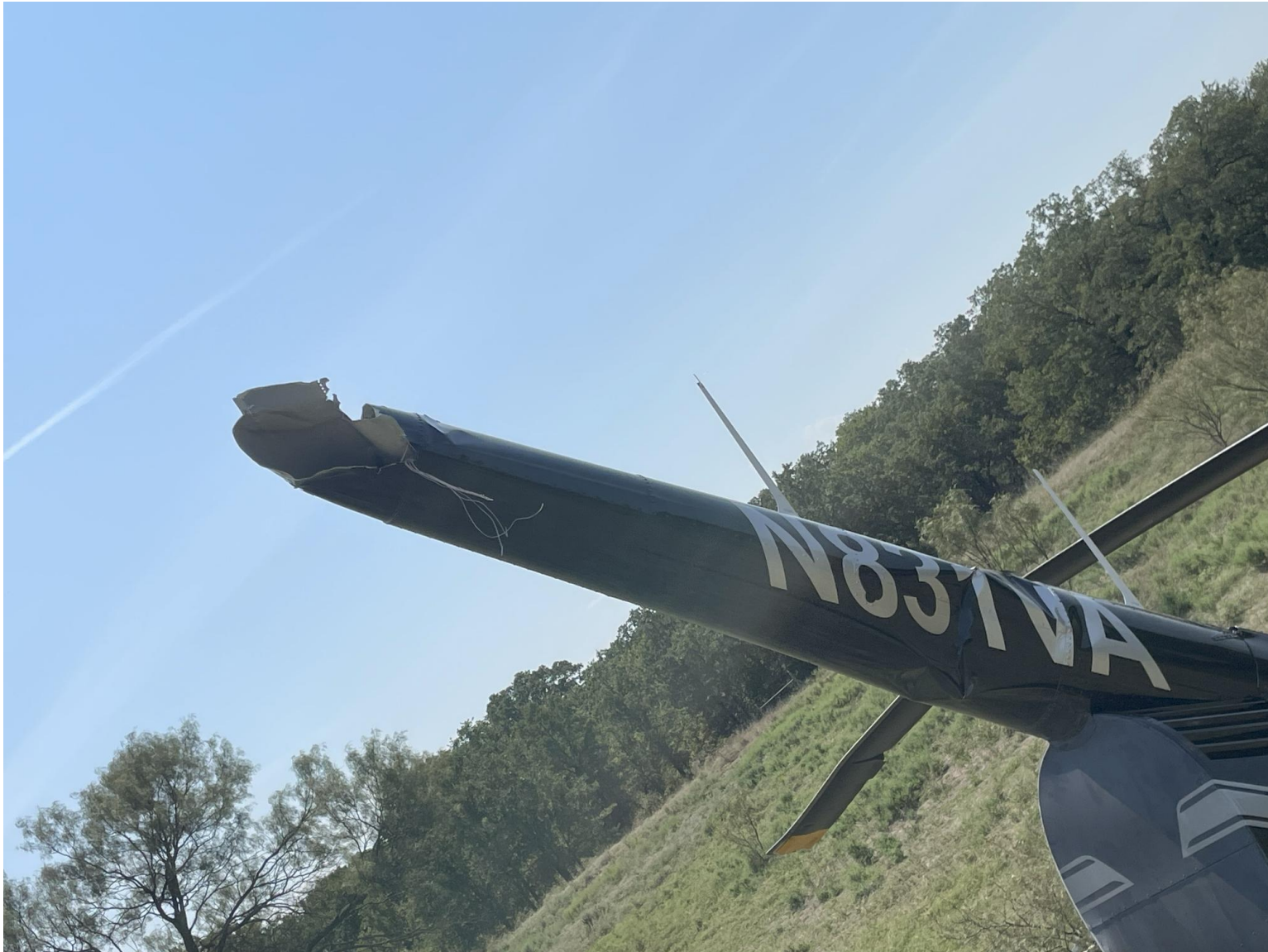
Photograph 3 - Tail boom (FAA photo)
