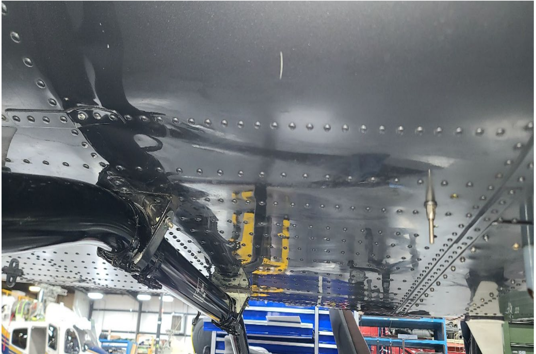
Photograph 7 - View of the substantial damage sustained to the rear right underside of the fuselage inside of a hangar (courtesy of Bell)
