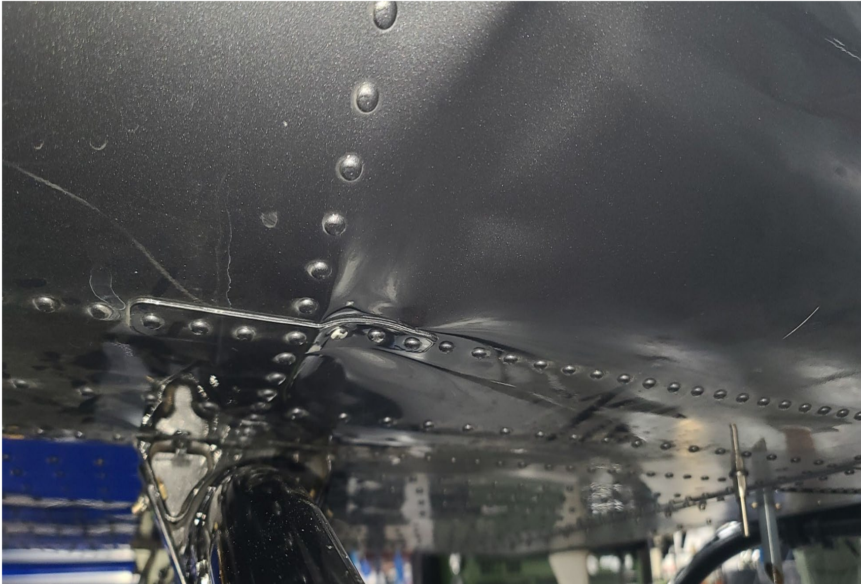
Photograph 6 - View of the substantial damage sustained to the front left underside of the fuselage inside of a hangar (courtesy of Bell)
