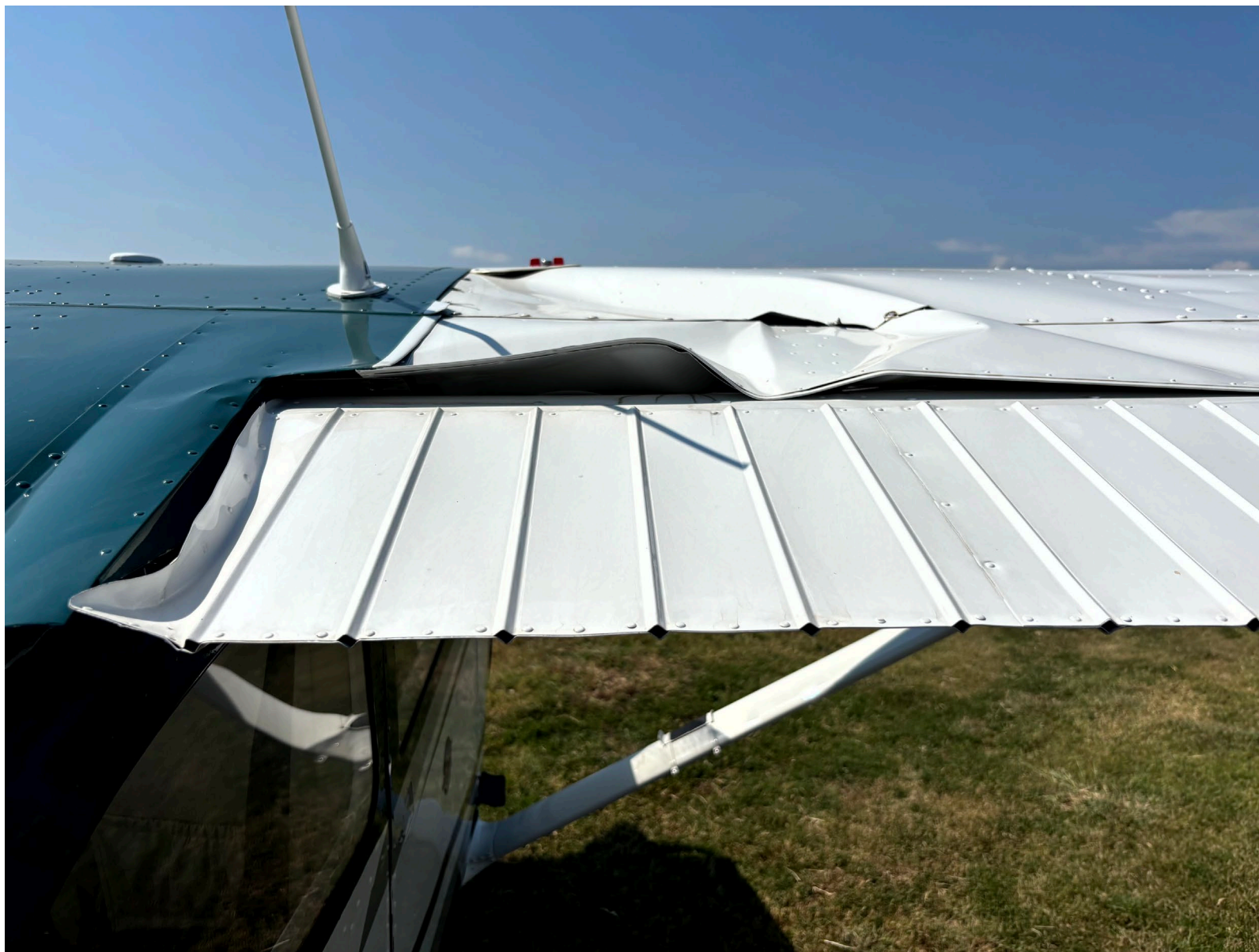
Photograph 4 - Aft right wing damage (Courtesy of FAA)
