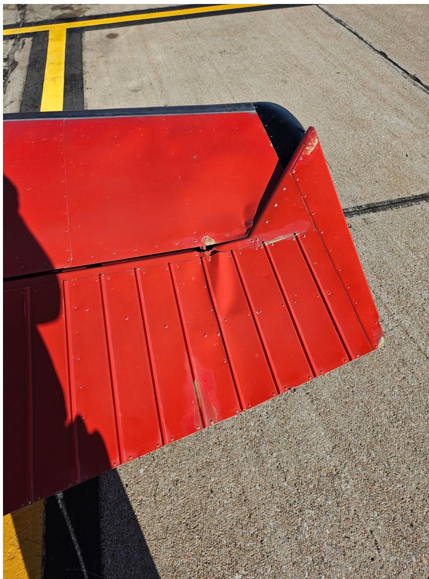
Photograph 2 - Right horizontal stabilizer and elevator after the accident (Courtesy of FAA)
