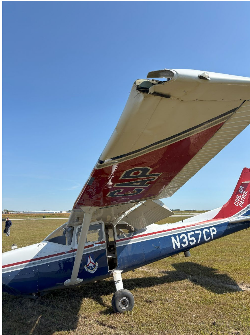
Photograph 4 - Left Wing Damage (Courtesy of Freeman Municipal Airport Manager)
