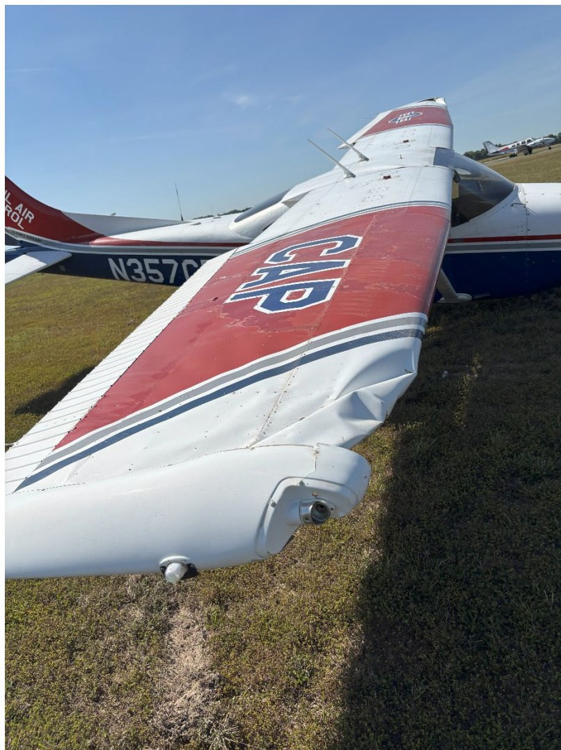
Photograph 2 - Right Wing Damage (Courtesy of Freeman Municipal Airport Manager)
