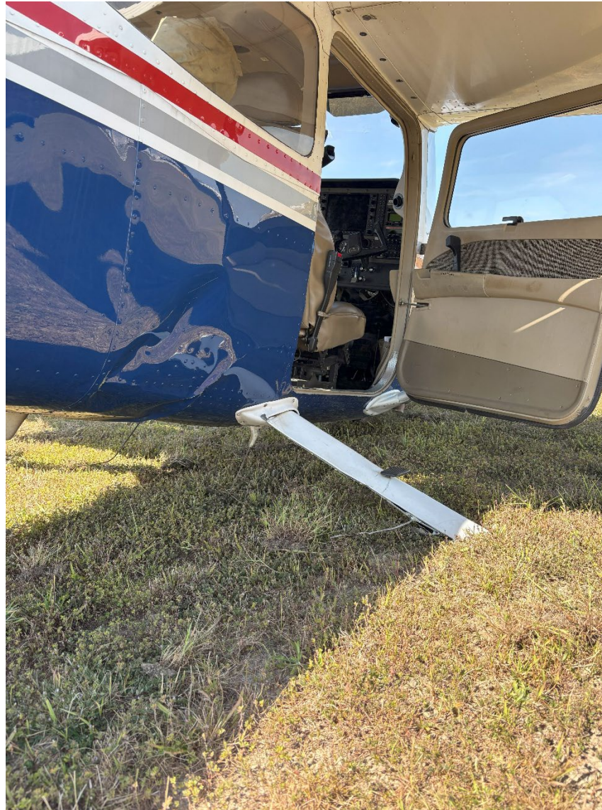
Photograph 3 - Right Fuselage Damage (Courtesy of Freeman Municipal Airport Manager)
